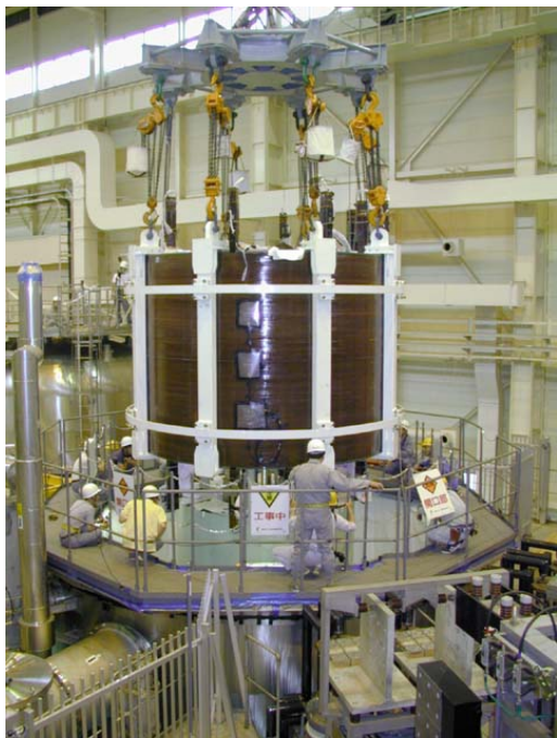
FIG. 5: Central Solenoid Model Coil Facility
