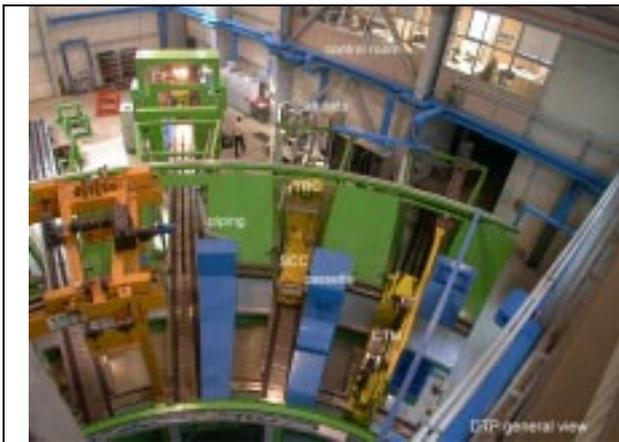
FIG. 2. Mock-up of the lower portion of the vacuum vessel in the DTP
