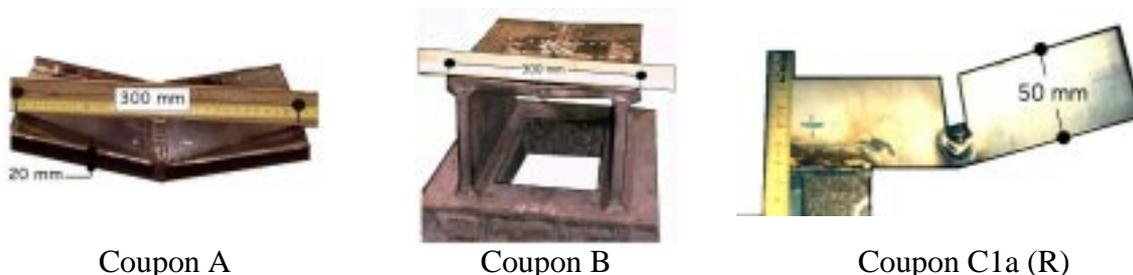
*FIG. 13. Coupons for Distortion Analysis (Manual TIG Welding - SAW)*
