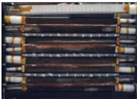
FIG. 5. Joints E-beam Welding
