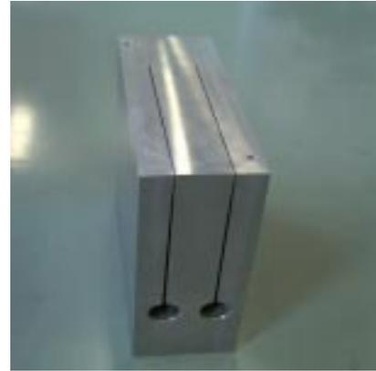
FIG. 2. Shield Block Slotting (JA HT)
