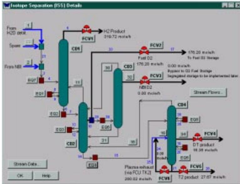
FIG. 2. ISS Detailed Model.
