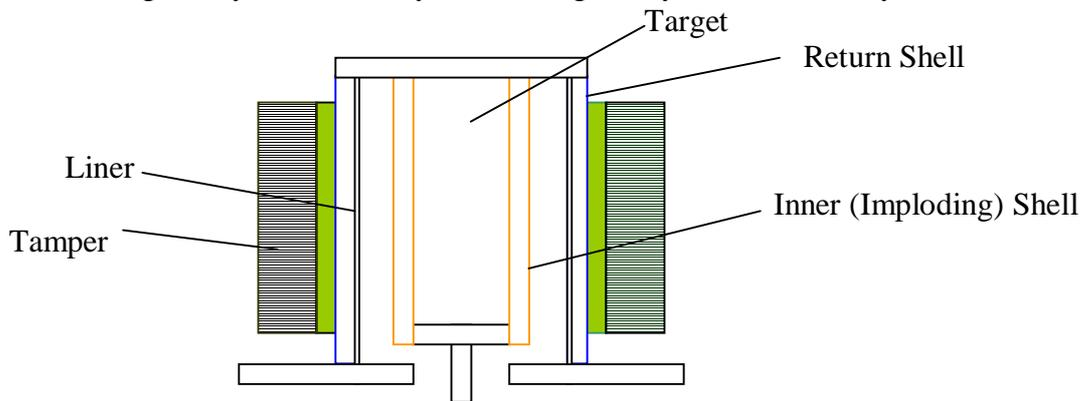
FIG.1. Schematic of the Assembly
