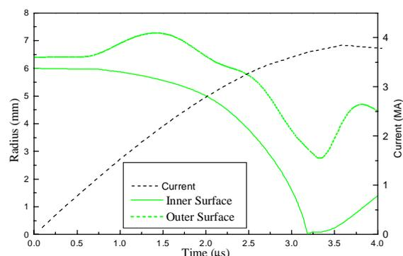
FIG. 3. Features of Liner Implosion on the 280 kJ Bank.
