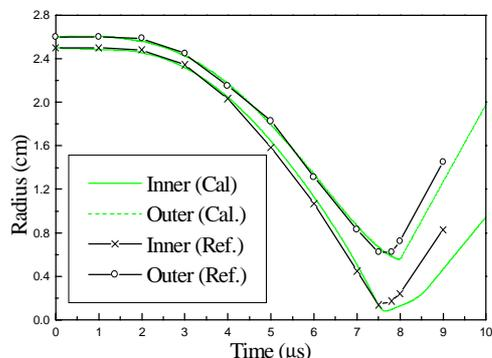
FIG. 2. Validation Result for Implosion of Thick Liner [Ref. 12].
