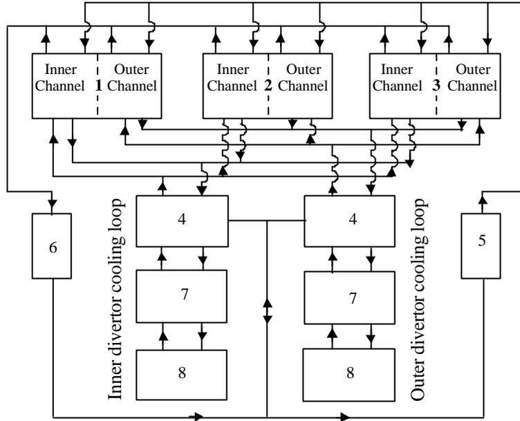
FIG. 2. Heat removing and conversion system scheme of lithium divertor sector 1, 2, 3 - divertor section; 4- lithium cooling channel and tritium recovery system , 5-lithium supply channel of CPS; 6- lithium output channel of CPS; 7-Na-K cooling loop; 8- conversion system.
