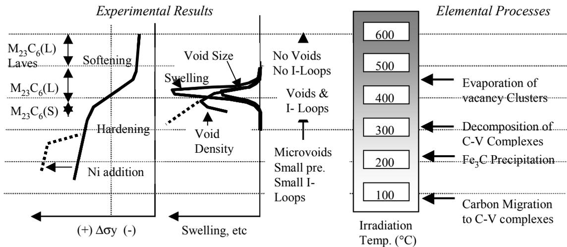
FIG.1. Material behavior-irradiation temperature diagram of RAFS
