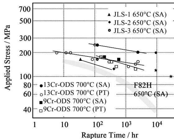
FIG.6. Improvement of the high temperature creep properties of RAF and ODS steels.
