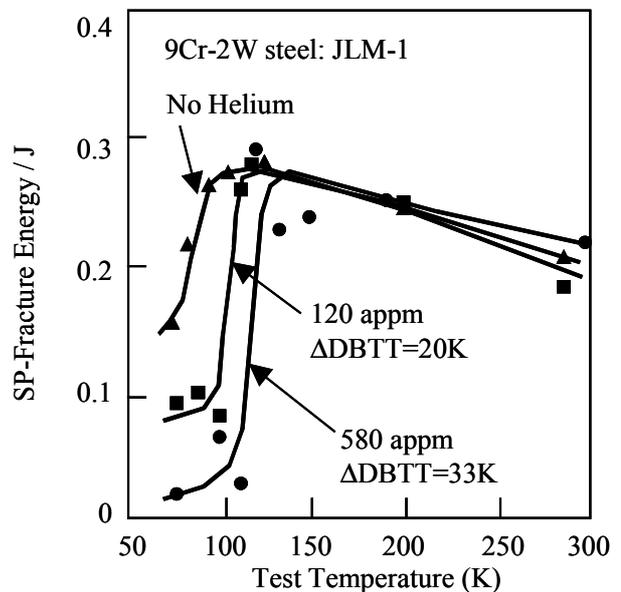
FIG.3. Effects of helium implantation on the ductile-brittle transition behavior of RAFS.
