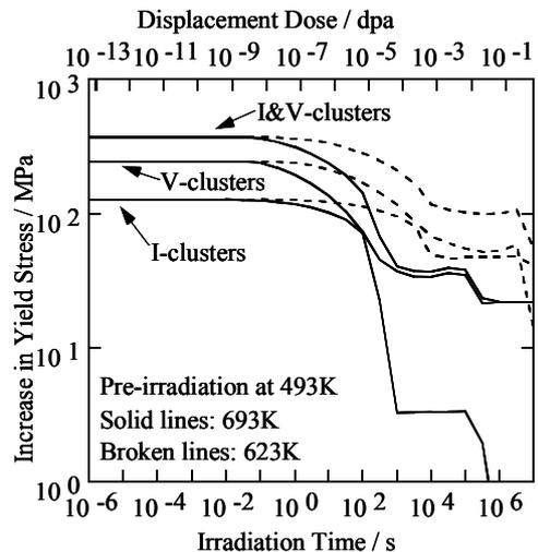
FIG.5. Results of computer simulation of irradiation behavior of RAFS under the varying temperature irradiation.
