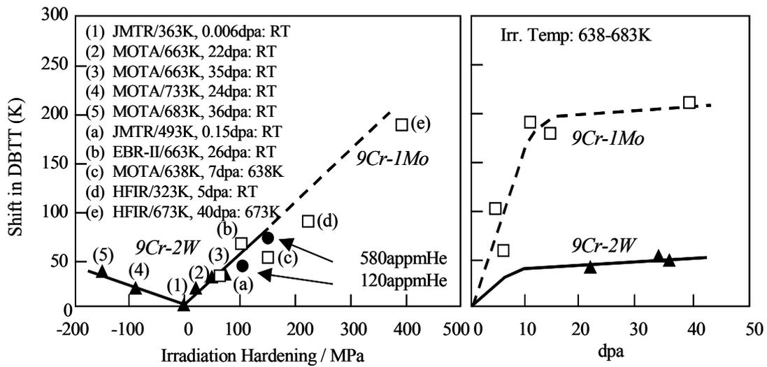
FIG.2. Effects of irradiation temperature on the shift in DBTT in ferritic steels.
