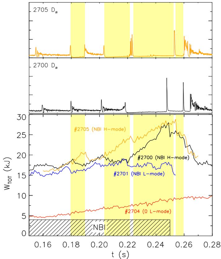
FIG. 4. Evolution of the plasma stored energy in discharge series 2700-2705. The benefit of injecting a modest  $\sim 0.5\text{MW}$  of NBI can clearly be seen, in particular for achieving L-H transition.
