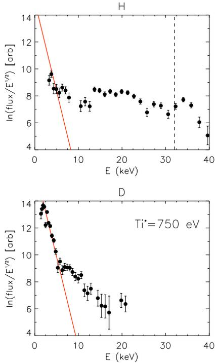
Figure 1 H and D neutral flux spectra recorded using the mid-plane mounted E||B NPA for shot 2932.
