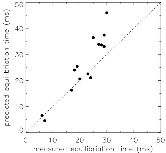
FIG. 5. Measured slowing down time against that for a uniform, steady state plasma.
