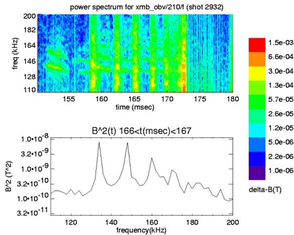
FIG. 6. Spectrogram for discharge 2932 showing at least 4 discrete modes (indicated by the time averaged plot of  $B^2(t)$  vs. frequency spectrum) persisting through a series of fishbone-like broad-band events.
