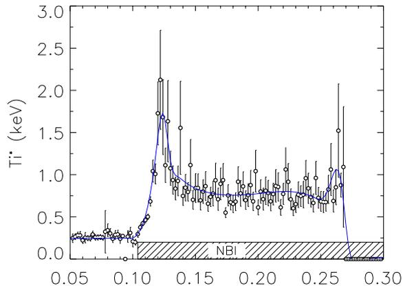
FIG. 3. Ion temperature recorded by the NPA throughout discharge 2932.
