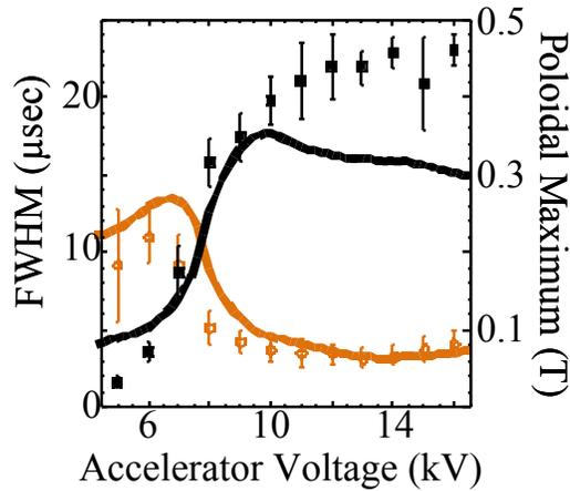
Figure 2. Comparison between experimental measurements and simulations of the compact toroid's poloidal magnetic field at 1.42 m. Simulations are denoted by gray and black lines while experimental measurements are denoted as gray circles and black squares for the FWHM and the field maximum, respectively.
