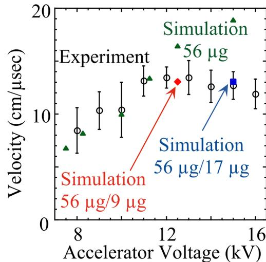
Figure 3. Comparison of the compact toroid's velocity between experiment and simulations. Simulations are represented by the diamond, square and triangles while the experimental mean is denoted by the black circles, respectively. The diamond and square represent a 56  $\mu\text{g}$  compact toroid accelerated through 9  $\mu\text{g}$  and 17  $\mu\text{g}$  of plasma uniformly distributed throughout the accelerator section, respectively.
