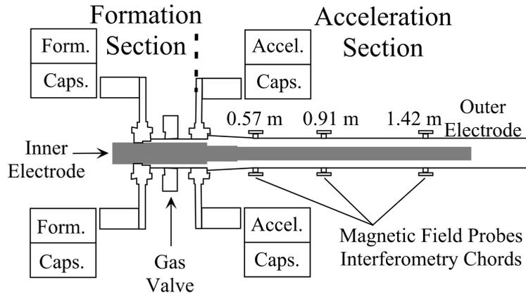
Figure 1. Schematic of the compact toroid injection experiment (CTIX). The compact toroid is accelerated between the inner and outer electrodes. Diagnostics placed at the three locations indicated measure the time-integrated magnetic field, line-integrated electron density and visible emission.
