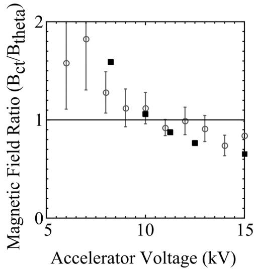
Figure 4. Comparison of the ratio of the compact toroid's internal magnetic field to the acceleration field between experiment and simulations. Simulations are represented by the solid black squares and experiments by the black circles.
