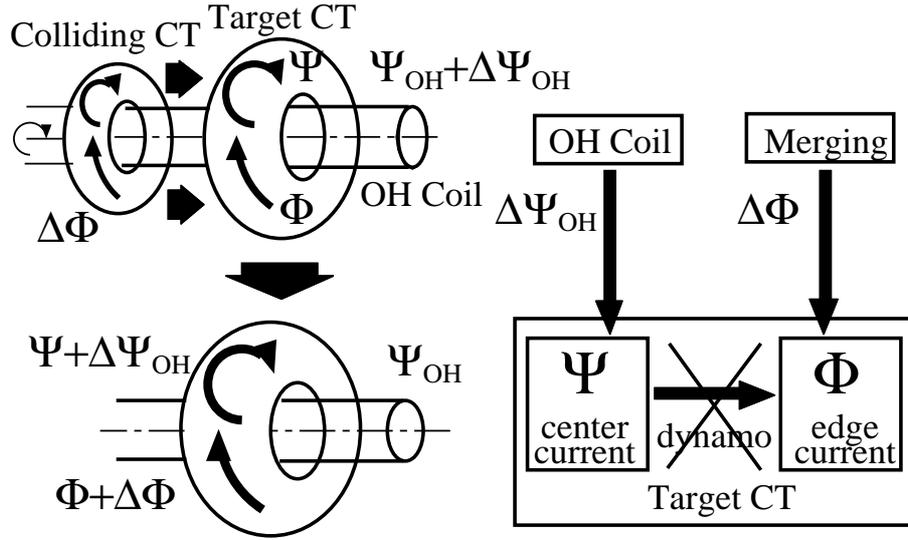
FIG. 1. Comparative study of CT stability under balanced current drive of merging / OH coil.
