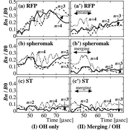
FIG. 6. Toroidal mode amplitudes of compact RFP(a), spheromak(b) and ST(c) under OH current drive and those under balanced current drive of merging / OH coil (a')-(c').
