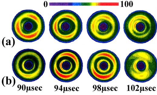
FIG. 5.  $H_{\beta}$  light emissivity of compact RFP (a) and spheromak (b) on the midplane.
