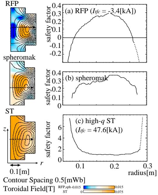
FIG. 3. Radial  $q$  profiles of compact RFP (a), spheromak (b) and ST (c) and their magnetic surfaces.
