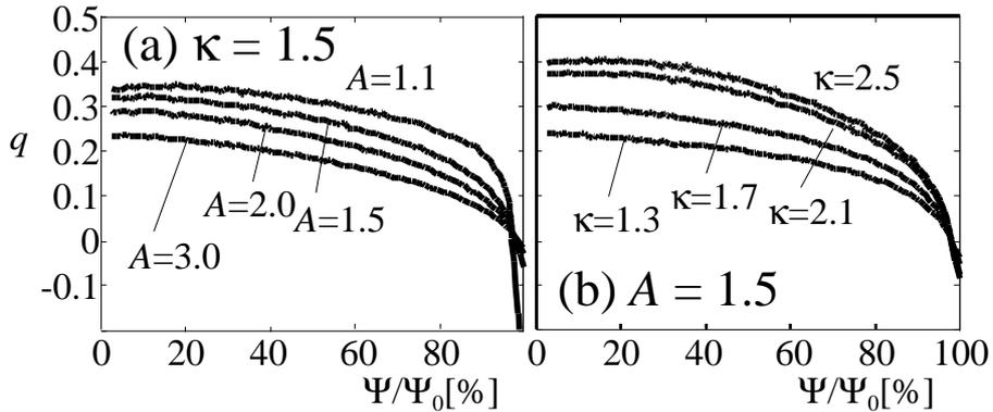
FIG. 4.  $q$ -profiles of compact RFPs with varied  $A$  and  $\kappa$ .
