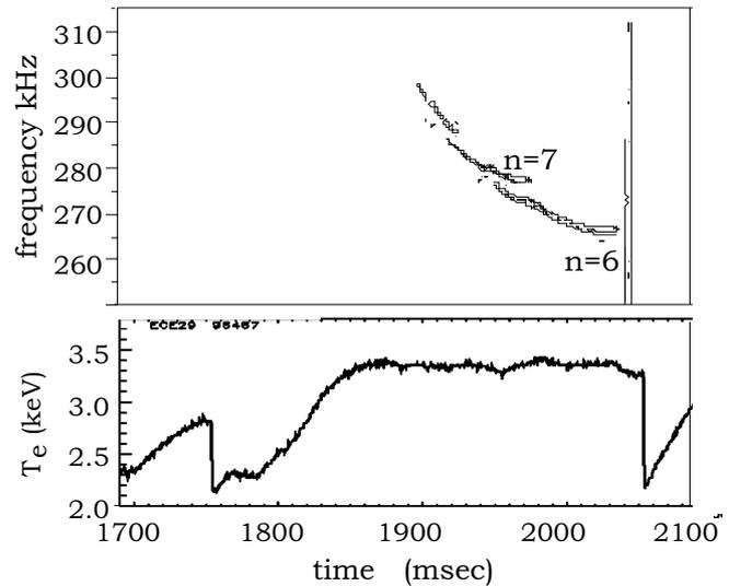
Fig. 1 Monster sawtooth with accompanying Alfvén instabilities in DIII-D. RF power of 1.2 MW is applied at  $t=1800$  msec.
