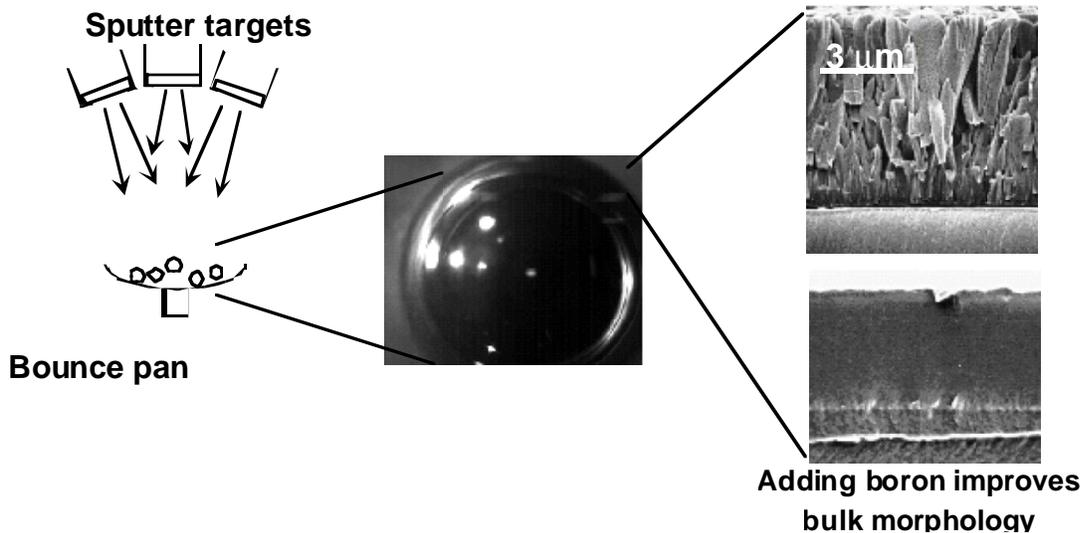
FIG. 10 Sputter deposition approach for fabricating beryllium ignition capsules.
