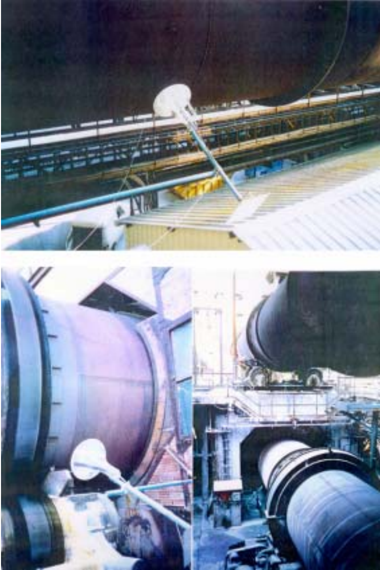
FIG. 33. Tracer test in a rotary kiln in the minerals industry. Heat protection of detectors.
