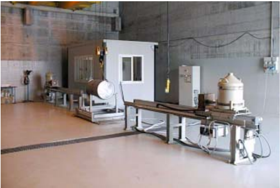
FIG. I-14. Drum radiological characterization at the Trino NPP.
