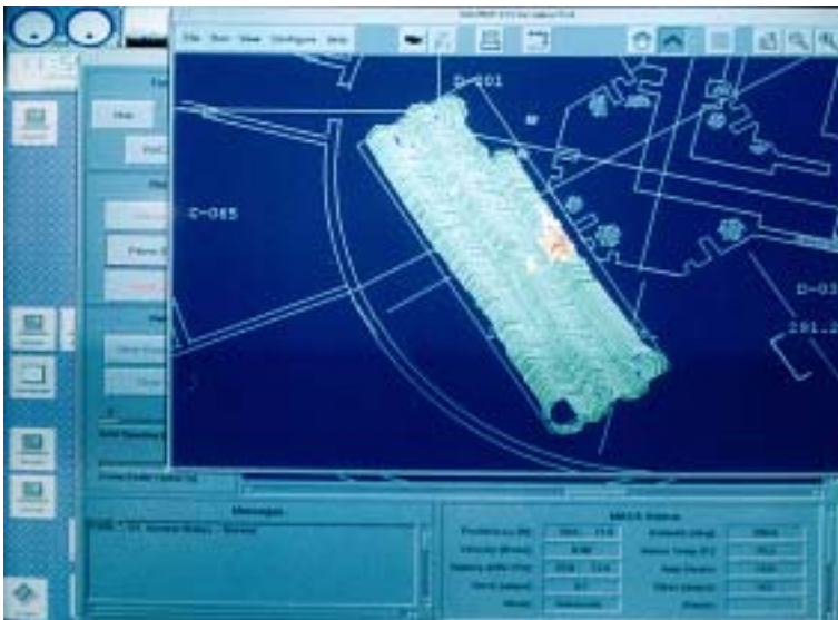
FIG. 9. Mobile automated characterization system (MACS) (CP-5 decommissioning project, Argonne National Laboratory, USA): graphic result of floor survey; yellow and red areas indicate contamination (Argonne National Laboratory).
