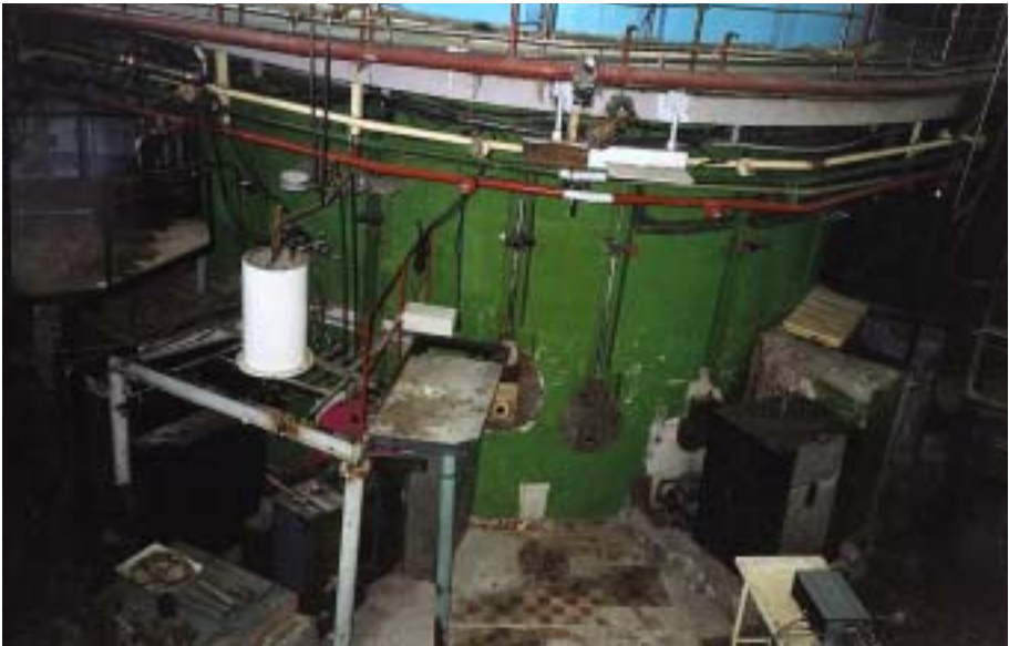
FIG. 12. The reactor block and experimental test apparatus of the IRT reactor, Georgia. At the end of operation, a research reactor's hall is typically full of experimental devices which are removed in preparation for decommissioning.
