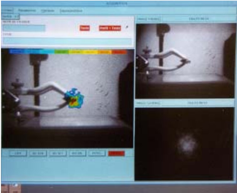
FIG. 8. ALADIN, France: a gamma camera to identify hot spots (red in the photo).
