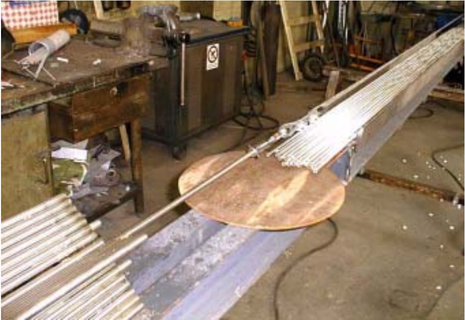
FIG. I-18. Disassembling of spare control rods at the Trino NPP to extract the Ag, In and Cd alloys.
