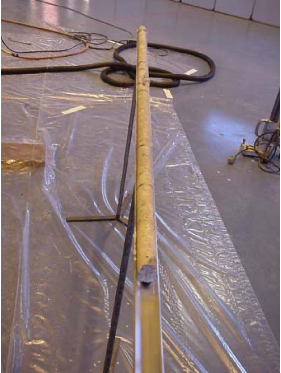
FIG. I-6. The borehole core resulting from drilling through the concrete shield of the DR-2 reactor, Denmark.
