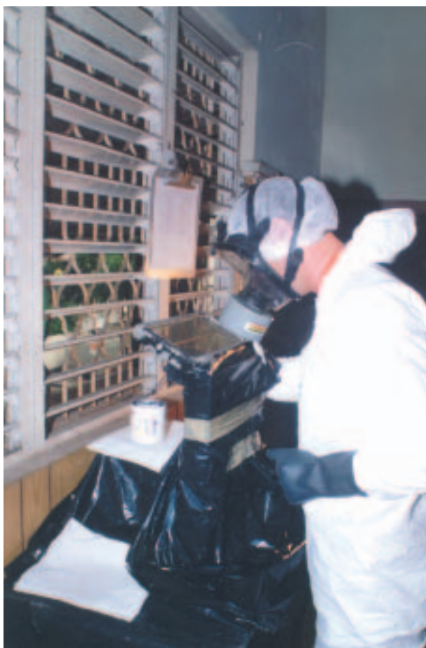
FIG. I.D-4. Conditioning the disused ^{226}\text{Ra} radiation sources into stainless steel capsules.
