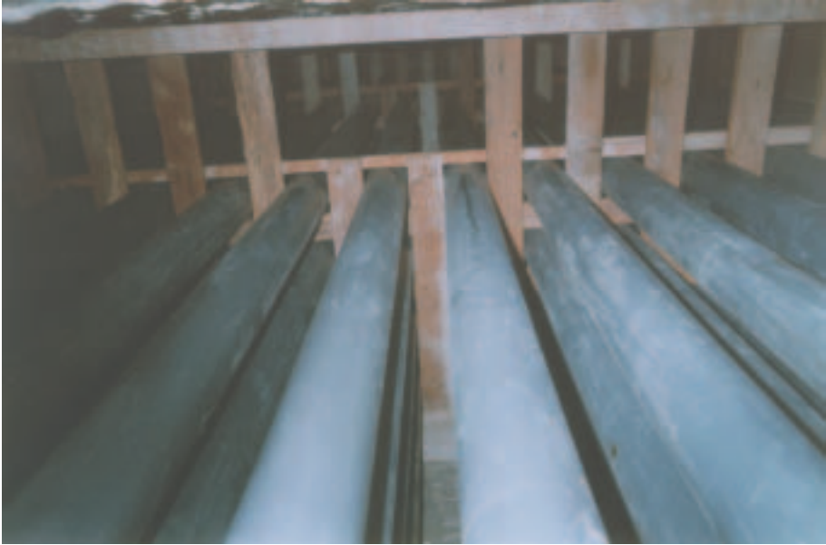
FIG. I.B-2. View of the well showing the pipe distribution. The length of the pipes was 10 m.
