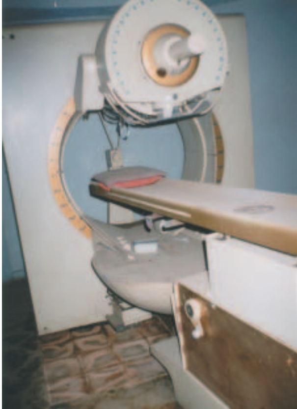
FIG. 3. A teletherapy unit being decommissioned.
