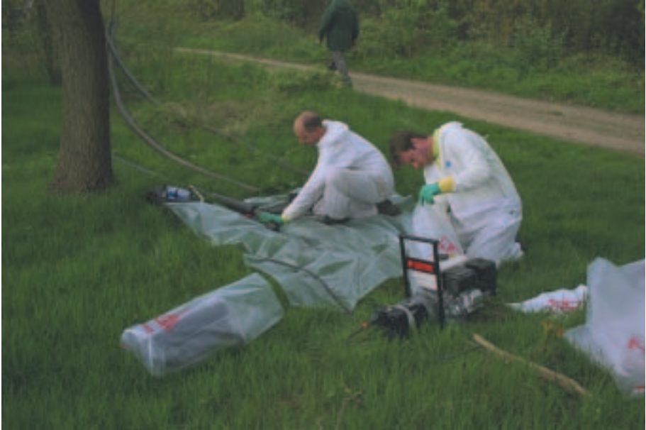
FIG. I.A-6. The segments are cut on the site and placed in plastic bags.
