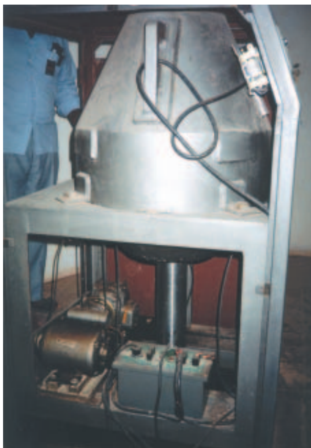
FIG. 4. A seed irradiator being decommissioned.
