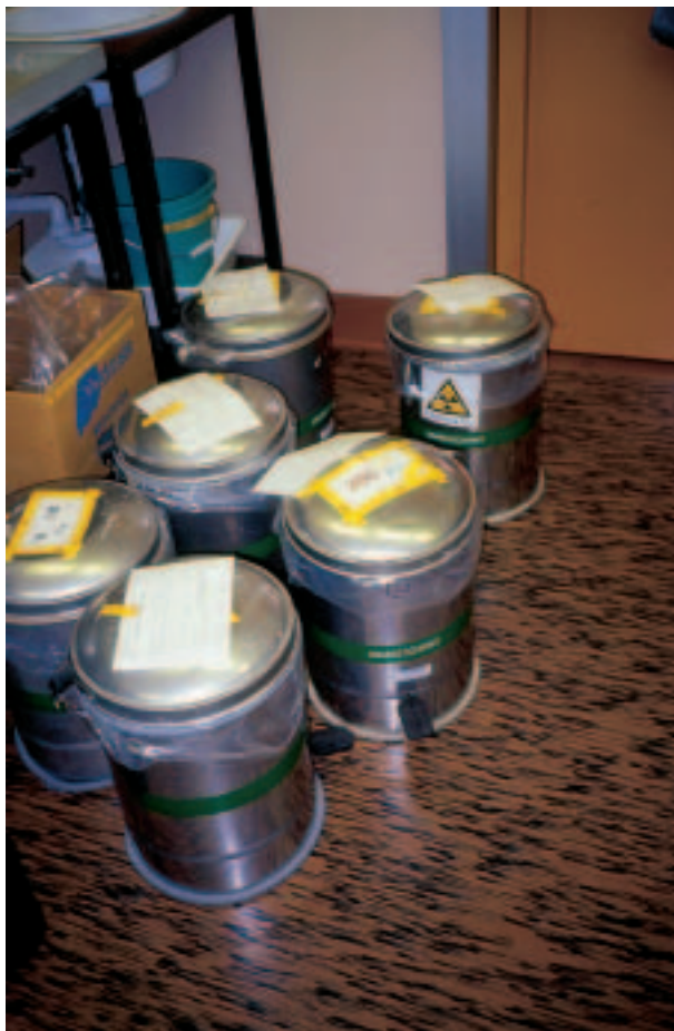
FIG. 2. Radioactive waste containers at a medical biological laboratory (courtesy of the Department of Pathophysiology, University of Vienna Medical School).
