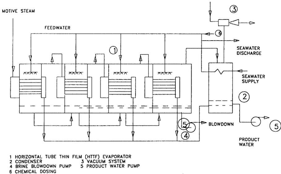
FIG. 4.2. Schematic flow diagram of the multiflect (MED) desalination process.
