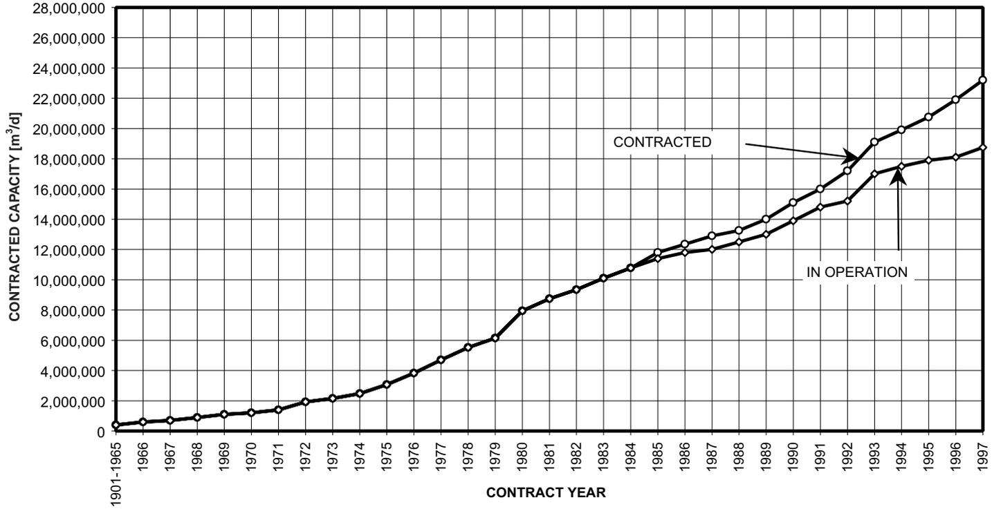
FIG. 2.3. Cumulative capacity of all land based desalting plants capable of producing 100 m<sup>3</sup>/d and per unit or more fresh water versus contract year.
