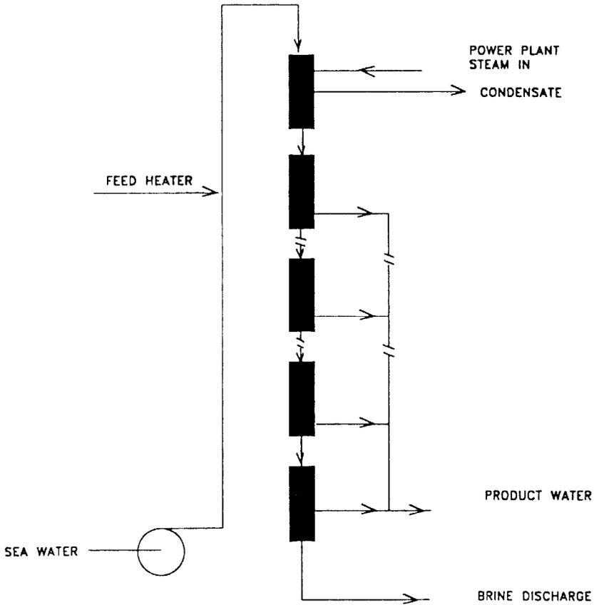
FIG. 4.7. Schematic process flow diagram of a stacked vertical tube evaporation plant.
