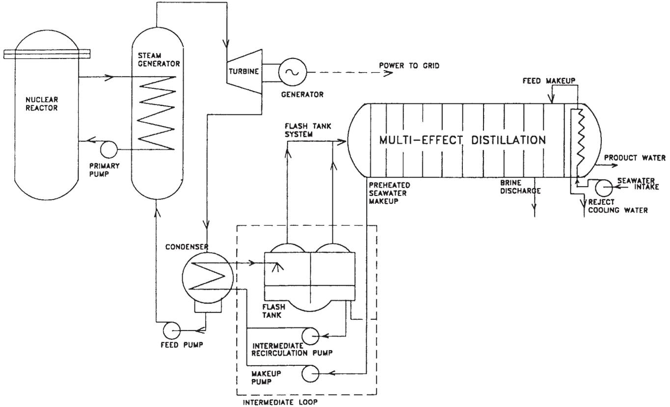
FIG. 5.5. Schematic diagram of a nuclear power reactor coupled to an MED plant.
