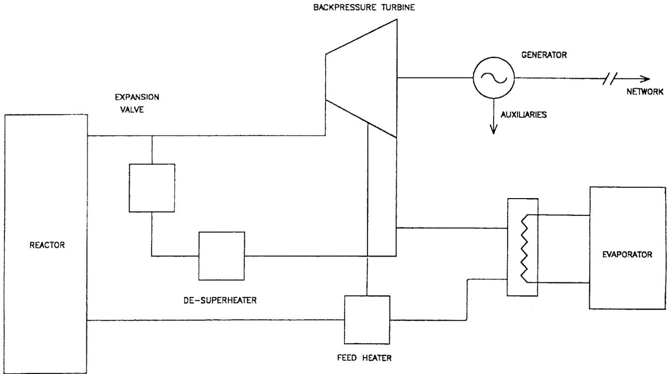
FIG. 6.1. Dual purpose plant backpressure cycle.
