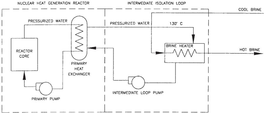
FIG. 5.2. Intermediate isolation loop between heating reactor and MSF plant.
