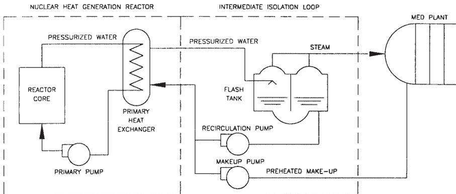
FIG. 5.3. Intermediate isolation loop between heating reactor and MED plant.
