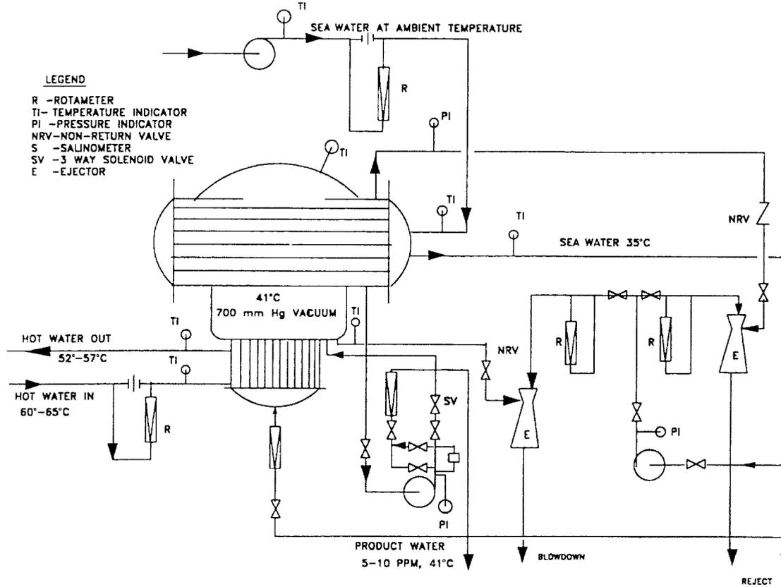
FIG. 4.6. Schematic flow diagram of a low temperature vacuum evaporation (LTE) desalination system.
