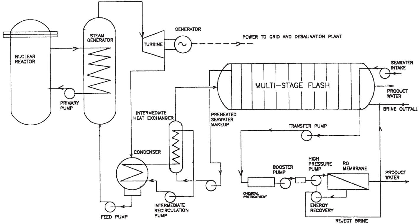
FIG. 5.6. Schematic diagram of a nuclear power reactor coupled to an MSF-RO plant.
