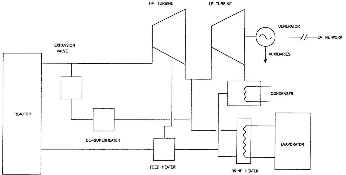
FIG. 6.2. Dual purpose plant extraction cycle.
