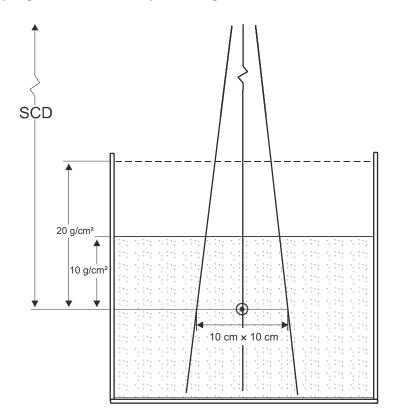
FIG. 6. Experimental set-up for the determination of the beam quality index Q (TPR<sub>20,10</sub>). The source-to-chamber distance (SCD) is kept constant at 100 cm and measurements are made with 10 g/cm<sup>2</sup> and 20 g/cm<sup>2</sup> of water over the chamber. The field size at the position of the reference point of the chamber is 10 cm × 10 cm. Either a cylindrical or a plane-parallel ionization chamber can be used.
