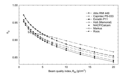
FIG. 8. Calculated  $k_Q$  values for electron beams, for various plane-parallel chamber types calibrated in  ${}^{60}$ Co gamma radiation.
