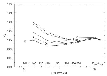
FIG. 11. Chamber to chamber variation in  $k_Q$  for seven ionization chambers, all of the type M23331. The values are normalized at <sup>60</sup>Co (data measured at PTB).
