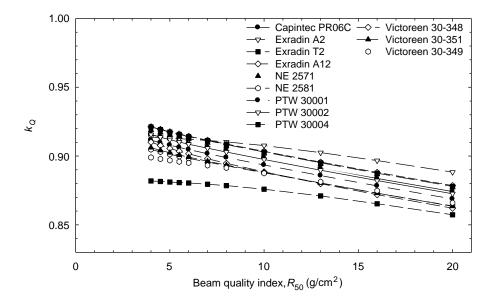
FIG. 9. Calculated  $k_Q$  values for electron beams, for various cylindrical chamber types calibrated in  ${}^{60}$ Co gamma radiation.
