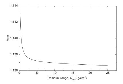
FIG. 21. Spencer–Attix ( $\Delta = 10 \text{ keV}$ ) stopping-power ratios, water to air, for clinical proton beams as a function of the beam quality index  $R_{res}$ . The curve is a fit to monoenergetic stopping-power ratios calculated by Medin and Andreo using the Monte Carlo code PETRA [151, 152]. The data include the transport of secondary electrons and nuclear inelastic processes, and the basic proton stopping powers are taken from ICRU Report 49 [118].
