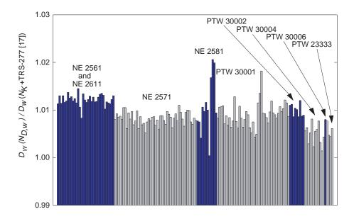
FIG. 19. The ratio of absorbed dose to water in  ${}^{60}$ Co determined with calibration factors in terms of absorbed dose to water,  $N_{D,w}$  and with calibration factors in terms of air kerma,  $N_{K}$  using the IAEA TRS-277 [17] Code of Practice for some of the ionization chamber types shown in Fig. 2. Both calibration factors are traceable to the BIPM. The differences are in most cases within the combined standard uncertainty of the two Codes of Practice based on  $N_{D,w}$  and  $N_{K}$
