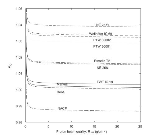
FIG. 15. Calculated values of  $k_Q$  for various cylindrical and plane-parallel ionization chambers commonly used for reference dosimetry, as a function of proton beam quality  $Q(R_{res})$  (data from Table 14).
