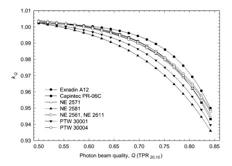
FIG. 7. Sigmoidal fits of calculated values of  $k_Q$  for various cylindrical ionization chambers commonly used for reference dosimetry, as a function of photon beam quality, Q (TPR<sub>20,10</sub>). Open symbols correspond to graphite walled ionization chambers, solid symbols to plastic walled chambers. Data from Table 14.
