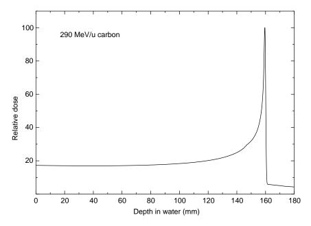
FIG. 16. Depth dose distribution of a monoenergetic 290 MeV/u carbon beam in water.
