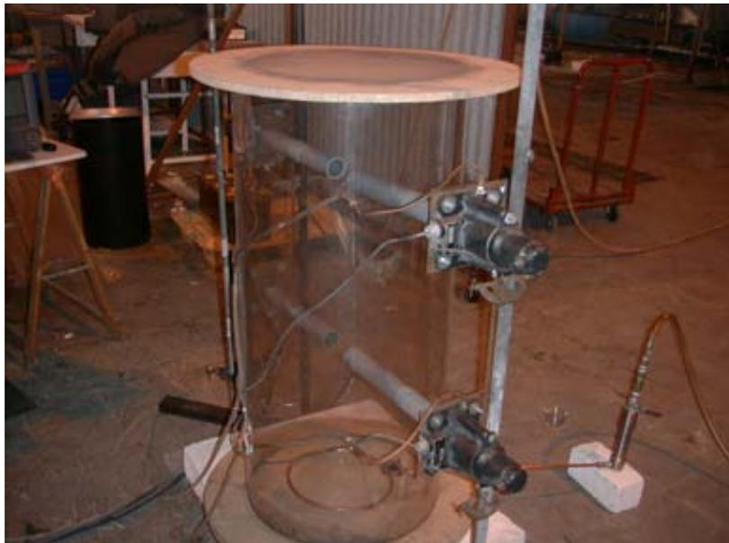
*FIG. 9. CNPP apparatus for the determination of the relationship between opacimeters and graphite dust concentration.*
