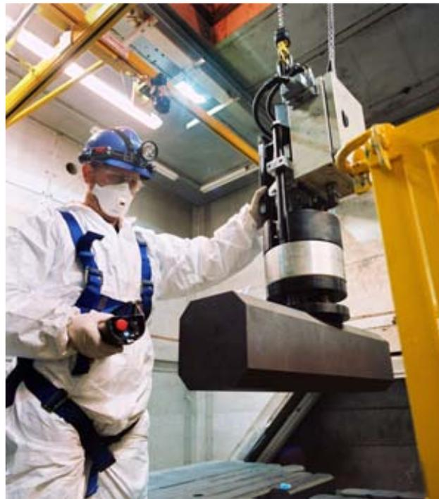
*FIG. 4. Graphite block handling.*
