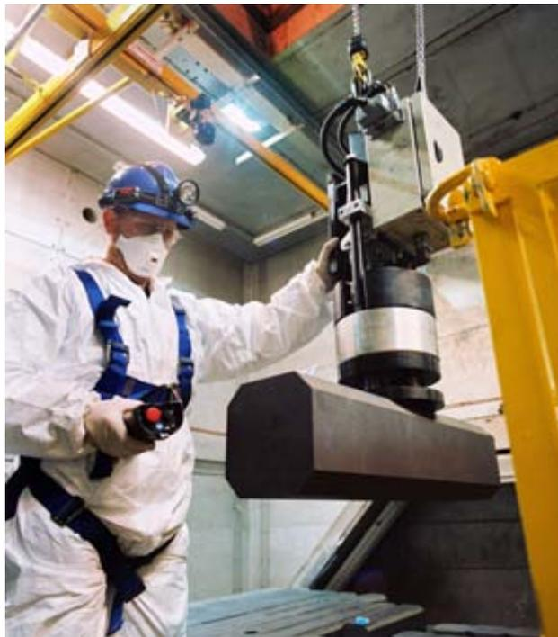
*FIG. 4. Graphite block handling.*
