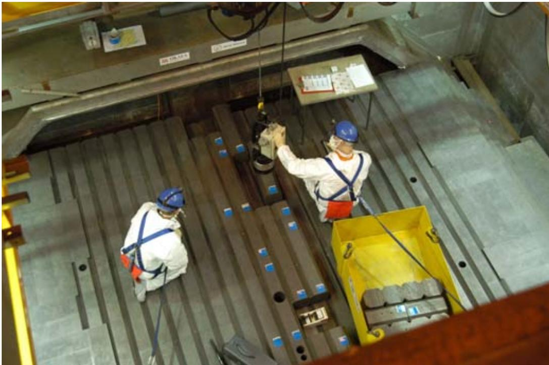
*FIG. 5. View of top access into reactor showing bin and top of core.*
