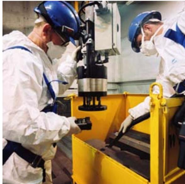
*FIG. 3. Drill and tap machine and collection of graphite sample.*
