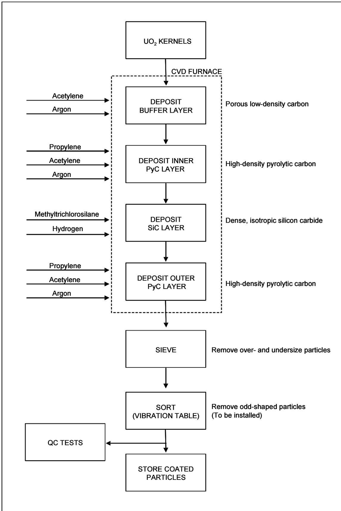
FIG. 2. Coating process.
