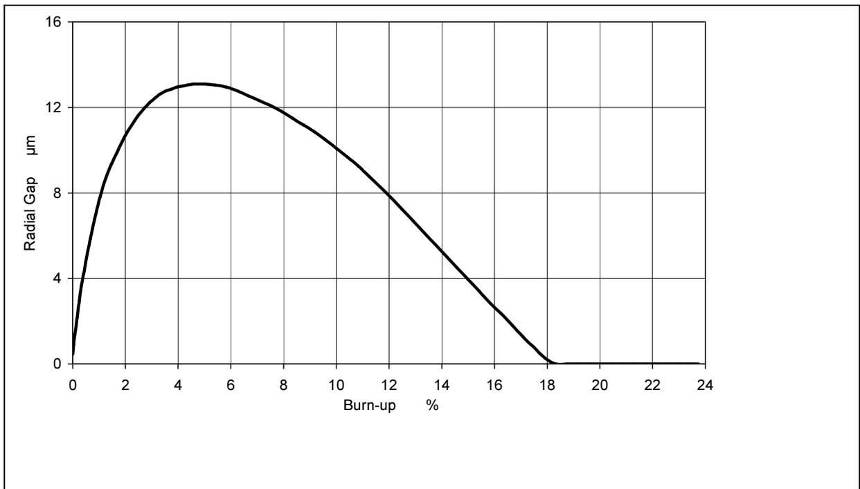
FIG. 5. Kernel-coating radial gap during irradiation.
