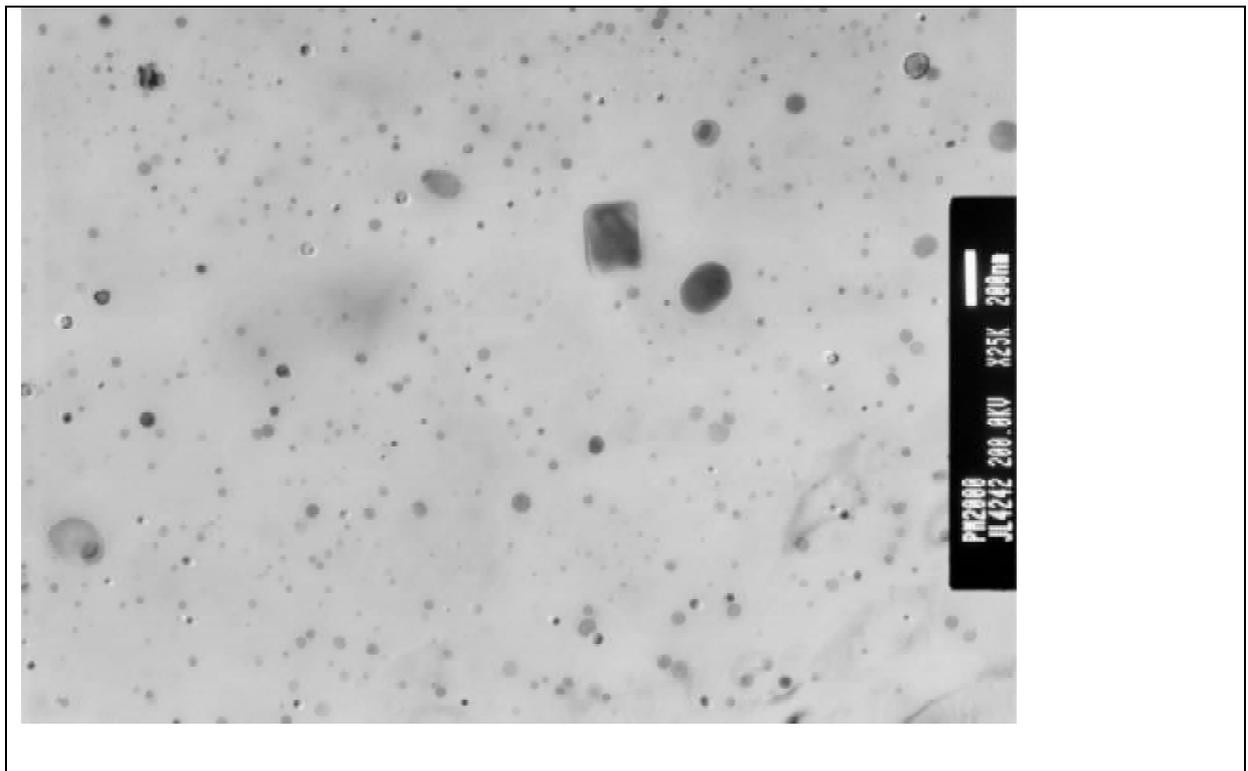
FIG. 1. Microstructure of a ferritic ODS alloy (TEM micrograph) ODS = oxide dispersion strengthened alloys.
