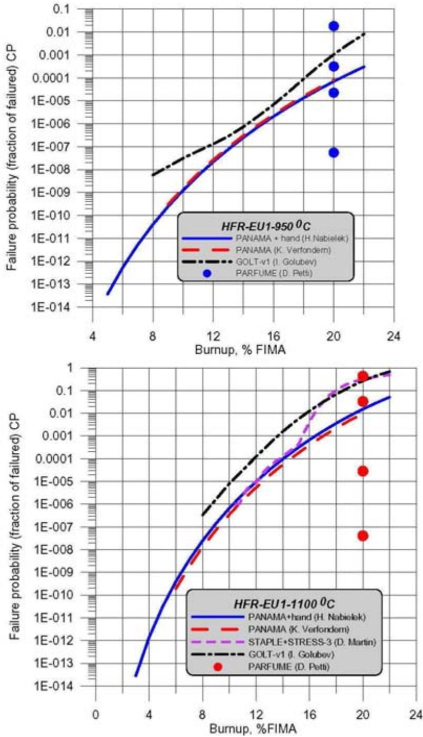
FIG. 1. Prediction of coated particle failure probability for HFR-EU1 irradiation test with different computer models.
