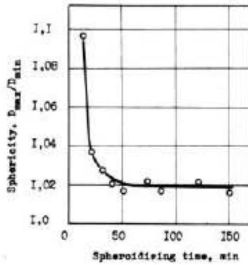
Fig.1 SP sphericity as a function of spheroidization time
