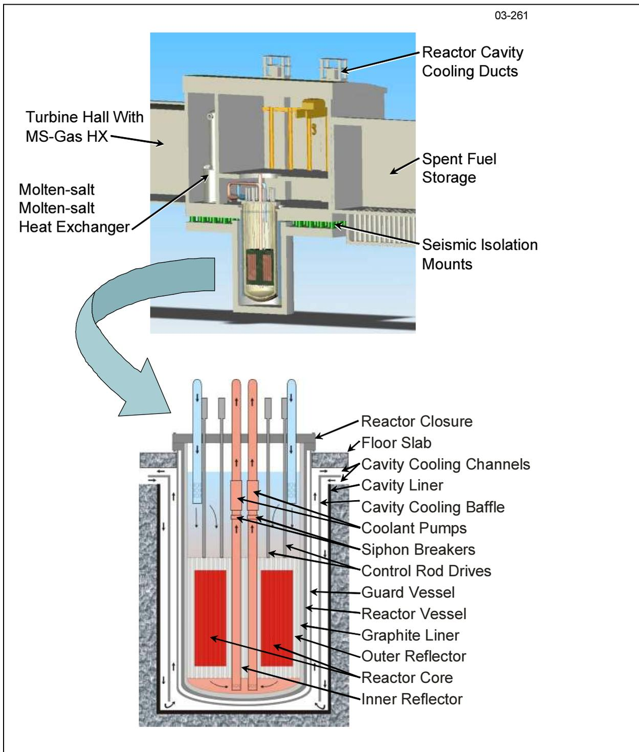
FIG. 2. Schematic of the AHTR nuclear island and vessel.
