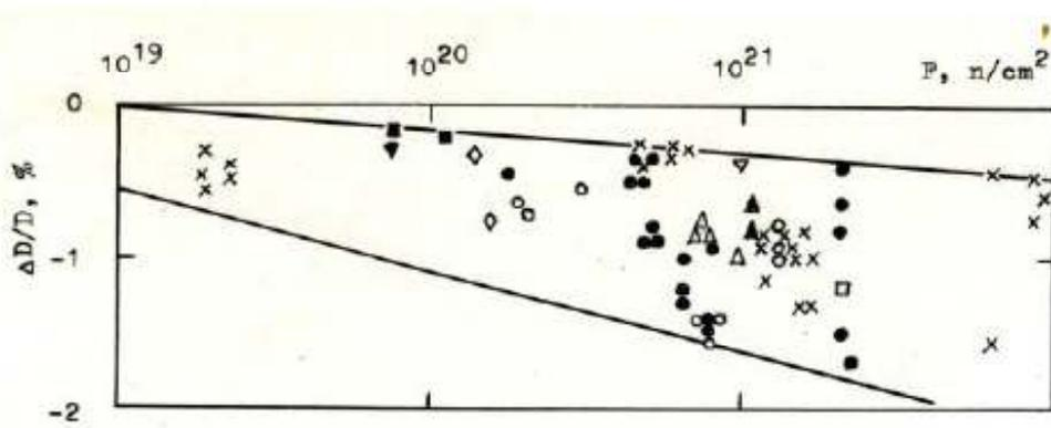
Fig.16. Dimension changes of absorbing (x) and fuel (the other points) elements versus the neutron fluence at irradiation temperatures of 400...1250 °C for absorbing elements and for fuel elements:
