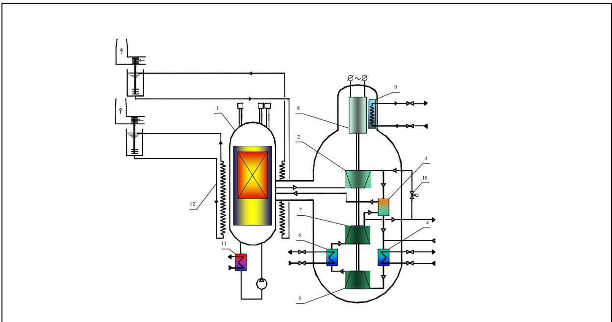
FIG. 2. The GT-MHR flow diagram: 1–reactor; 2–turbine; 3–recuperator; 4,6–pre-cooler and intercooler; 5,7–low-pressure and high-pressure compressor; 8–generator; 9–cooler; 10–bypass valve; 11–shutdown cooling system; 12–reactor cavity cooling system.
