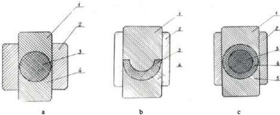
Fig. 5. Diagram of molding the billets of core, shell and fuel element in assembly:
