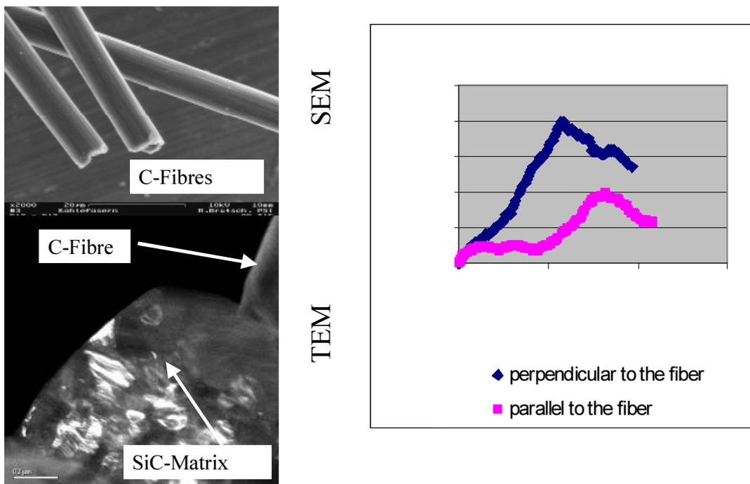
FIG. 2. Microstructure and results of punch test in different orientation of a SiC/C fibre reinforced ceramic.
