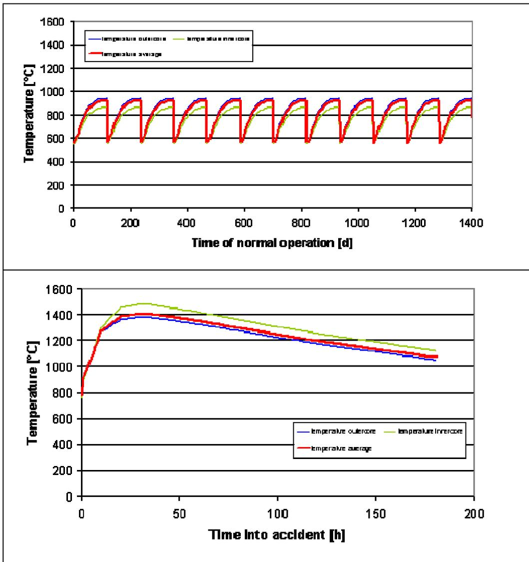
FIG. 2. Fuel temperatures during normal operation (top) and accident conditions.
