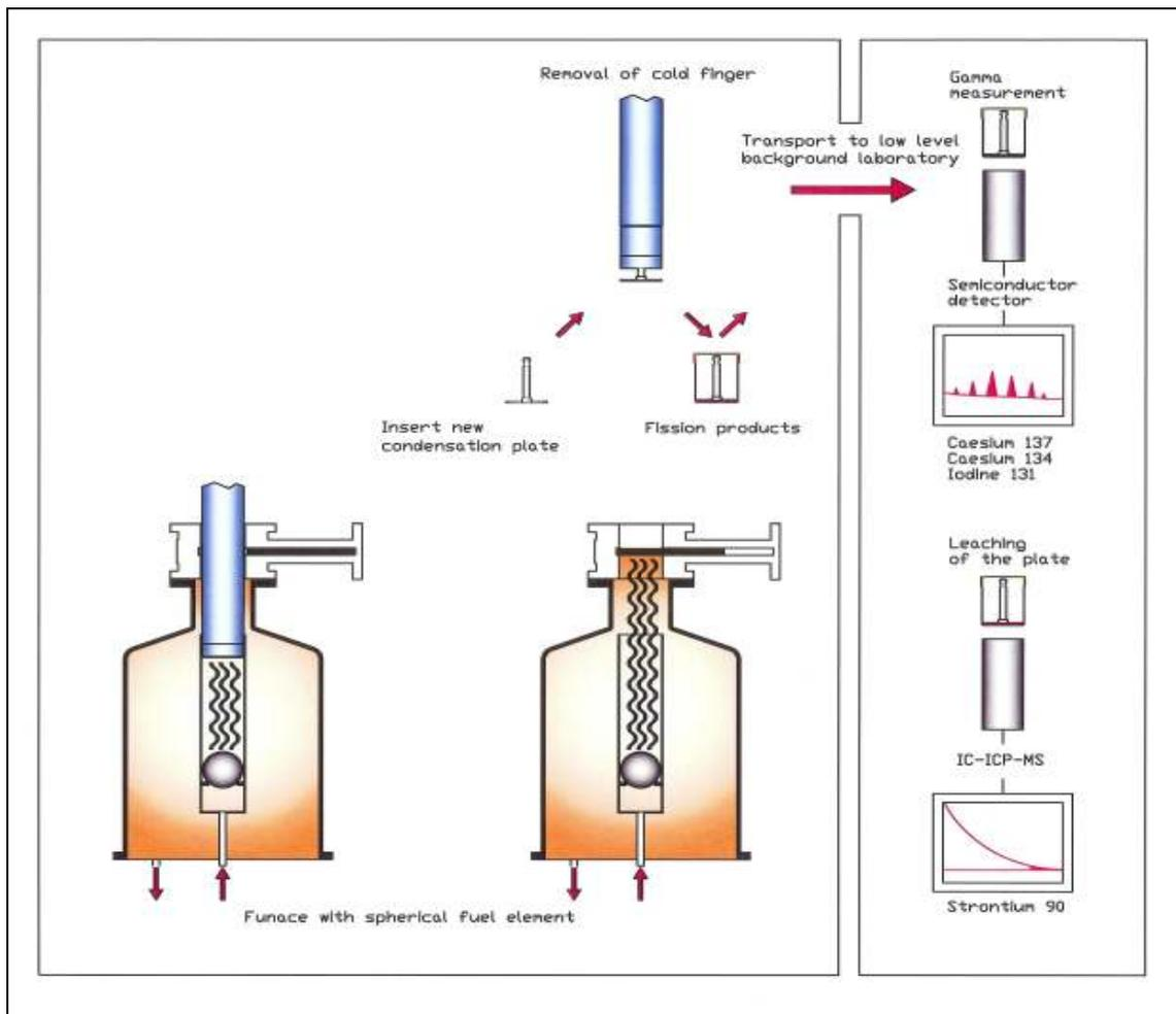
FIG. 3. Schema of the solid fission products measurement.
