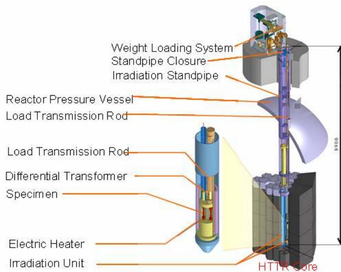
FIG. 9. Schematic view of irradiation capsule for the HTTR.
