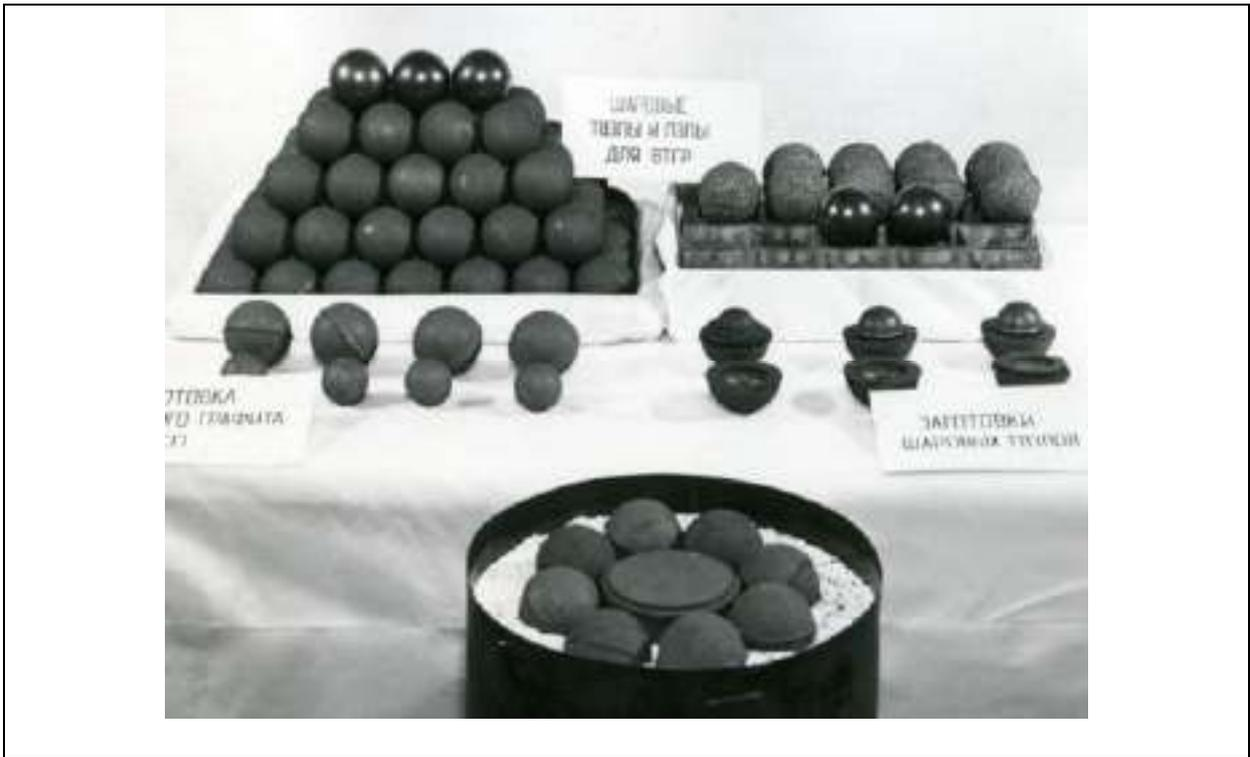
*Fig. 6. Spherical fuel and absorber elements.*
