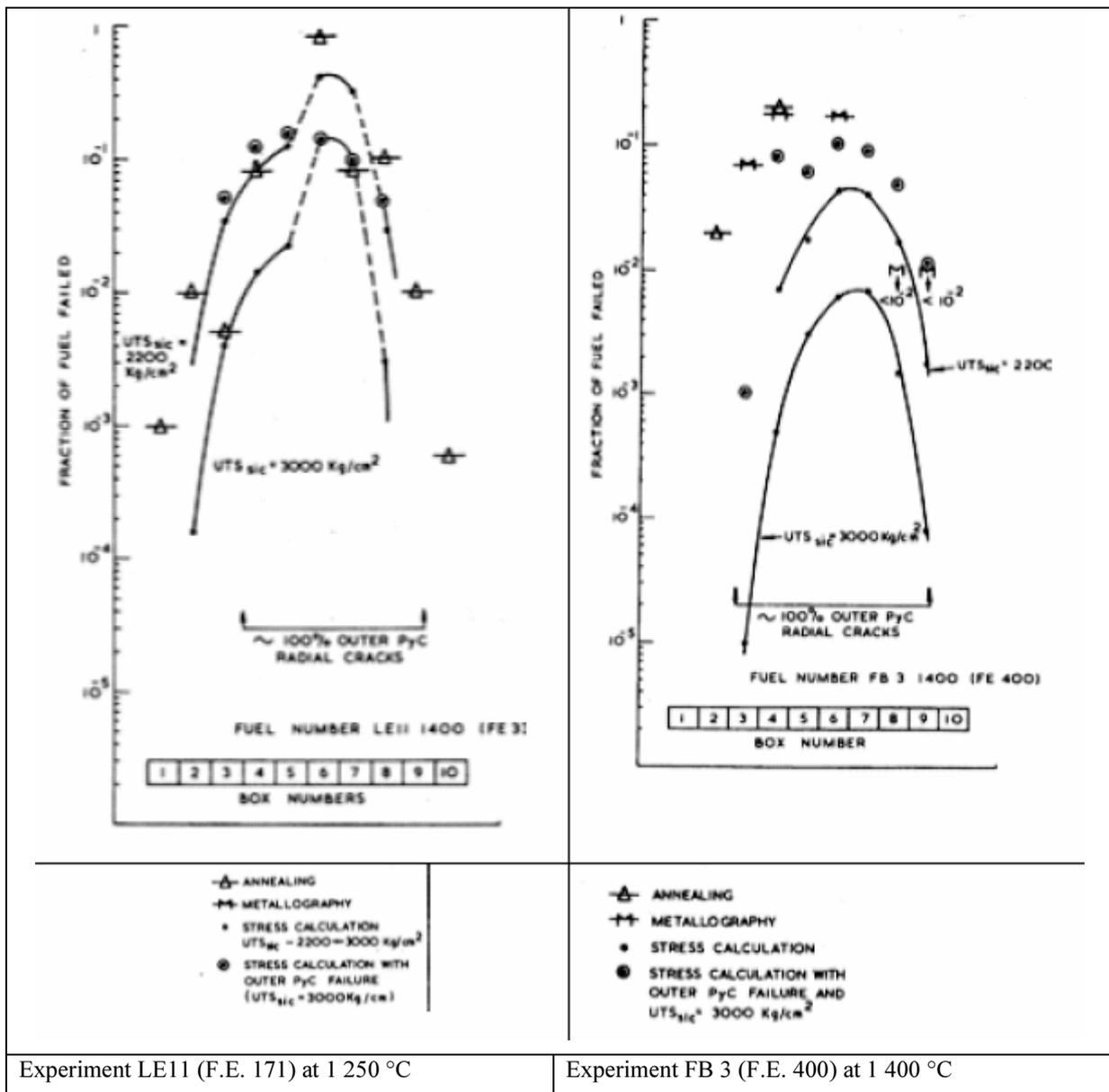
FIG. 5. Observed and postcalculated failure levels in Dragon charge III LE centre rod experiment series. The original STRESS code had no statistical options, but empirical correlations were used. Assumed median SiC strength was 220 or 300 MPa [11,21].
