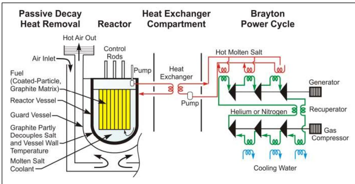
FIG. 1. Schematic of the AHTR for electricity production.
