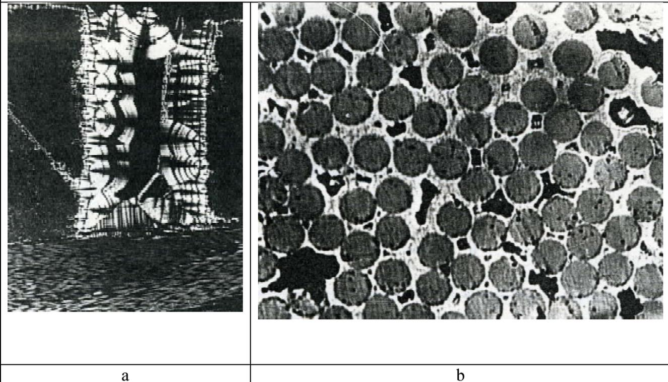
*Fig. 13. Macrostructure (a- x50) and microstructure (b- x1000) of carbon-carbon composites with a PyC matrix.*
