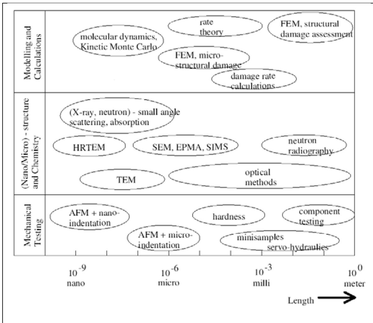
FIG. 4. Scheme of a multiscale approach for damage analysis. The line separates conventional (right) and advanced (left) techniques, modified after [6], (finite element (FM), (high resolution) transmission electron microscope (HR)TEM, atomic force microscope (AFM), scanning electron microscope (SEM), electron probe micro analysis (EPMA), secondary ion mass spectroscopy (SIMS).
