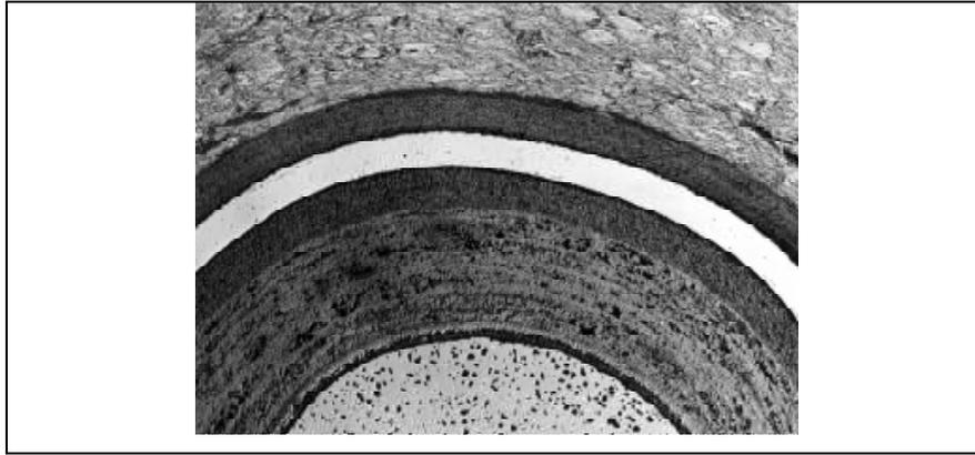
FIG. 8. Photomicrograph of German AVR fuel after irradiation.
