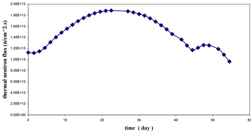
FIG. 1. Steady state flux distribution for one pass of the MEDUL cycle.
