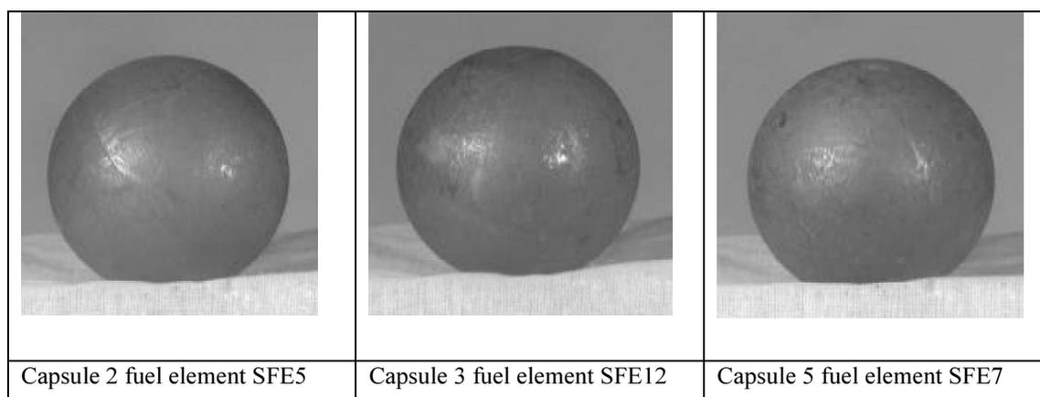
*FIG. 2. Appearance of irradiated spherical fuel elements.*
