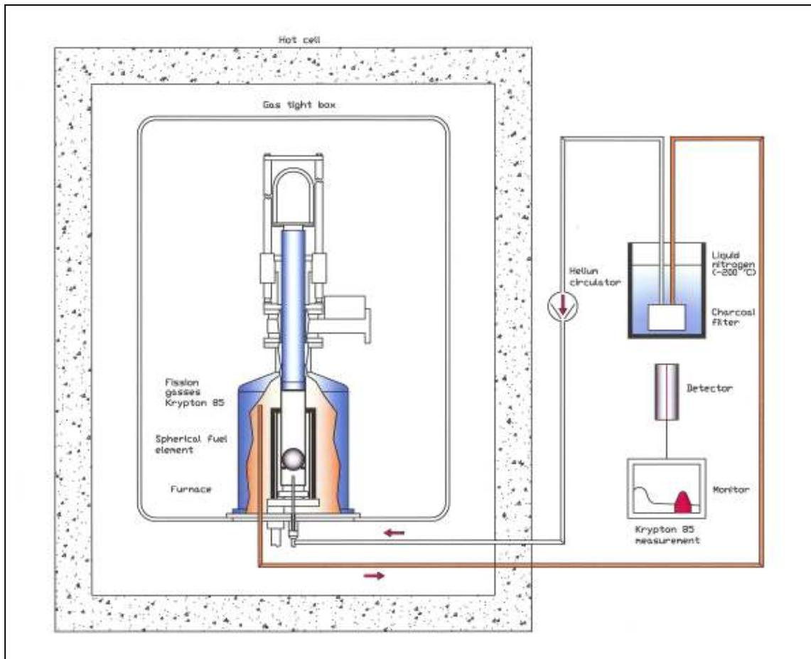
FIG. 2. Scheme of fission gas release measurement.
