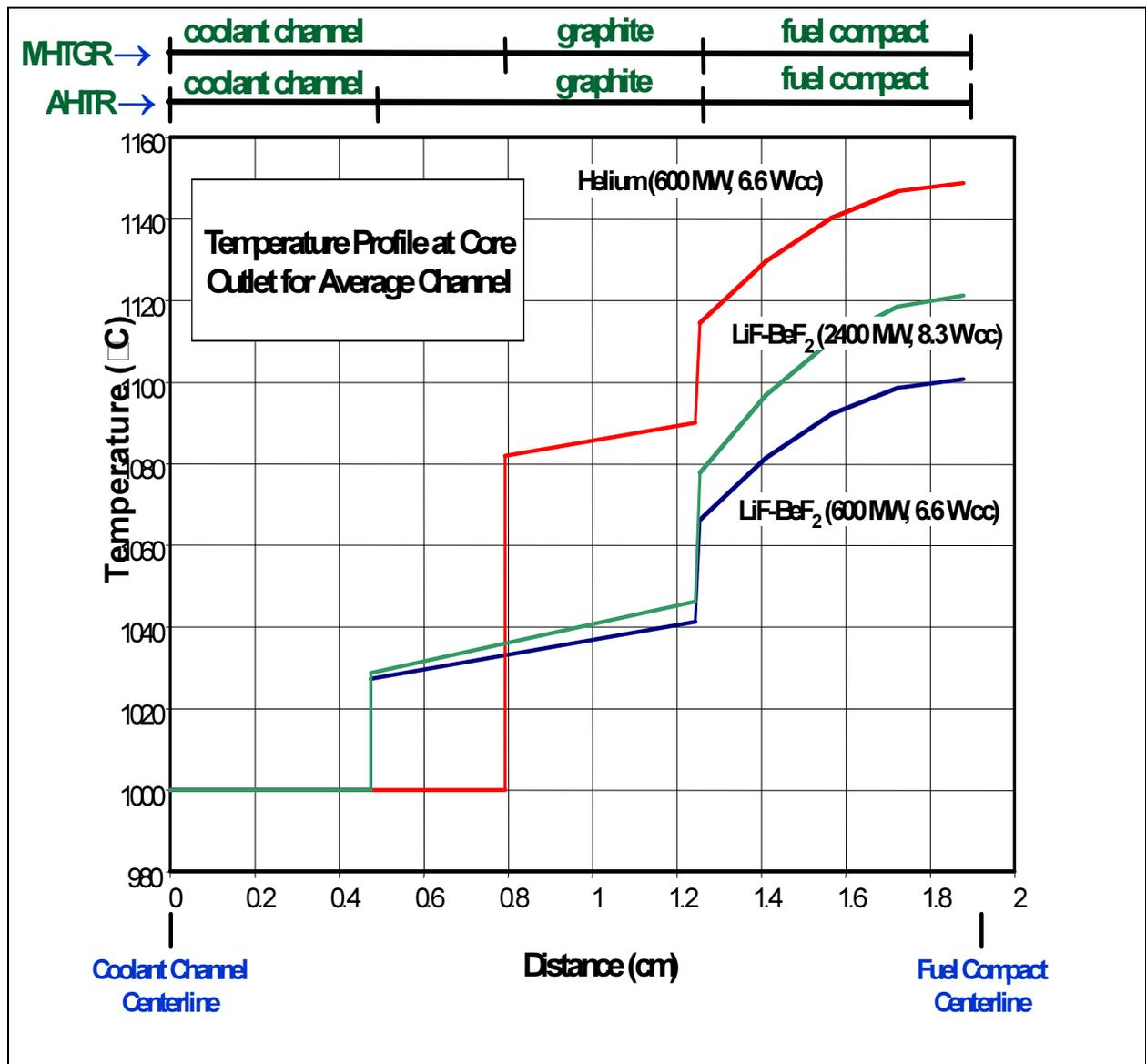
FIG. 4. Temperature profile from the coolant to fuel compact centerline.
