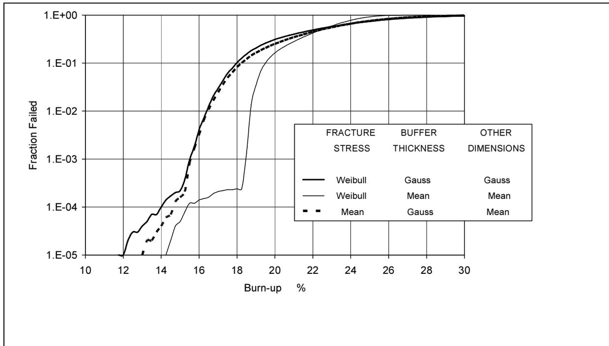
FIG. 6. Effect of variability in fracture stresses and buffer thicknesses and other dimensions on failure fractions.
