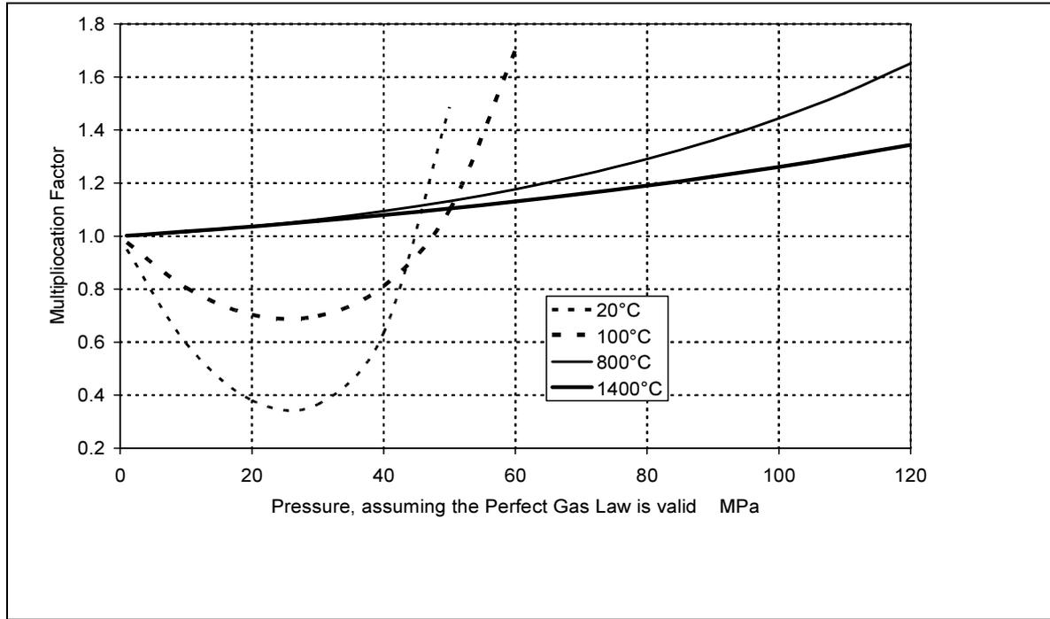
FIG. 2. Correction of fission gas pressures, calculated assuming the perfect gas law.
