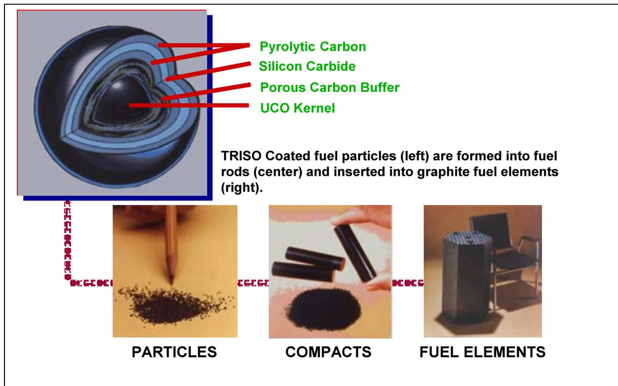
FIG. 1. Cutaway schematic of a TRISO coated fuel particle and pictures of prismatic fuelled high-temperature gas reactor fuel particles, compacts, and fuel elements.
