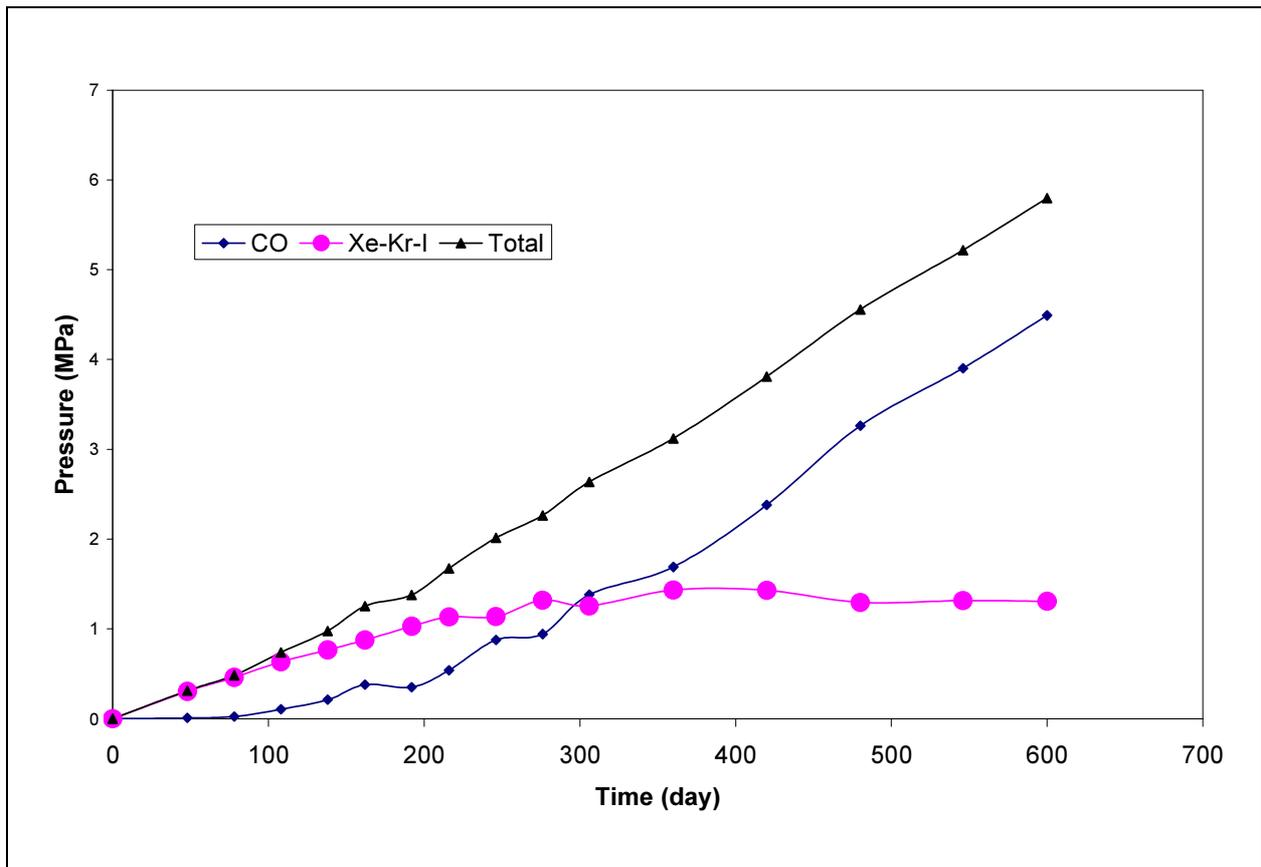
FIG. 3. Coated fuel particle internal pressure (Case I).
