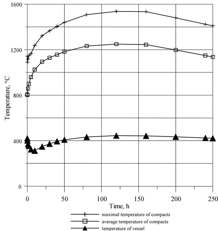
FIG. 4. Temperature state of the core and reactor vessel during depressurization with cooling by RCCS.
