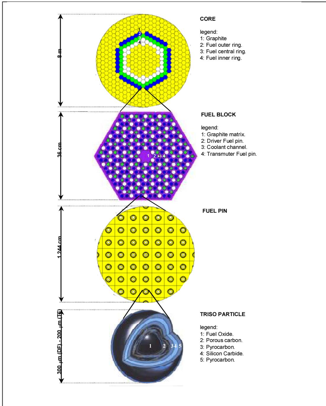
FIG. 1. The gas turbine modular high temperature reactor GT-MHR.
