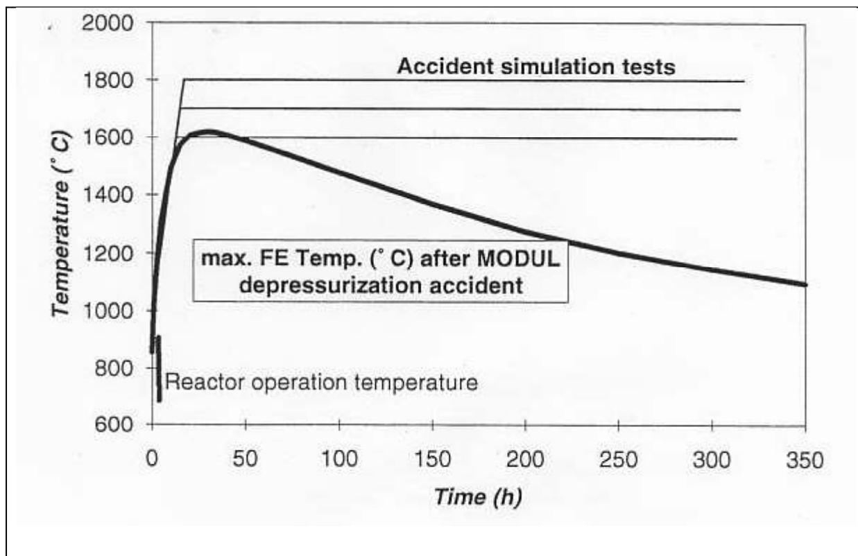
FIG. 5. Temperature evolution during a loss-of-coolant accident in a small HTR and in the heating tests.
