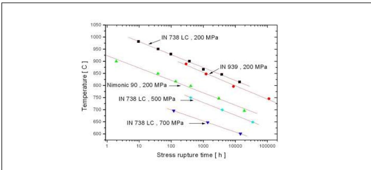
FIG. 5. Iso-Stress plot for different Ni-base superalloys showing a linear relationship between log stress rupture time and temperature<sup>23</sup>.
