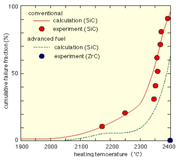
FIG. 10. Comparison ZrC and SiC in heating condition.
