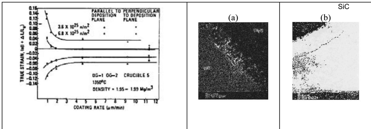
FIG. 2. Irradiation induced strains in PyC as a function of PyC coating rate.
