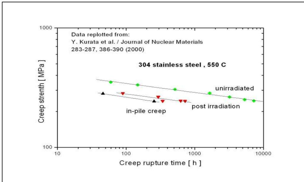
FIG. 6. Influence of irradiation on stress rupture behaviour of 304 stainless steel. Data replotted from [27].
