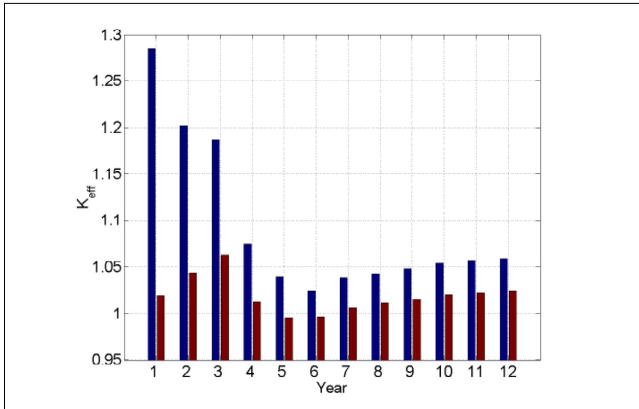
FIG. 3. Values of  $k_{\text{eff}}$  at beginning (left columns) and at the end (right columns) of each year. All values have a relative standard deviation smaller than 0.04%.
