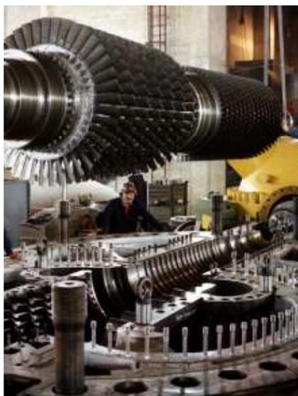
*FIG. 3. Helium turbine plant being fabricated at Oberhausen, Germany.*
