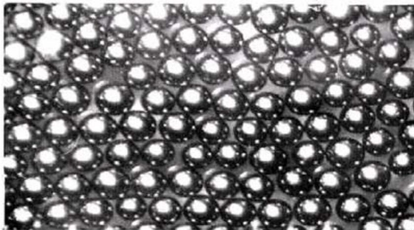
FIG. 5. Sintered UO<sub>2</sub> microspheres of 700 um DIA.
