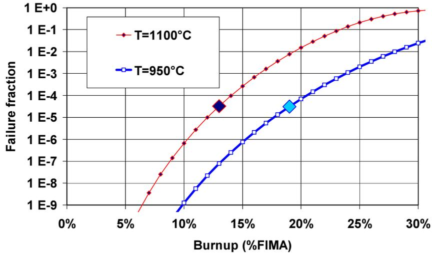
FIG. 3. PANAMA particle failure prediction HFR-EU1: failure on one particle after 13% FIMA at 1100 °C and after 19% FIMA at 950 °C.
