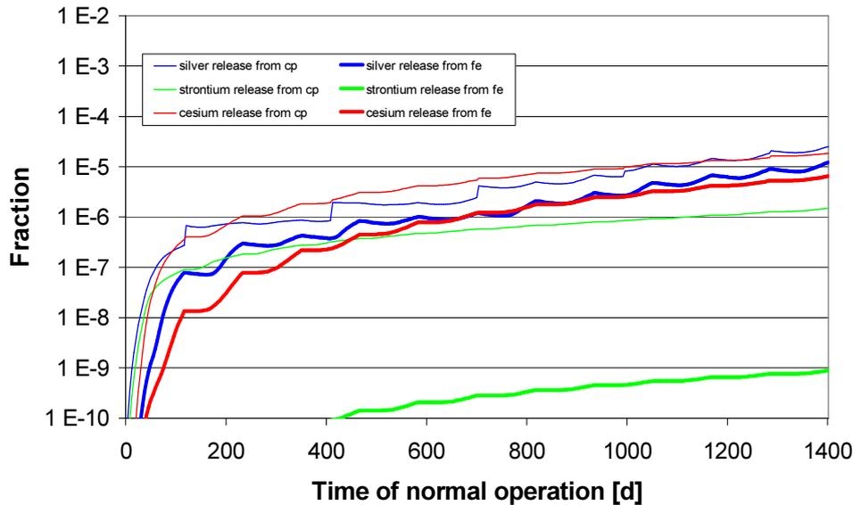
FIG. 3. Fractional release of metallic fission products during normal operation.
