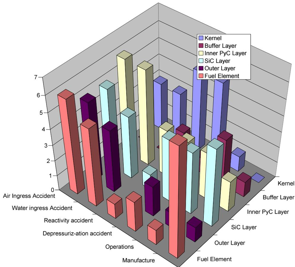
FIG. 1. Census of various safety-significant phenomena for GCR fuelled with coated particle fuel.
