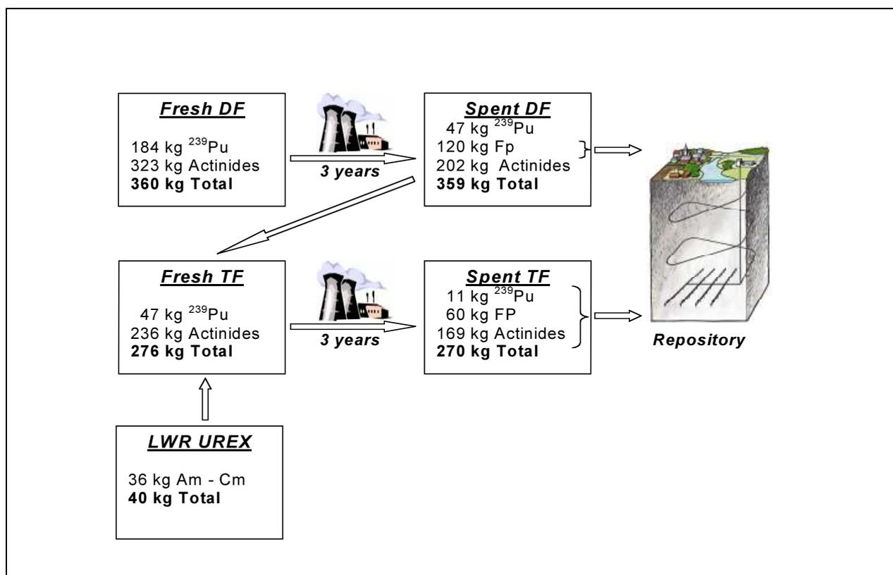
FIG. 4. Yearly mass flow of one module of the GT MHR during the 12<sup>th</sup> year. The total mass takes into account also oxygen.
