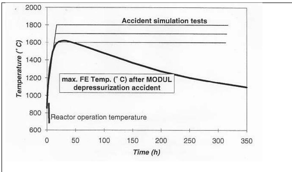
FIG. 4. Temperature evolution during a loss-of-coolant accident in a small HTR and in the heating tests.
