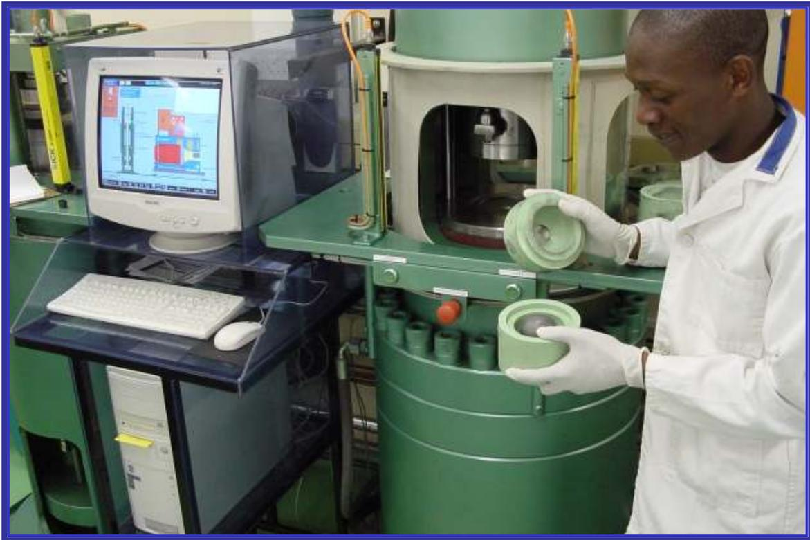
PHOTOGRAPH 7: Placement of fuel cores
