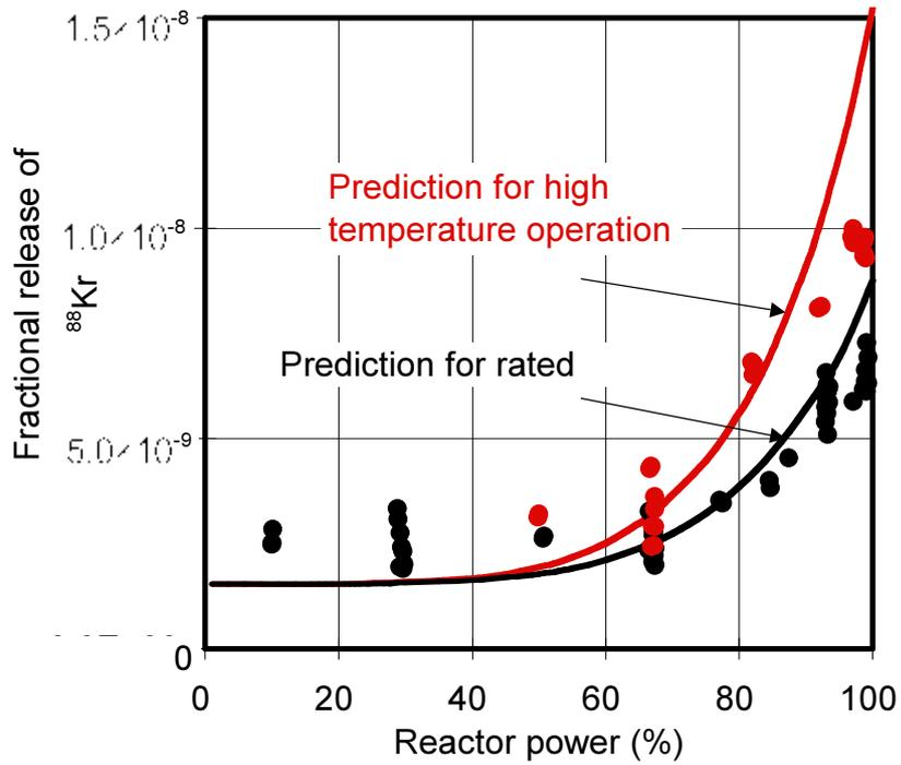
FIG. 5. <sup>88</sup>Kr release rates during rise-to-power operation:
