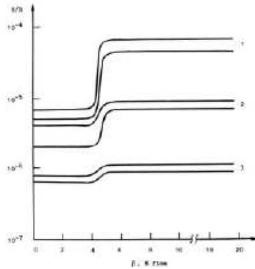
Fig. 14.  $^{85}\text{Kr}$  release from spherical GSP fuel elements based on coated particles with protective coatings of different types:
