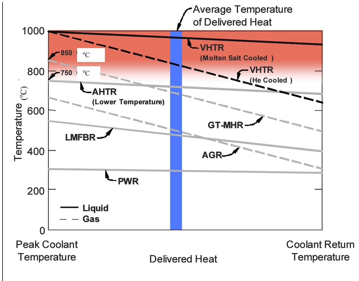
FIG. 5. Temperatures of delivered heat for different reactors.
