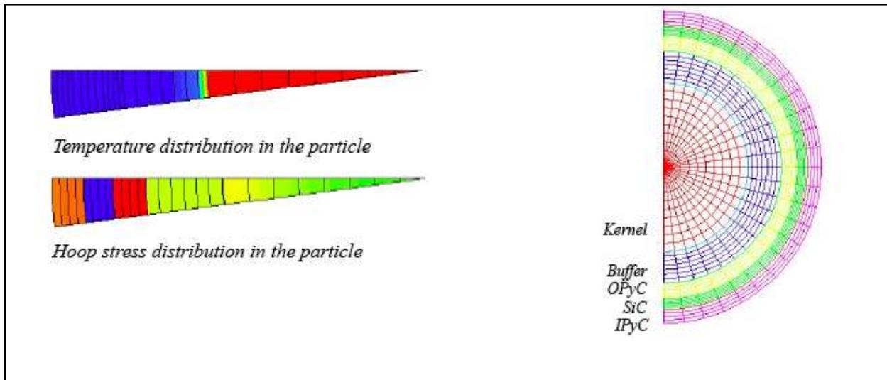
FIG. 11. and 12. 1D particle finite element model, 2D particle finite element model.
