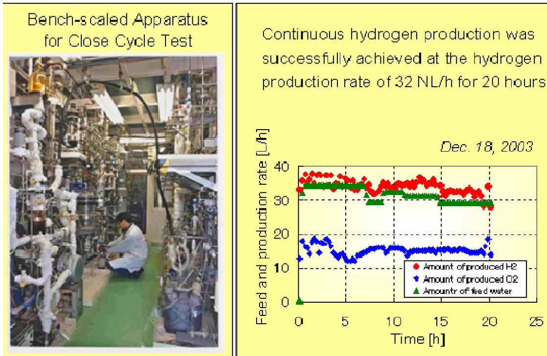
FIG. 7. Result of continuous hydrogen production test.
