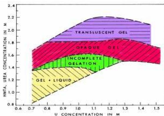
FIG. 3. Gelation field diagram for uranium.
