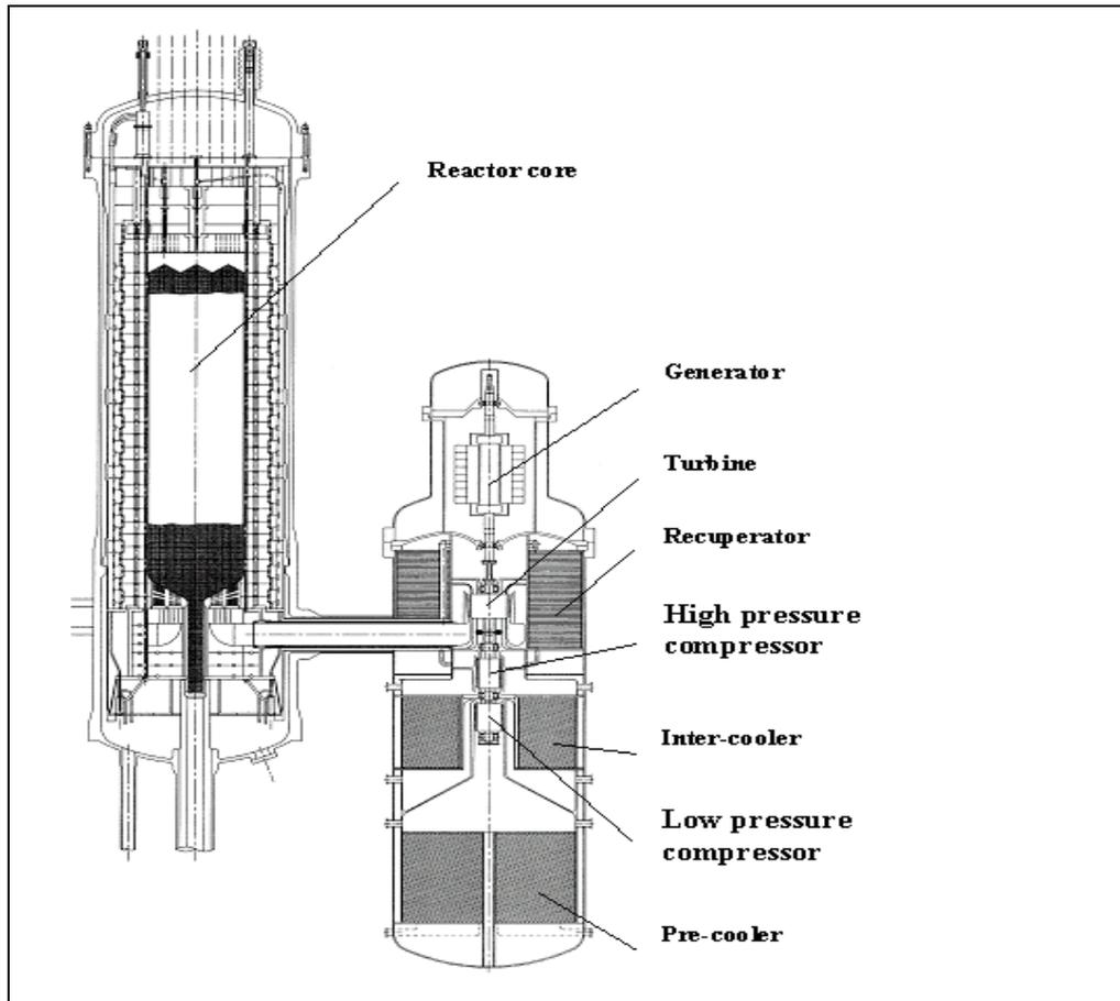
FIG. 1. Cross section of FAPIG-HTGR reactor system.
