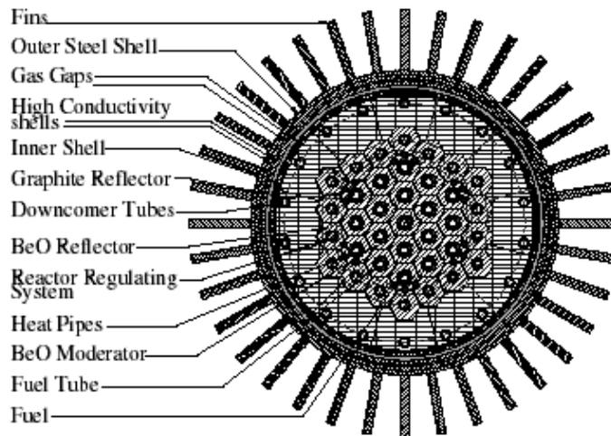
FIG. 1. CHTR core cross sectional layout.
