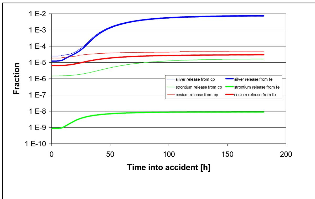
FIG. 5. Fractional release of metallic fission products during core heatup accident.
