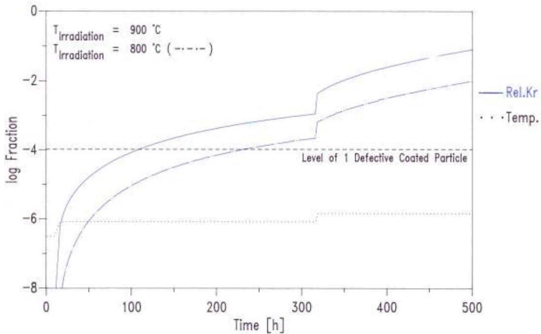
FIG. 2. Prediction of fuel performance for FRJ2-K15/1,3 if heated at 1600 and 1800 °C.
