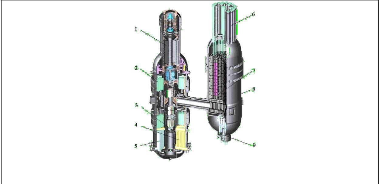
FIG. 1. GT-MHR reactor unit: 1–generator; 2–recuperator; 3–turbo-compressor; 4–intercooler; 5–pre-cooler; 6–control rod drive mechanism assembly; 7–core; 8–vessel system; 9–reactor shutdown cooling system.
