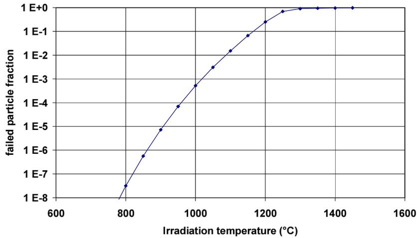
FIG. 4. PANAMA particle failure prediction HFR-EU1 at 20% FIMA for 600-1400°C.
