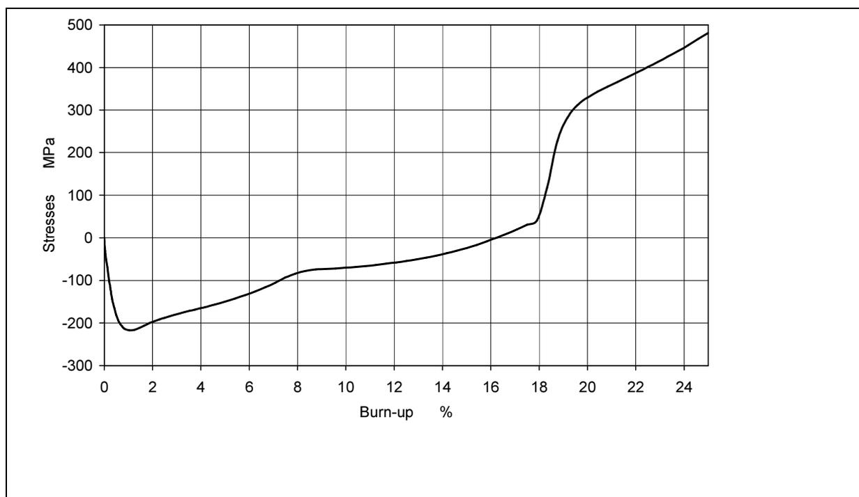
FIG. 4. Stresses in the SiC layer during irradiation.
