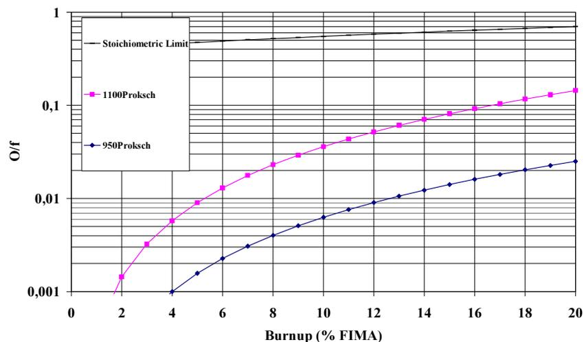
FIG. 1. Oxygen release per fission during burnup of HFR-EU1 and stoichiometric limit.
