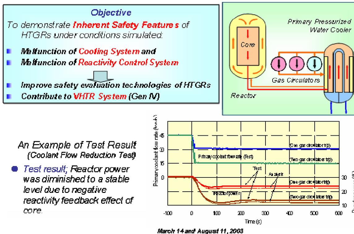
FIG. 4. An example of the safety demonstration test.
