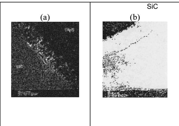
FIG. 3. Comparison of SiC/IPyC interface in (a) German and (b) US fuel.
