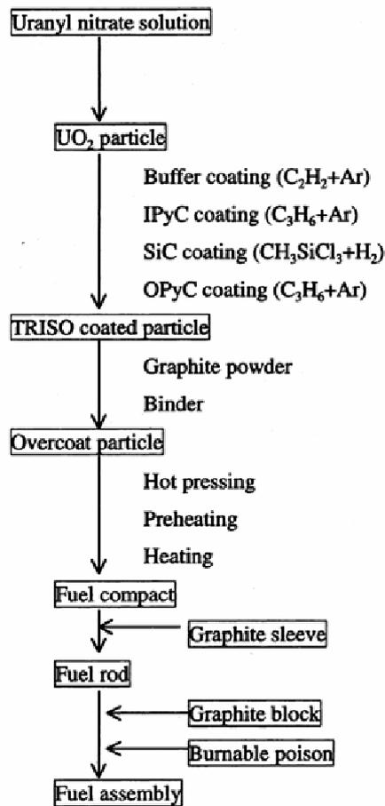
FIG. 3. Flow diagram of HTTR fuel fabrication
