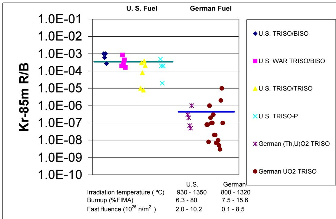
FIG. 5. Comparison of end of life  $\text{Kr-85m}$  R/B from historic German and US irradiations. BISO= particle with PyC only coating; TRISO= particle with PyC/SiC/PyC coating WAR= weak acid resin kernel; TRISO-P = particle with additional outer coating.
