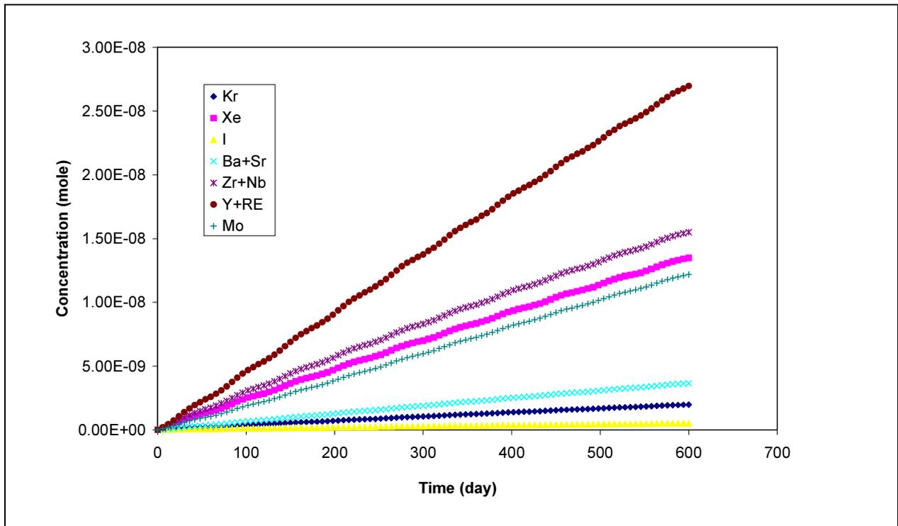
FIG. 2. Fission product concentration during reactor operation.
