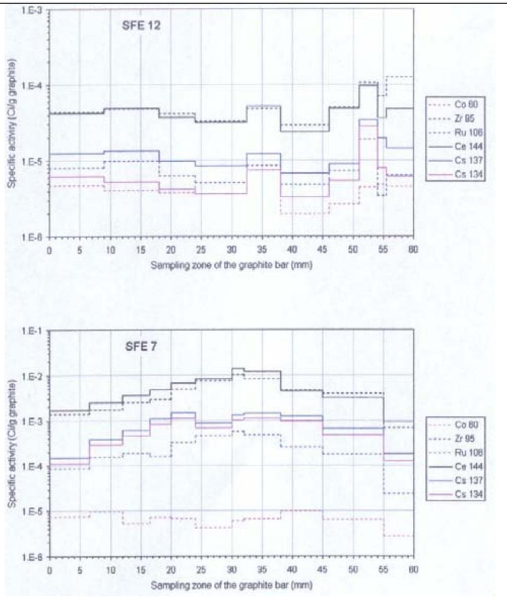
FIG. 3. Radial distribution of  $^{60}\text{Co}$ ,  $^{95}\text{Zr}$ ,  $^{106}\text{Ru}$ ,  $^{144}\text{Ce}$ ,  $^{137}\text{Cs}$  and  $^{134}\text{Cs}$  determined during axial deconsolidation of SFE 12 and SFE 7.
