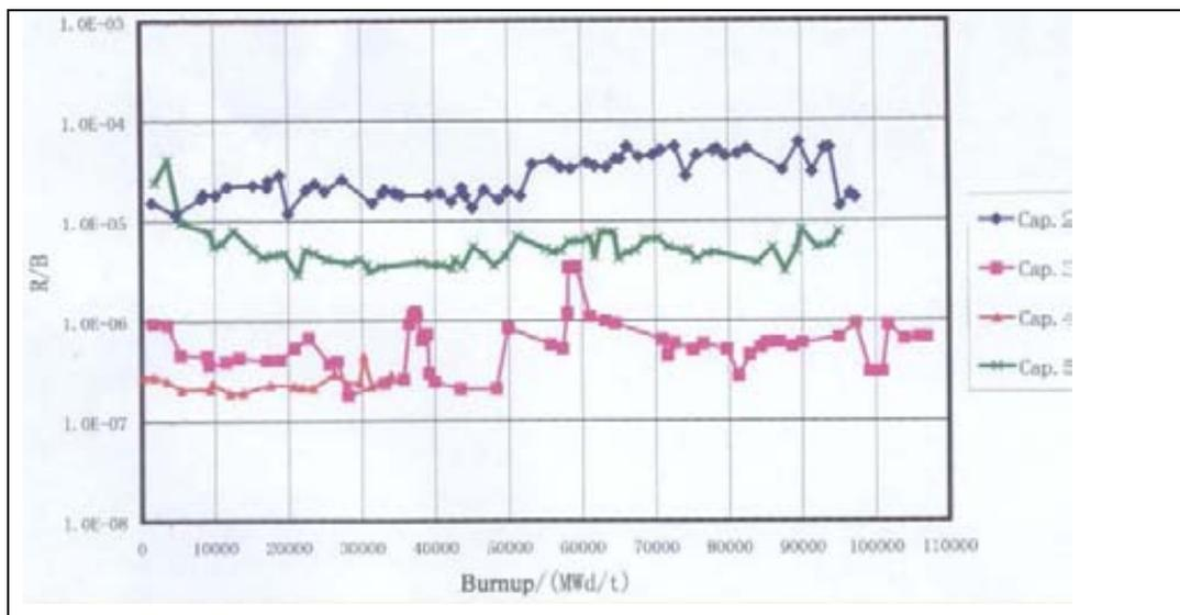
FIG. 1.  $^{85m}\text{Kr}$  release rates of the four fuel elements as a function of burnup.
