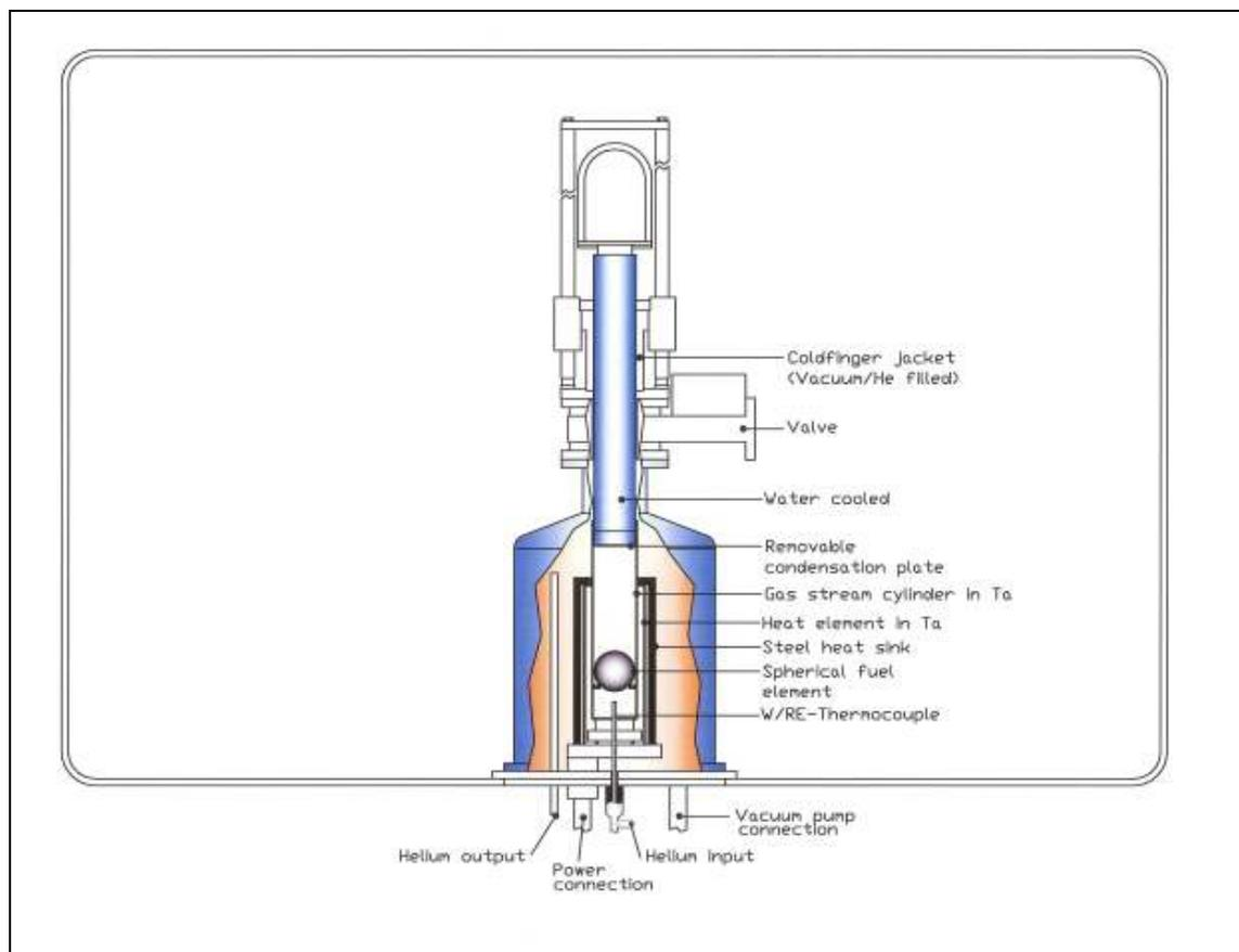
FIG. 1. Cold-finger apparatus (KÜFA).
