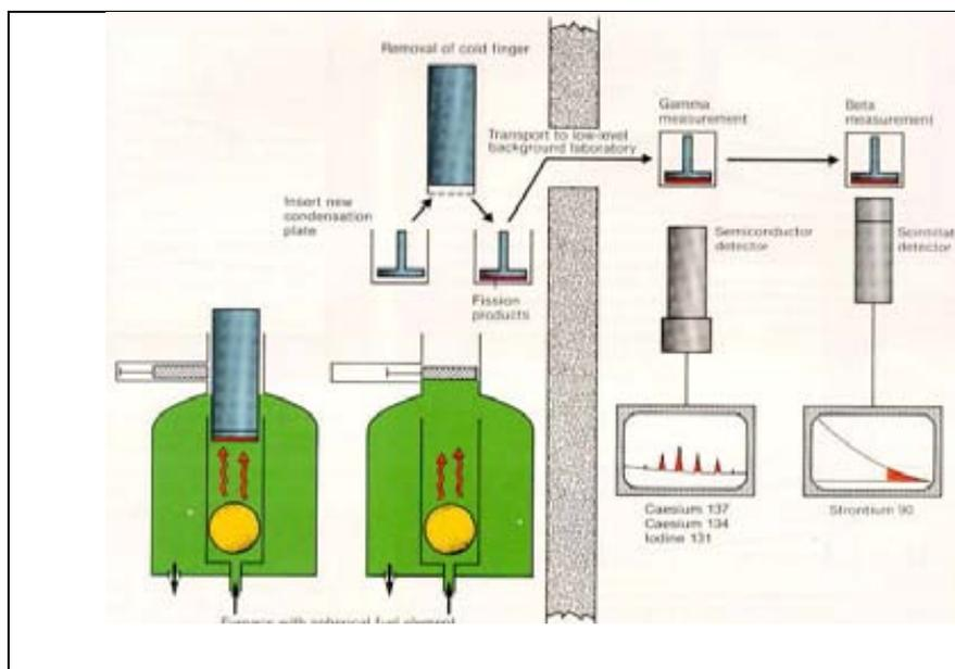
FIG. 9. Schematic of German heating test apparatus KUEFA.
