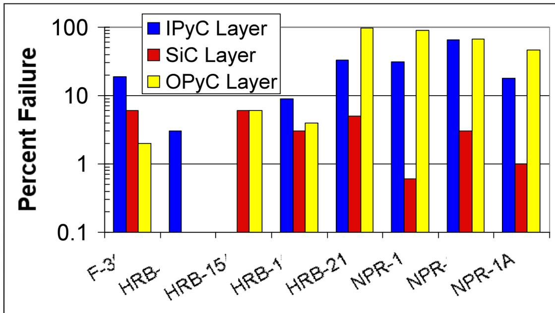
FIG. 6. Failures observed during postirradiation examination of US coated particle fuel over the past 25 years.
