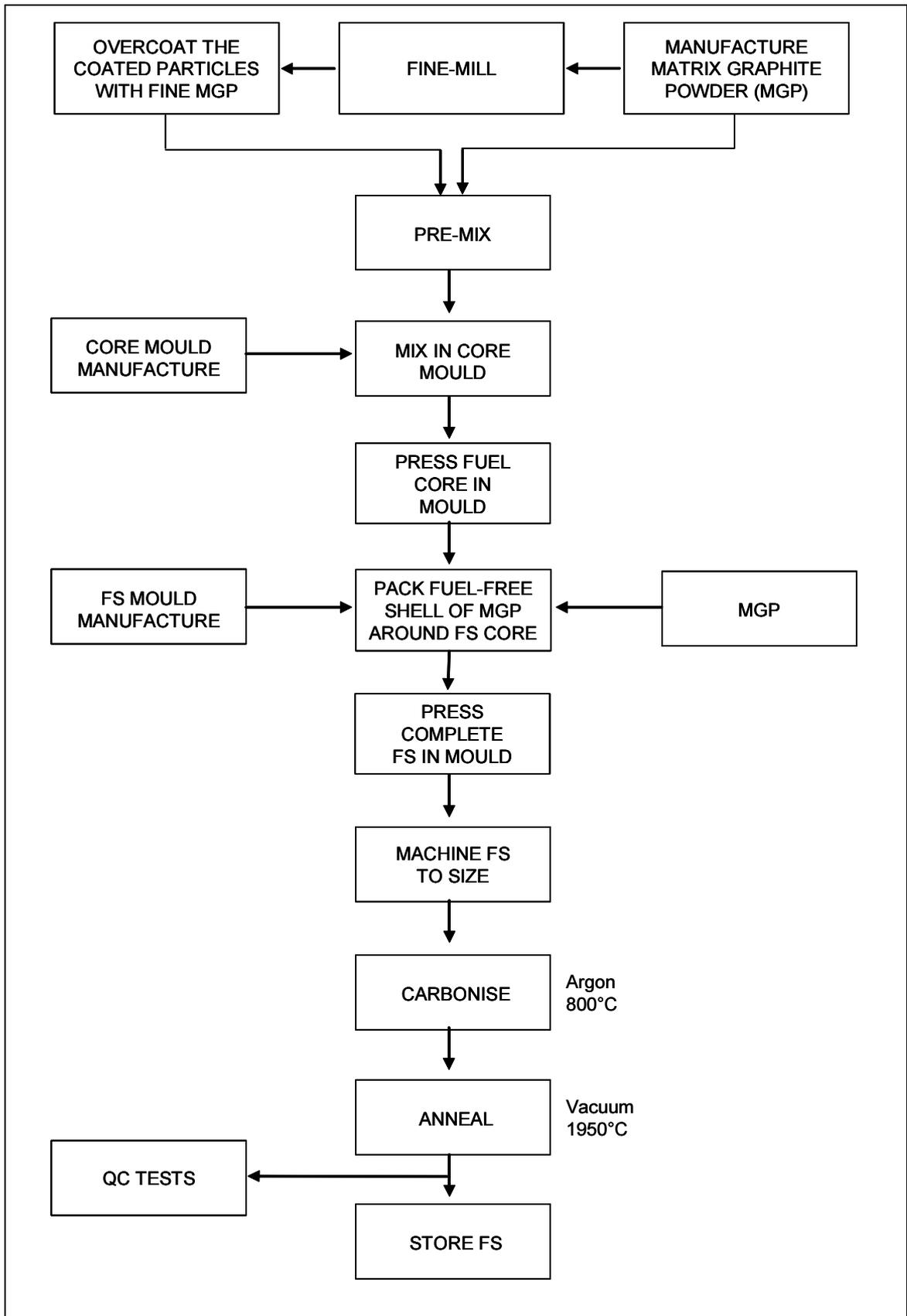
FIG. 3. Fuel sphere (FS) manufacturing.
