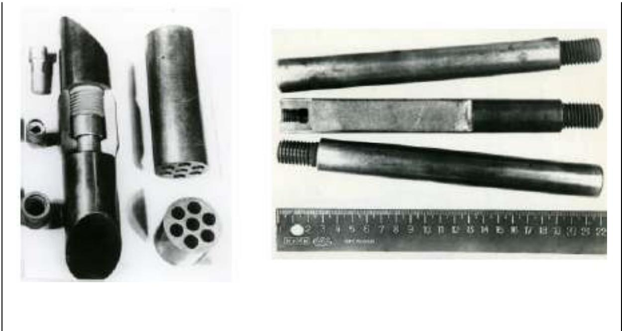
*Fig. 7. Prismatic fuel and absorber elements.*
