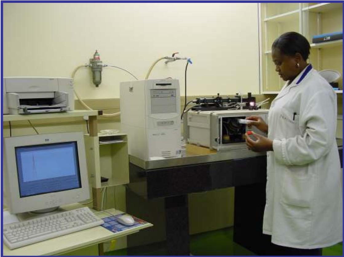
PHOTOGRAPH 9. Optical anisotropy factor determination system
