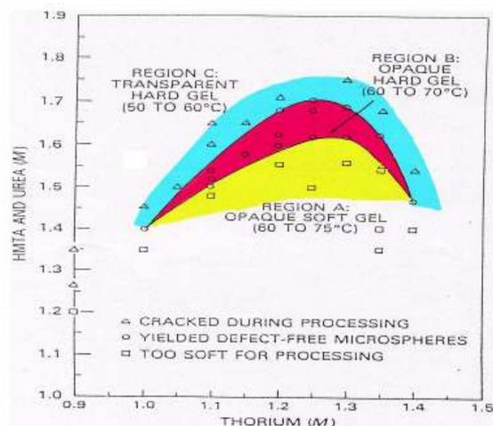
FIG. 4. Gelation field diagram for thorium.
