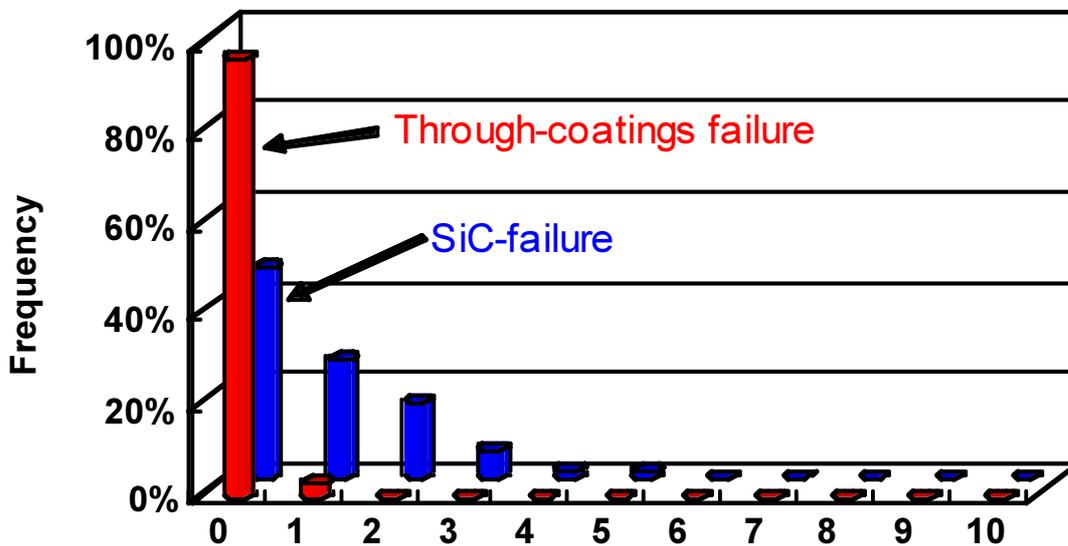
FIG. 4. Number of failed particles in a fuel compact in the first loading fuel fabrication:-average through coating failure,  $2 \times 10^{-6}$  (spec.  $1.5 \times 10^{-4}$ )-average SiC failure fraction,  $8 \times 10^{-5}$  (spec.  $1.5 \times 10^{-3}$ ).
