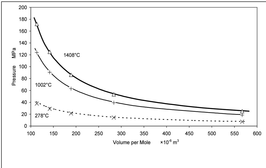
FIG. 1. A comparison between the Redlich-Kwong Equation of State (Lines) and experimental values (Points) for Xenon.
