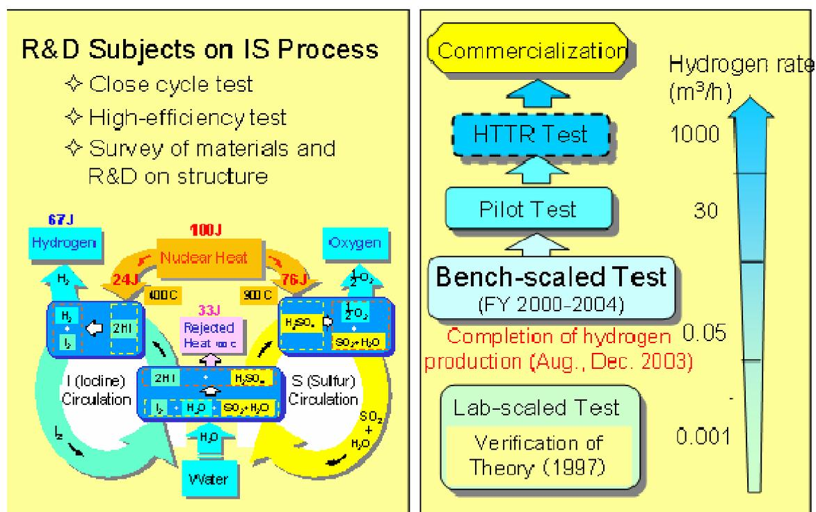
FIG. 6. The diagram of IS process.
