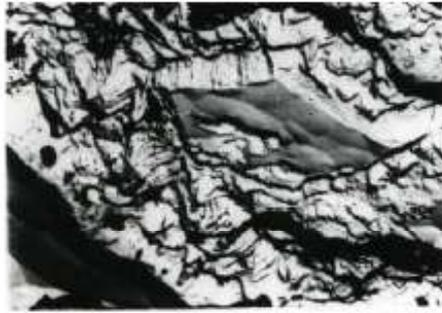
Fig.15. Pyrocarbon sealing of a process impurity in the GSP graphite matrix, 78000.
