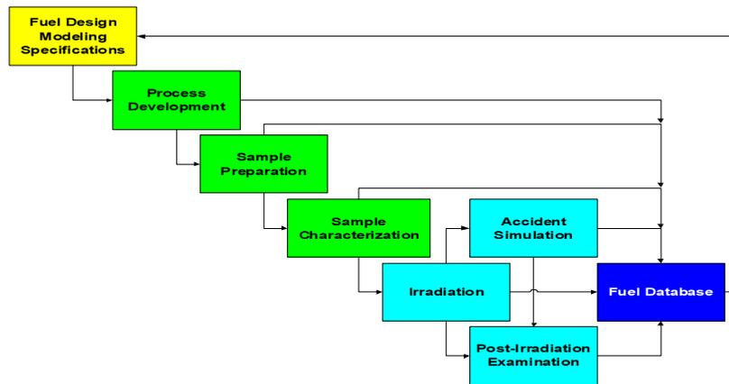
FIG. 1. Fuel development program testing sequence.
