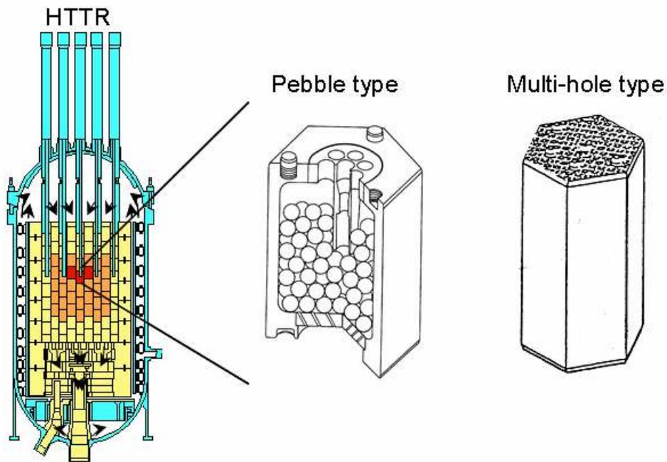
FIG. 8. Fuel irradiation in the HTTR core.
