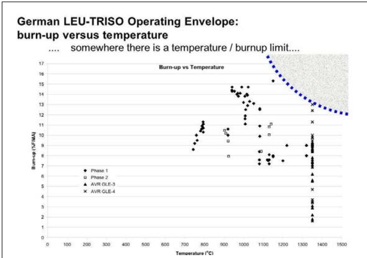
FIG. 6. Burnup-temperature tuples from German high quality TRISO fuel irradiation testing to be used as base material for performance code validation (we are grateful to Johan H Venter of PBMR for providing part of this diagram).
