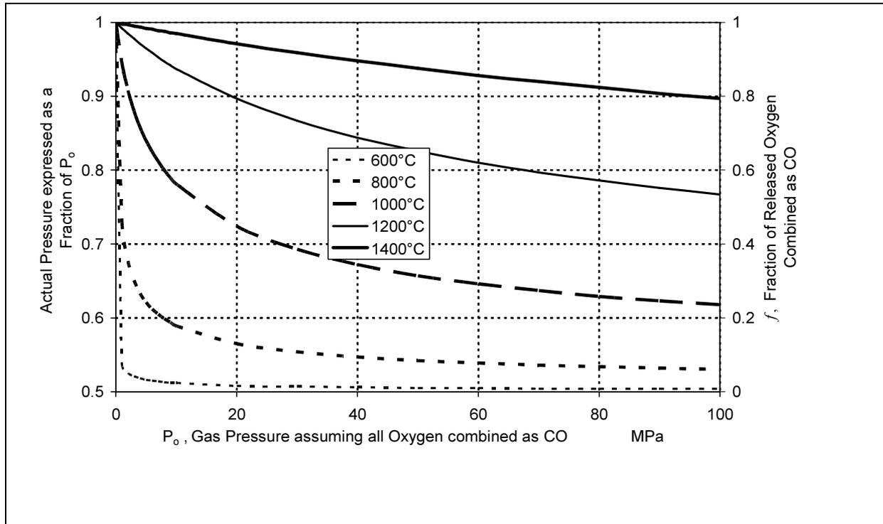
FIG. 3. Effect of CO<sub>2</sub> production on gas pressure.
