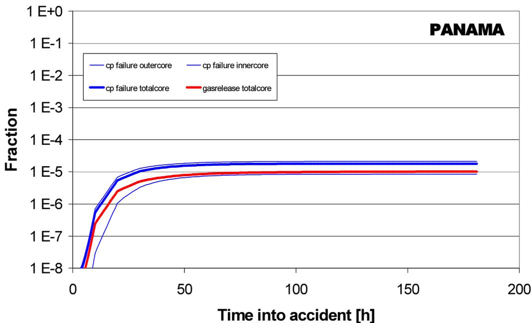
FIG. 4. Failure probability of and gas release from EOL coated particles during core heatup accident scenario.
