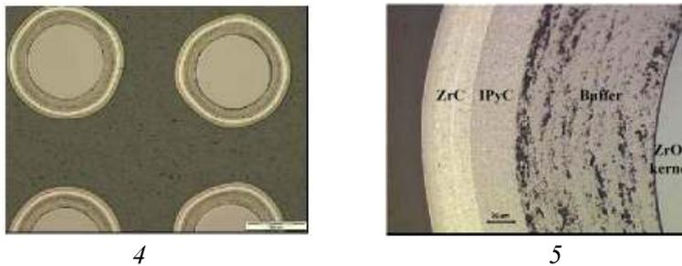
FIG. 4. Optical micrograph of TRISO SiC coated particles produced at CEA Grenoble.
