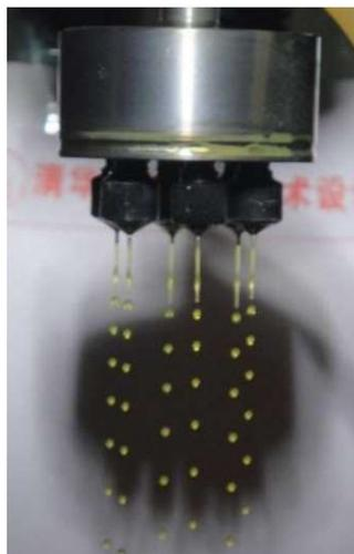
FIG. 24. Casting equipment of the sol-gel in INET (courtesy of Tsinghua University).
