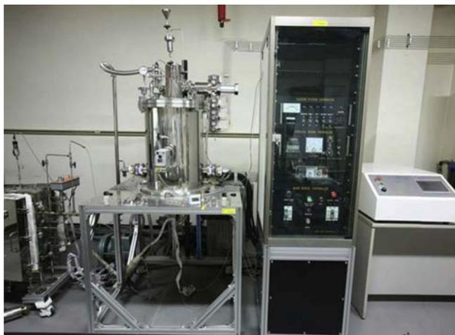
FIG. 21. TRISO coating system (courtesy of KAERI).
