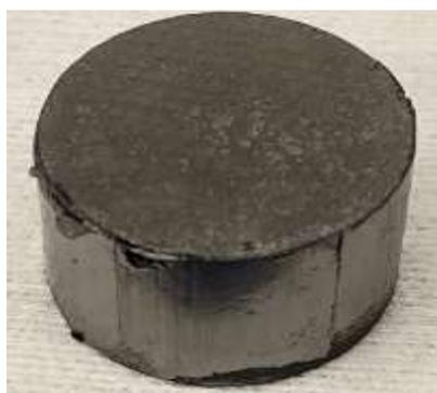
FIG. 18. Sintered FCM fuel with surrogate kernels (courtesy of CNL).
