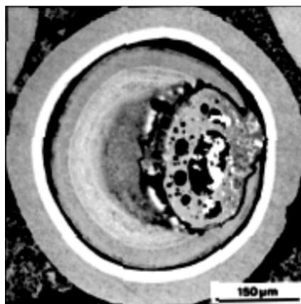
FIG. 112.  $\text{UO}_2$  exhibiting the amoeba effect (courtesy of ORNL).
