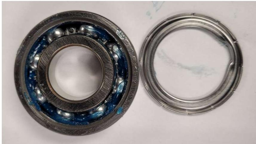
*FIG. 12. Photo of commercial grade single-row double-shielded ball bearings (Courtesy of Kinetrics).*
