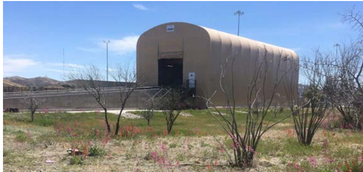
FIG. 44. The muon tomography system DISCOVERY deployed at the US–Mexico border crossing (courtesy of K. Borozdin, Decision Sciences).
