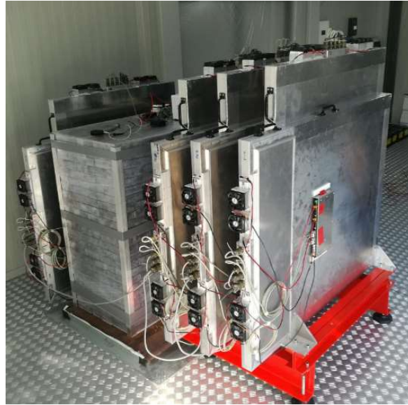
FIG. 33. The first full 1 \text{ m}^2 muon detector system (red) installed in 2019 in the Vesuvius muographic observatory created by the MURAVES collaboration (courtesy of L. Bonechi, Istituto Nazionale di Fisica Nucleare).
