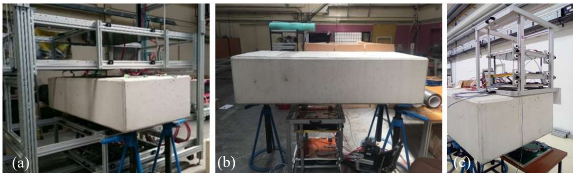
FIG. 10. A concrete slab tested with muon instruments in (a) scattering, (b) transmission and (c) absorption modes (courtesy of S. Procureur, CEA-Saclay).
