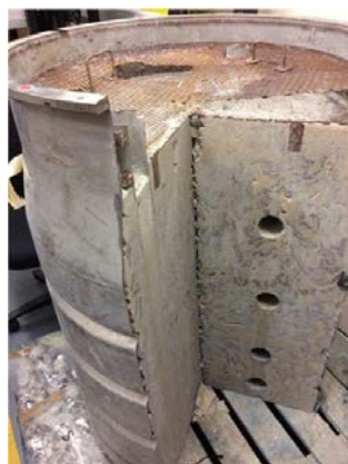
FIG. 49. Photographs of the Lillyhall 500-litre ILW drum prior to installation in the prototype MIS at the University of Glasgow. Shown are the four 60 mm-diameter horizontal cores. The two vertical cores are not pictured (courtesy of R. Kaiser, Lynkeos Technology Ltd).
