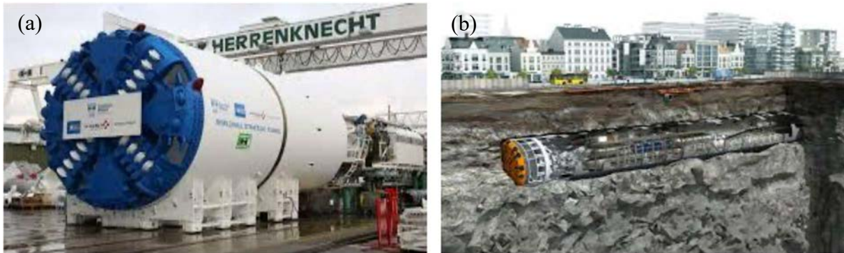
FIG. 21. (a) Picture of a Tunnel-boring Machine (TBM) of the Herrenknecht company during its construction phase, (b) Artistic view of a TBM while digging an urban tunnel (courtesy of J. Marteau, Institut de physique des deux infinis).
