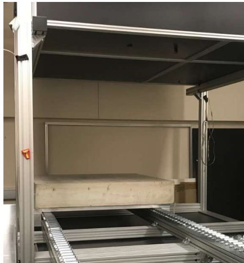
FIG. 13. The ‘Radarplatte’ reinforced concrete block inside the Lynkeos MIS at the University of Glasgow (courtesy of R. Kaiser, Lynkeos Technology Ltd).
