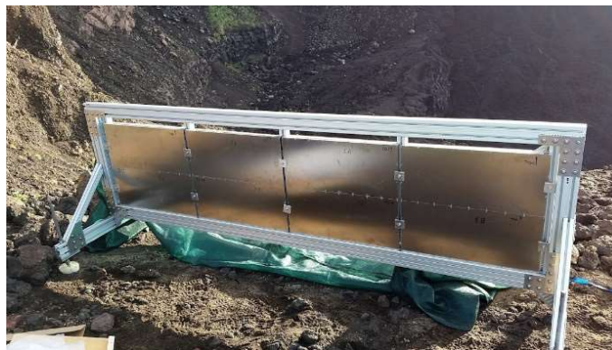
FIG. 31. The nuclear emulsion detector installed at Mount Stromboli in Italy (courtesy of V. Tioukov, Istituto Nazionale di Fisica Nucleare).
