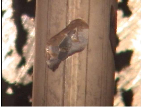
FIG. 2a. Fretting mark on fuel rod.
