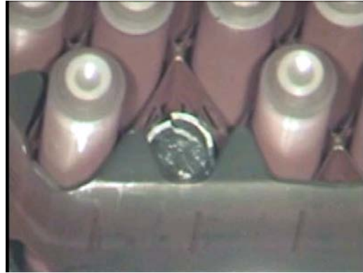
FIG. 2b. Ruptured fuel rod.
