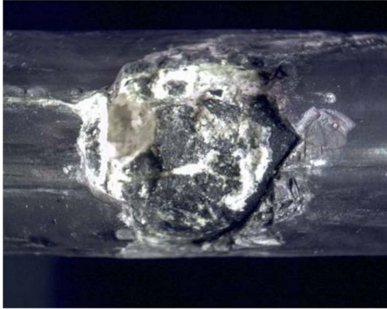
FIG. 3. Damage to the leaking fuel rod at the height of the fifth spacer. The damage is of the secondary fuel rod failure type.
