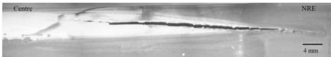
Confirmed defect: large sheath fracture
