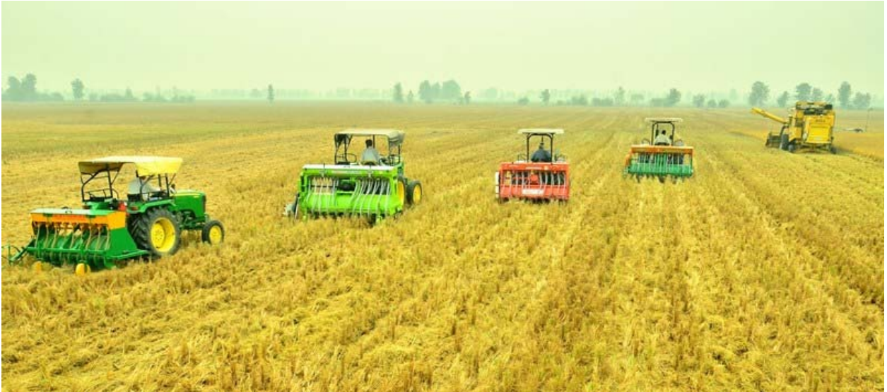
FIG. 7. Combine harvester (extreme right) is harvesting rice in BISA (Borlaug Institute for South Asia) farm in Ludhiana, India and other four machines are Happy Seeders direct seeding wheat with residue mulch. Source: [29].
