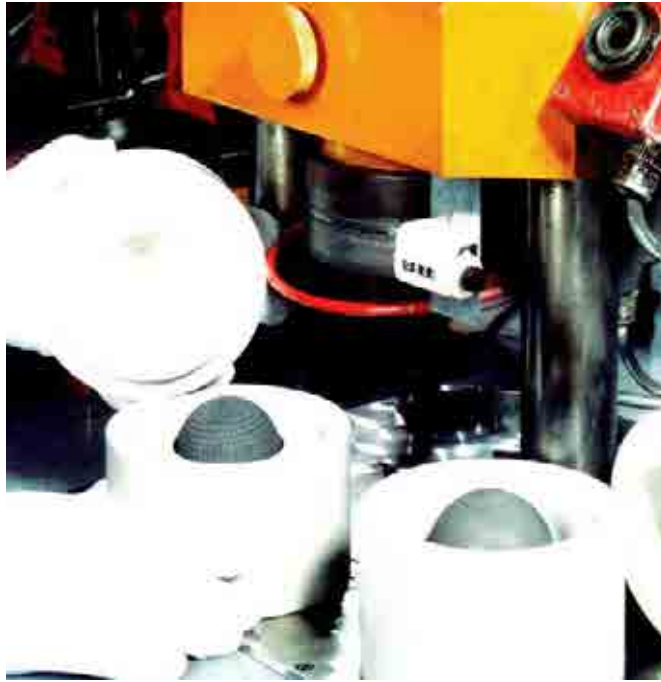
FIG. 19. Silicon rubber dies for fuel spheres.
