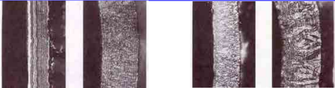
(c) Etched SiC ceramographic sections deposited at 1300, 1500, 1600 and 1700°C.
