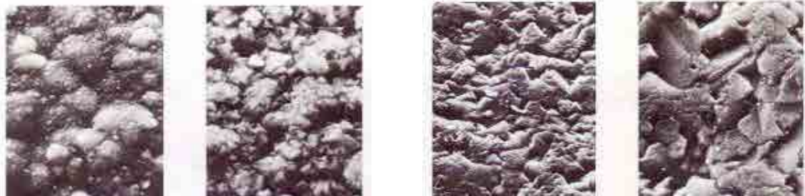
(b) SEM pictures of SiC surfaces deposited at 1300, 1500, 1600 and 1700°C.
