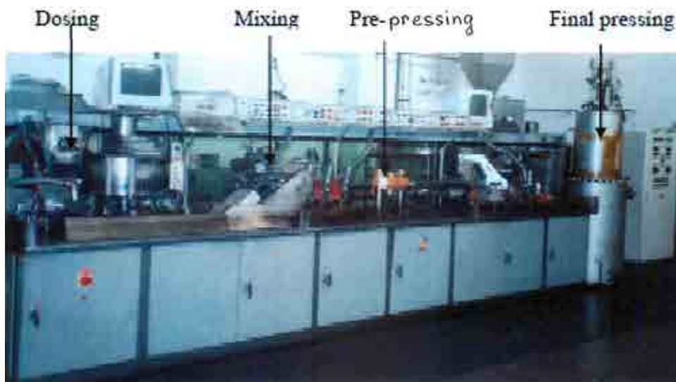
FIG. 18. Moulding and pressing line for green fuel spheres at the INET in China.
