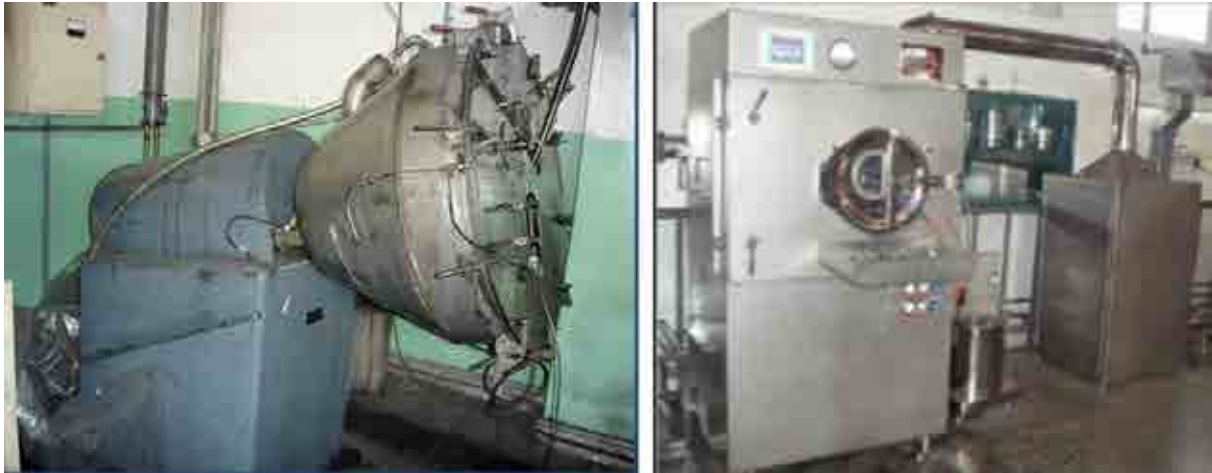
FIG. 16. Old manual overcoating drum that was used by NUKEM in the production of the HEU (Th,U)O 2 and LEU UO 2 TRISO coated particles (left); new automated overcoating facility used at present by INET in the production of LEU UO 2 TRISO particles (right).
