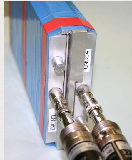
Beryllium neutron detector assembly. A 21cm \times 10.6cm \times 0.5cm Beryllium plate is sandwiched by 2 proportional counters filled with xenon gas
