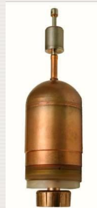
Sealed chambers suitable for DT gas mixture
