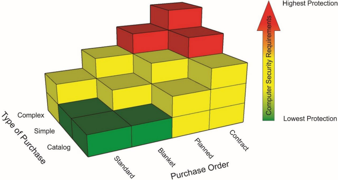
FIG. 6. Procurement matrix – increasing level of computer security requirements and complexity based on purchase types, classification and computer security level requirements.
