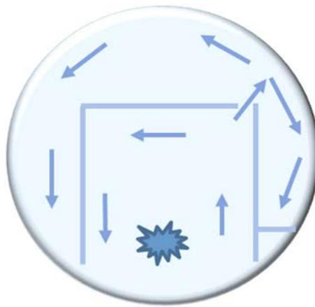
FIG. 14. Flows in the containment with dead end rooms, reproduced from [1].
