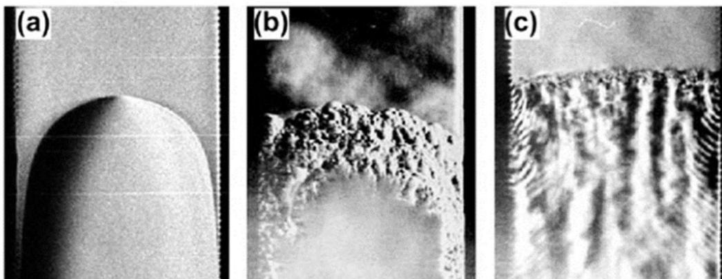
FIG. 6. Combustion regimes: (a) laminar deflagration; (b) turbulent deflagration; (c) detonation [1].
