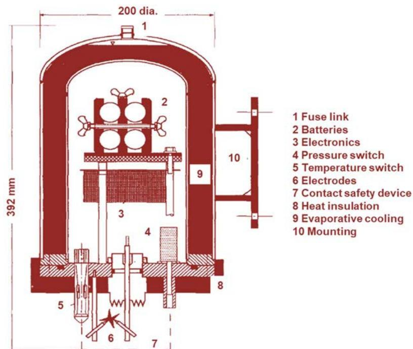
FIG. 36. Spark igniter, reproduced from [1].
