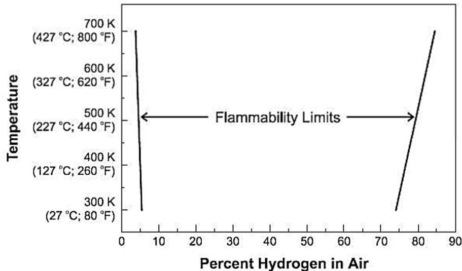
FIG. 4. Flammability limits of hydrogen–air mixture according to temperature [2].
