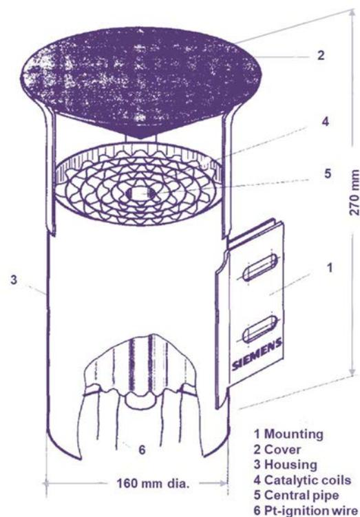
FIG. 37. Catalytic igniter, reproduced from [1].
