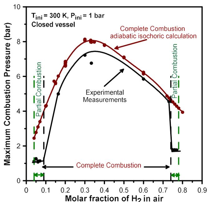
FIG. 23. Measured and calculated maximum combustion pressure of the hydrogen–air mixtures initially at 1 bar and 300 K (1bar = 100 kPa) [38].
