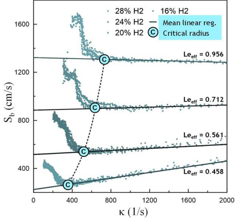
FIG. 32. Burning speed evolution versus stretch rate for hydrogen–air mixtures initially at 1 bar and 295 K, reproduced from [53].
