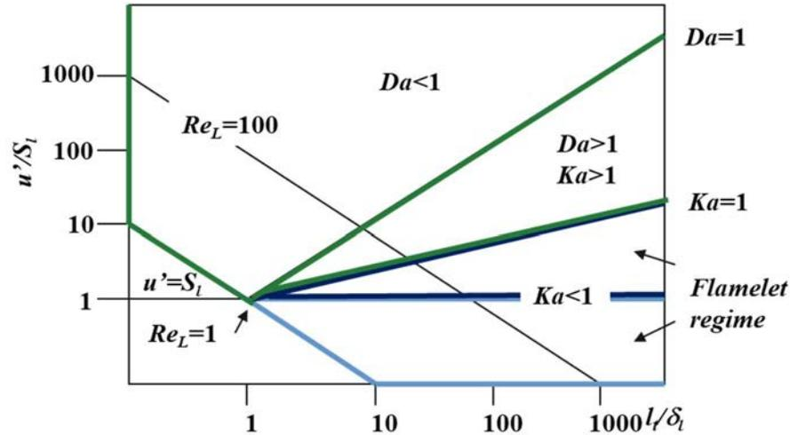
FIG. 8. Borghi diagram, reproduced from [12].
