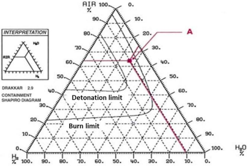
FIG. 16. Shapiro diagram for air–hydrogen–steam mixture [30].
