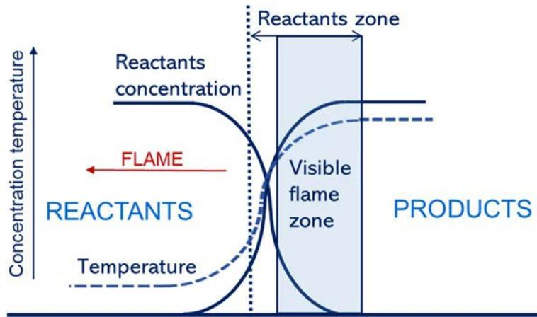
FIG. 5. Concentration and temperature profile in flame propagation, reproduced from [1].
