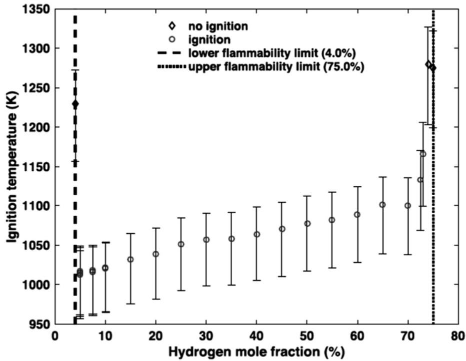
FIG. 19. Evolution of the ignition temperature threshold as a function of hydrogen mole fraction for hydrogen-air mixtures at 101 kPa  $T_0=300\text{K}$ ; lower (LFL) and upper (UFL) flammability limits are shown as dashed and dotted vertical lines, respectively while the error bars indicate temperature uncertainty [32].
