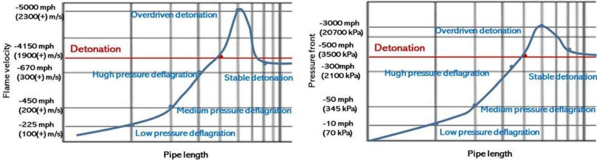
FIG. 9. Flame front velocity (left) and pressure during the DDT (right), reproduced from [14].
