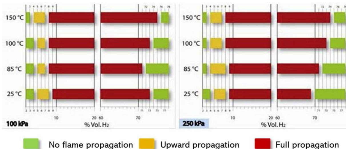
FIG. 22. Flammability limits for hydrogen–air mixture as a function of temperature and pressure[10].
