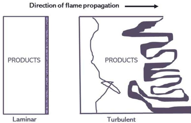
FIG. 7. Configuration of flame propagation for laminar and turbulent deflagration, reproduced from [11].
