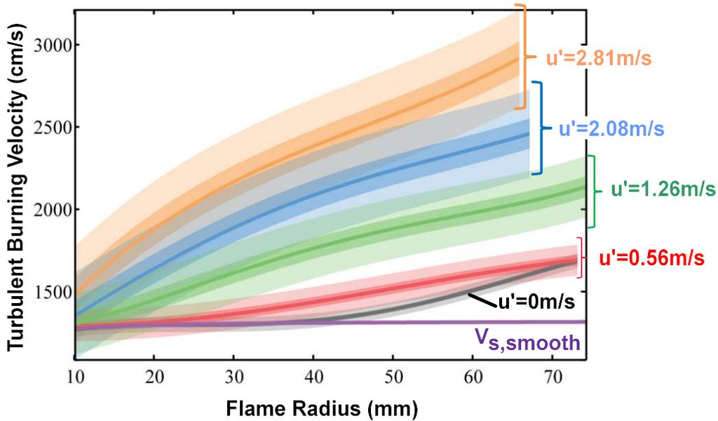
FIG. 33 Turbulent flame speed versus flame radius for different turbulent intensities; the mixture containing 28% of hydrogen in air was initially at 1 bar and 295 K [52].
