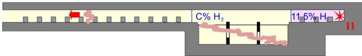
FIG. 29. RUT facility scheme and the piston effect on flame acceleration [43].
