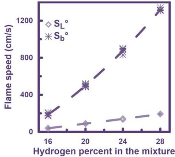
FIG. 31. Laminar flame speed,  $S_L^\circ$ , and laminar burning speed,  $S_b^\circ$ , versus the hydrogen molar percent for hydrogen–air mixture at an initial pressure and temperature of 1 bar and 295 K respectively, reproduced from [52].
