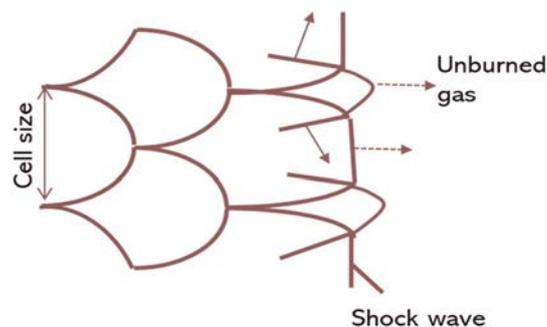
FIG. 25. Detonation cell size, reproduced from [1].
