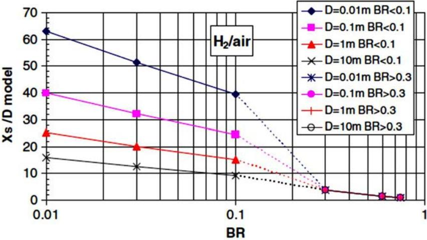
FIG. 12. Run-up distances in stoichiometric hydrogen–air mixtures at 298 K and 1 bar initial pressure as a function of blockage ratio (BR) for various tube diameters [19].
