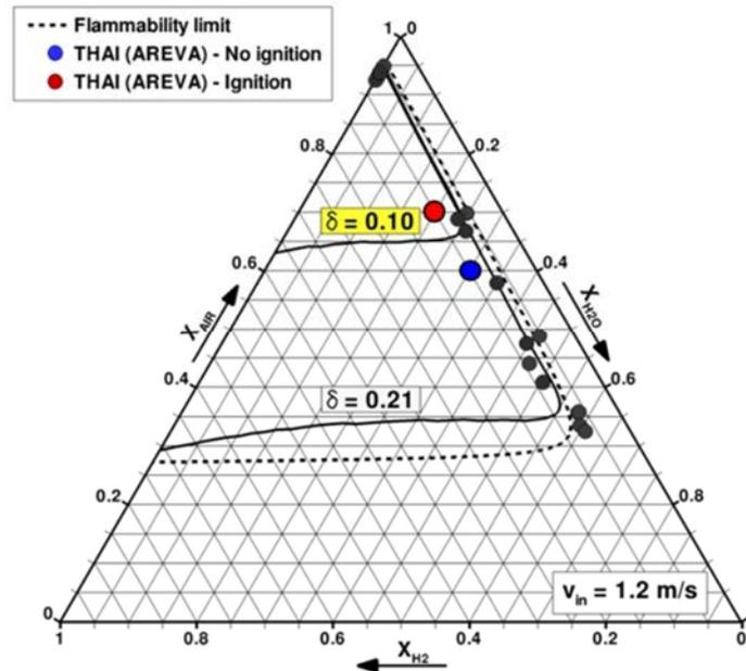
FIG. 21. Impact of lack of oxygen on the limit of ignition of hydrogen by the recombiners AREVA [35].
