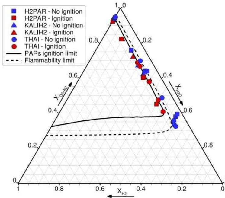
FIG. 20. Limit of ignition of hydrogen by the AREVA recombiners established with the code SPARK (at 1 atm) [37].
