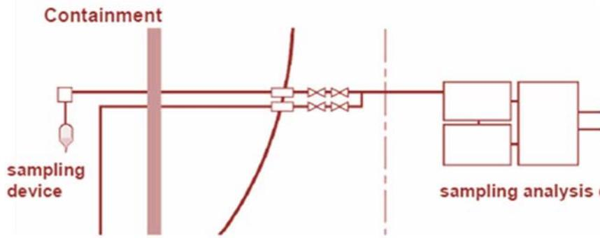
FIG. 35. Schematic diagram of sampling system to measure hydrogen concentration, reproduced from [1].
