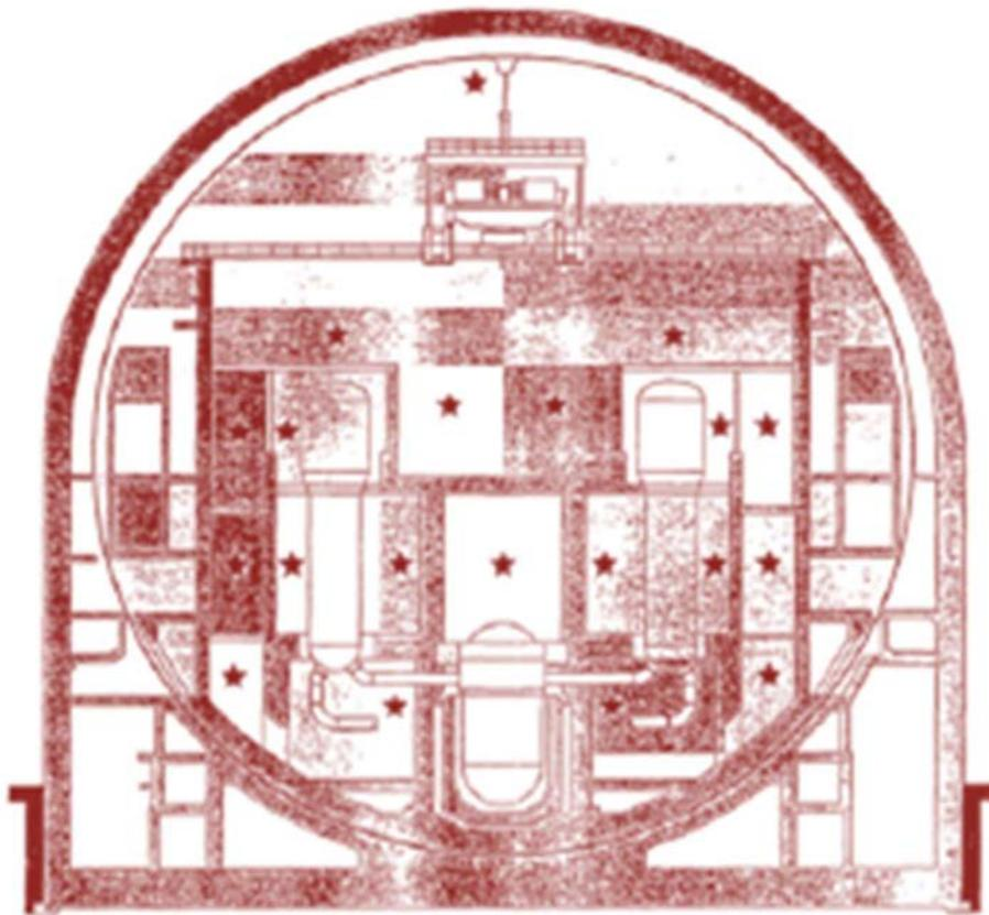
FIG. 39. Distribution of PARs in large dry PWR containment, reproduced from [1].
