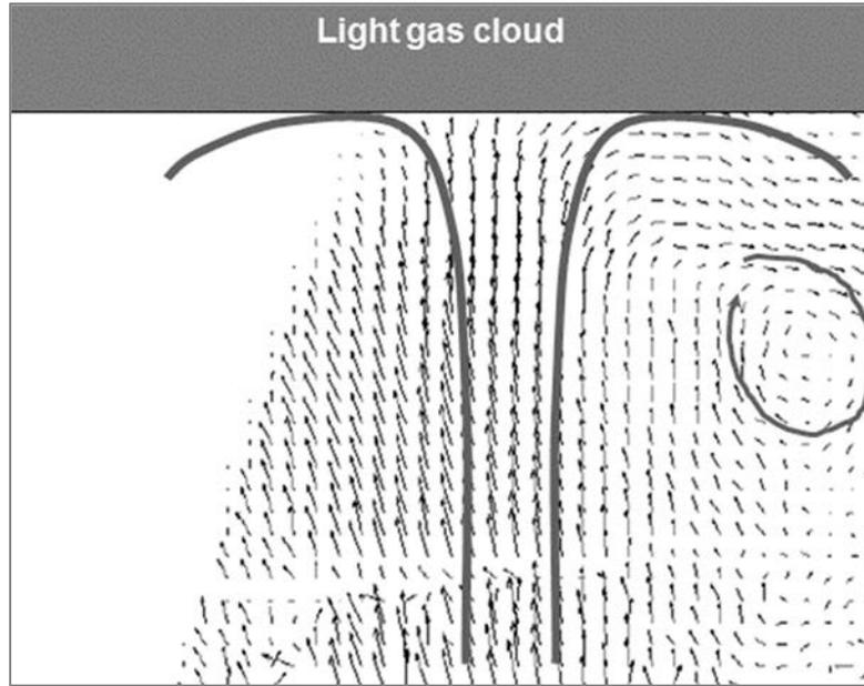
FIG. 2. Gas entrainment and vortex formation at the light gas layer interface [courtesy of Becker Technologies, Germany].
