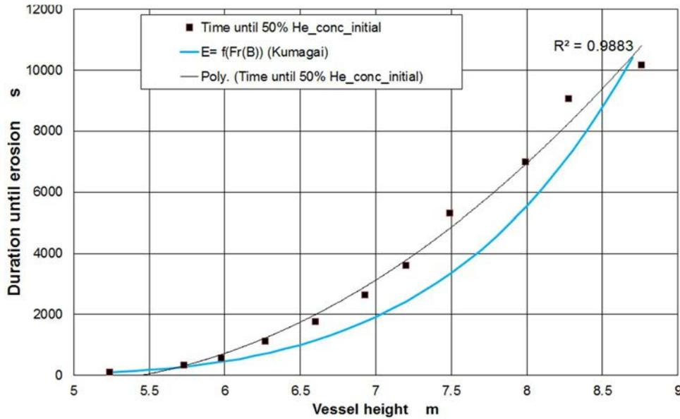
FIG. 3. Experimental and literature data on duration until erosion of the helium stratification as a function of containment vessel height [7].
