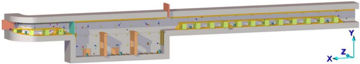
FIG. 28. RUT facility scheme (65 m length, height 6 m, canyon length 15 m, depth 2.5 m) [32].
