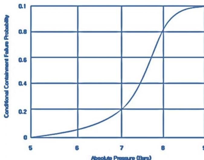
FIG. 34. Failure probability of containment according to pressure loads, reproduced from [1].
