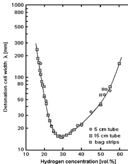
FIG. 11. Experimental measurement of detonation cell size for hydrogen-air mixture [11][18].
