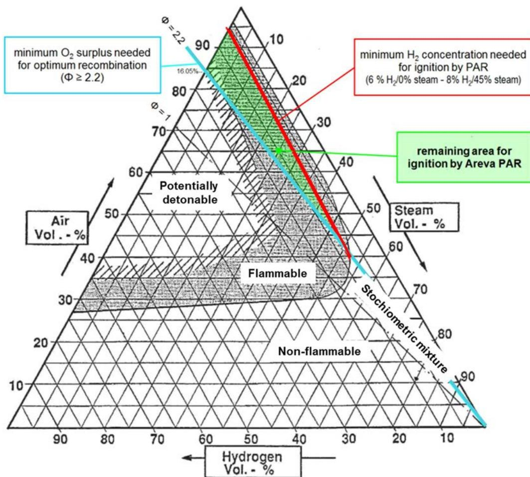
FIG.40. Ternary diagram: area of possible ignition by PAR, resulting from THAI tests [35].
