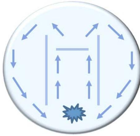
FIG. 13. General convection in the containment with missile shield, reproduced from [1].
