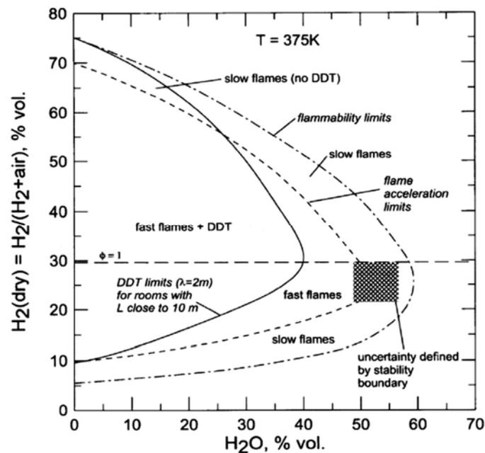
FIG. 26. Characterization of hydrogen–steam–air gaseous mixtures propensity to lead to flame propagation and flame acceleration [32].
