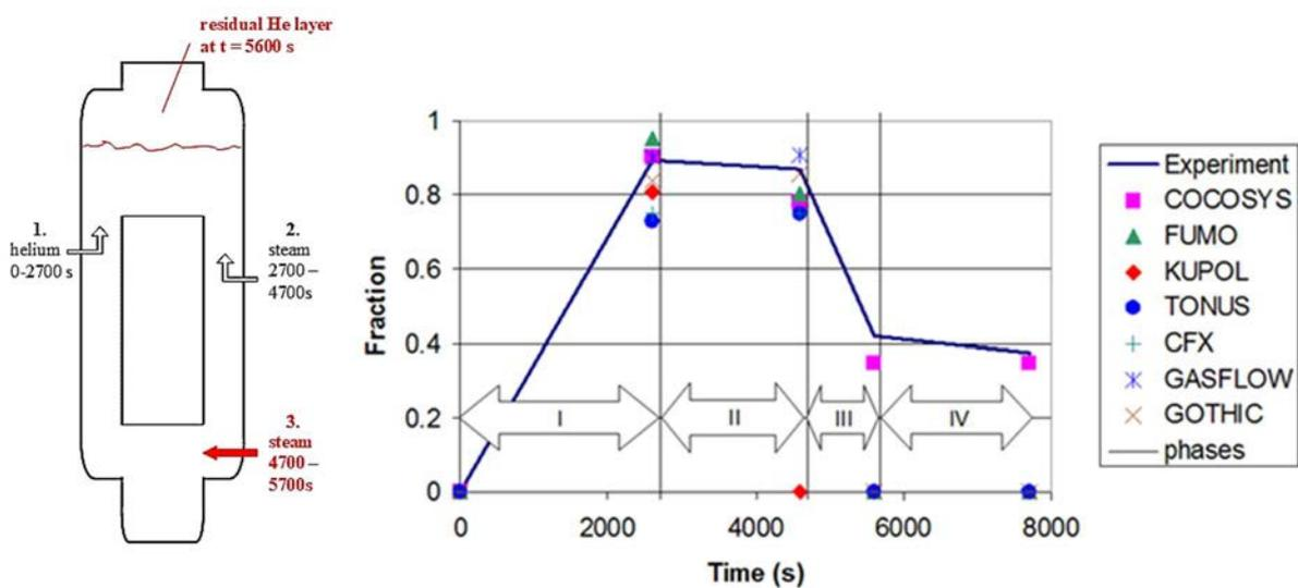
FIG. 1. Experimental and simulated fractions of detonable gas mass [4].
