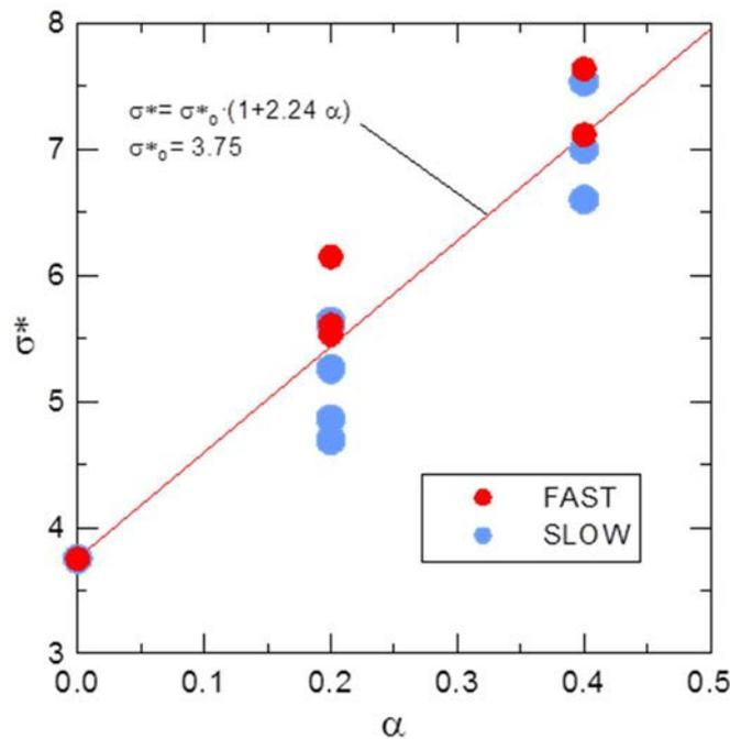
FIG. 27. Lateral venting effect on FA criterion [32].
