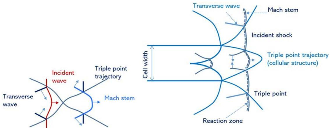
FIG. 10. Structure of detonation waves and triple point trajectory (left) and time evolution of fish scale detonation cell (right), reproduced from [16][18].
