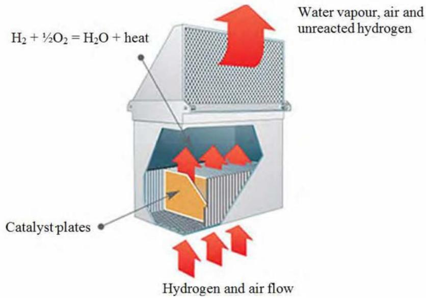
FIG.38. PAR components and flow of hydrogen [59].
