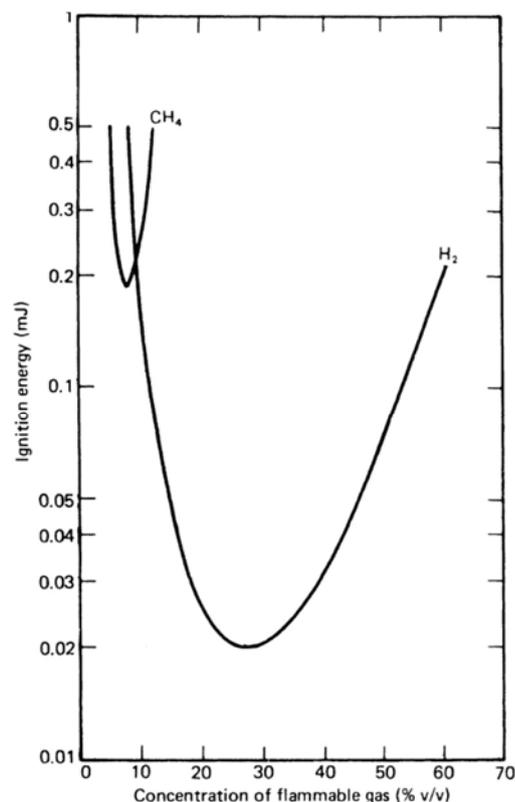
FIG. 18. Ignition energy of hydrogen–air mixtures compared to methane air mixture ignition energy [31].
