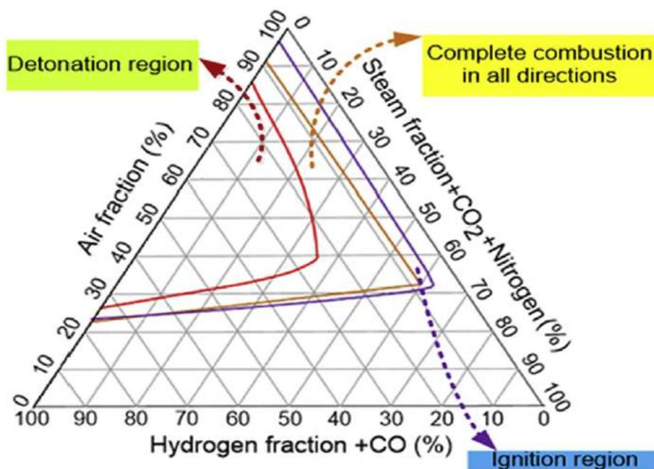
FIG. 17. Shapiro diagram for air–hydrogen–steam mixture with additional gases [22].
