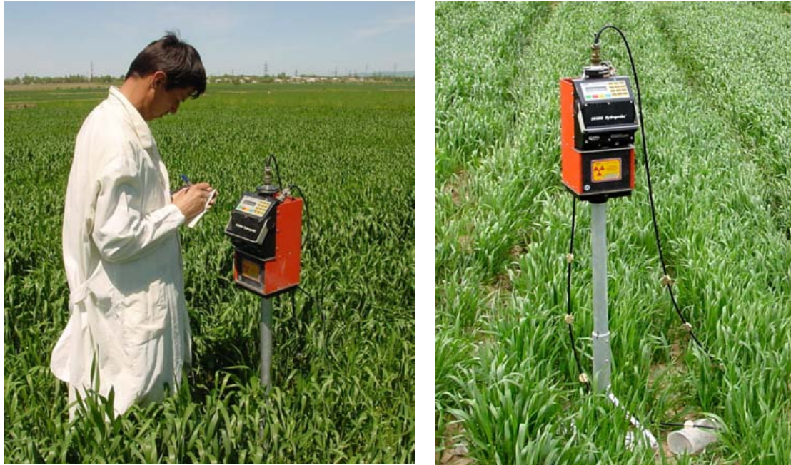
Figure 3.6. (Left) Using a NMM on a depth control stand during water content determinations in a winter wheat field near Tashkent, Uzbekistan. (Photograph courtesy of Dr. N. Ibragimov, Uzbekistan National Cotton Growing Research Institute, Tashkent.) (Right) A photograph taken earlier in the season shows the base of the depth control stand. Note the plastic bottle bottom that was used to protect the access tube.
