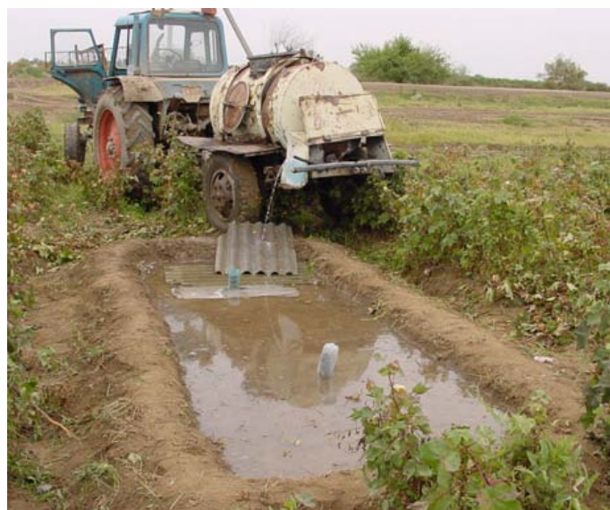
Figure 3.7. Creation of a wet site. In the training site depicted, only two access tubes were installed, although three would be preferred for an accurate calibration.
