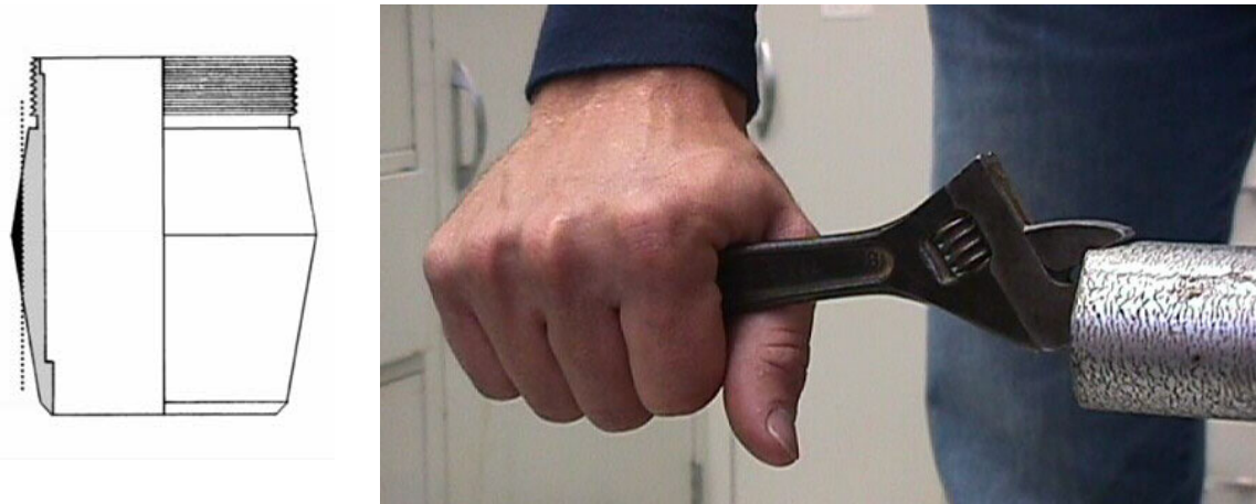
Figure 3.3. (Left) Example of a “Quick relief” coring tube bit (Giddings Machine Company). To obtain a tighter fit of the access tube in the cored hole, remove the bit material outside of the dotted line.
