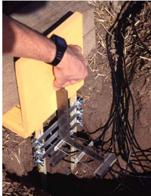
Figure 4.5. TDR probe placement jig. The right angle square and clear plastic spacers are used to ensure that the probe rods are parallel to the soil surface. The spacers, which have identical dimensions, are slotted on one side to slip on and off the probe rods. The plastic spacers also ensure that the rod separation distance is the same at the point where rods enter the soil as it is at the head of the probe, thus minimizing any air pockets along the rods that might be created during insertion. A rule in metric units on each yellow leg allows accurate placement of the aluminium cross bars. The probe rods are set on top of a bar before squaring the probe axis to be perpendicular to the yellow backplate. The probe is pushed partly into the soil, the distal spacer is removed, the probe is inserted further, the proximal spacer is removed, the probe is inserted further, the crossbar is removed, and the probe is inserted fully so that the head is in firm contact with the soil.
