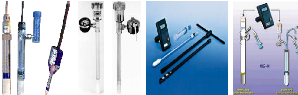
Figure 8.1. Some types of tensiometers available in the market ( http://www.sowacs.com/ ).
