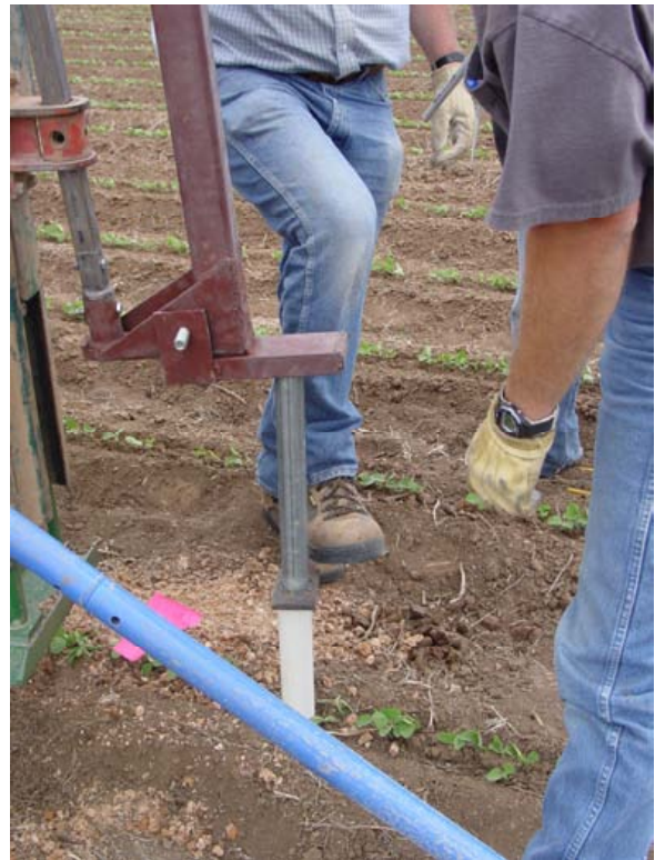
Figure 5.5. Installing access tubes, clockwise from upper left: (1) the Sentek driving head; (2) a steel tube used in conjunction with the hydraulic push machine; the long steel tube prevents the plastic tube from bending. (3) and (4) Using the hydraulic push machine with another steel tube to finish pushing the tube in after the tripod has been removed.
