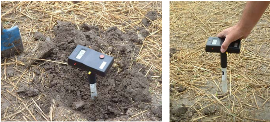
Figure 8.2. (Left) Newly installed tensiometer with Tensimeter (Marthaler et al., 1983) being used to sense the tension through a rubber septum that closes the top of the tensiometer tube. (Right) Example of reading a previously installed tensiometer. The black tube of the Tensimeter is pushed downward over the top of the white tube of the tensiometer, causing a needle inside the black tube to penetrate the rubber septum.
