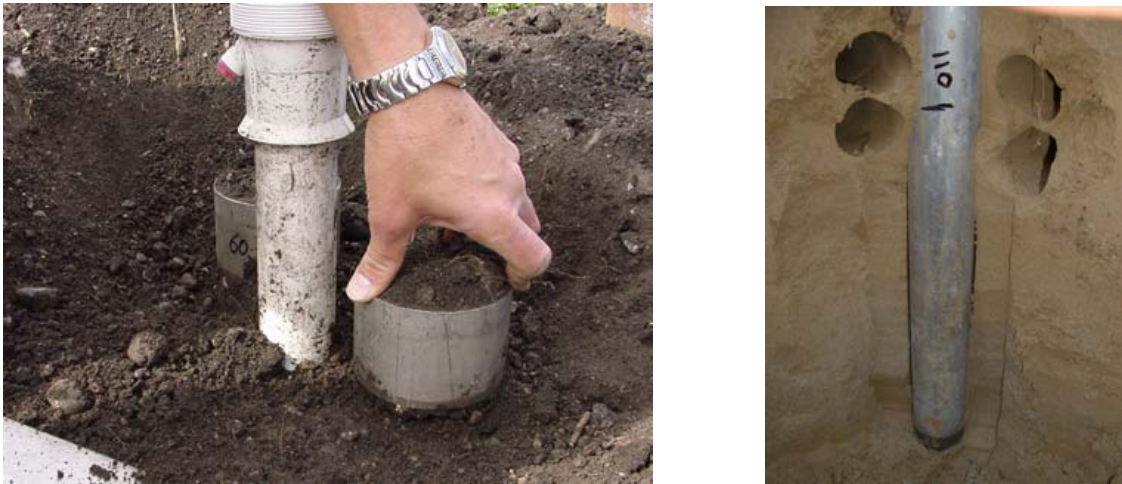
Figure 1.3. Examples of taking volumetric samples as close to the sensor position as possible. On the left is the plastic access tube for a capacitance sensor. Bevelled cylinders have been inserted into the soil as close to the tube as possible and to a depth that centres the sample on the depth of reading of the sensor. A third cylinder has already been removed, and the other two have been excavated. On the right is an aluminium access tube for a NMM. Four volumetric samples have already been extracted from as close to the access tube as possible. In this case, two were extracted from just above the 110 cm reading depth, and two from just below this depth, and all were taken horizontally.
