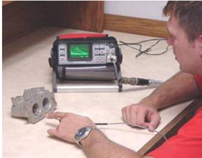
FIG. 8. A small surface probe is scanned over the part surface in an attempt to detect a crack.
