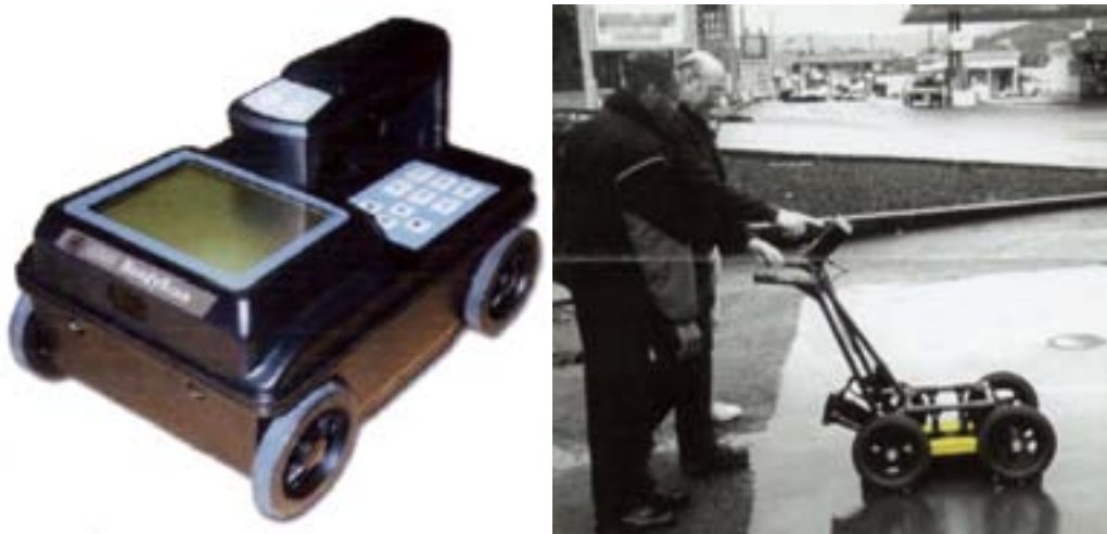
FIG. 30. Ground Penetrating Radars for detection of delaminations, cracks, voids, and reinforcing steel bars in concrete structures.
