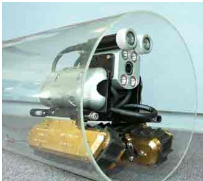
FIG. 21. Robotic crawler for remote visual inspection to assess the condition of the pipe.
