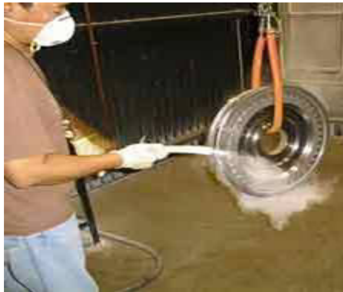
FIG. 3. Preparation of the object for the liquid penetrant inspection.
