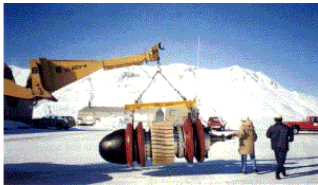
FIG. 19. Ultrasonic testing pig used for corrosion inspection of buried oil pipeline.
