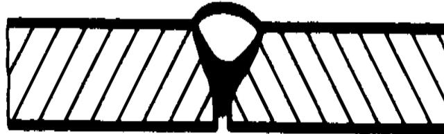
*FIG. 10. Incomplete root penetration.*
