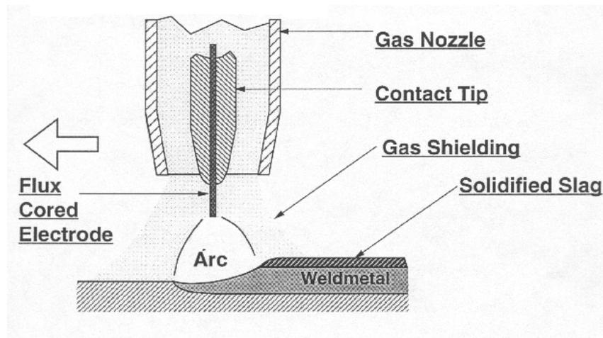
FIG. 5. Schematic diagram of FCAW.
