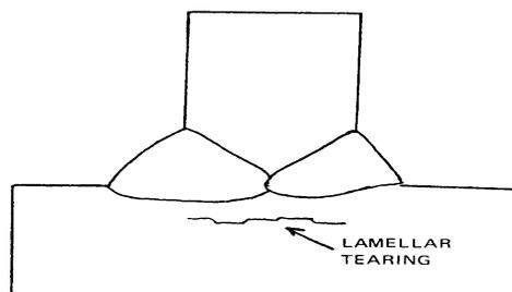
*FIG. 18. Lamellar tearing.*
