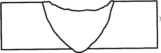
FIG. 15. Surface concavity.
