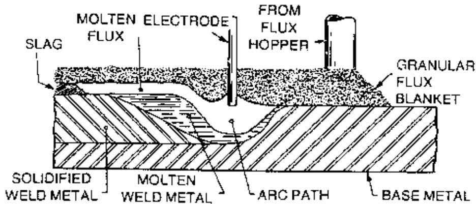
FIG. 6. Schematic diagram of SAW.
