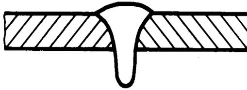
*FIG. 16. Excessive penetration.*
