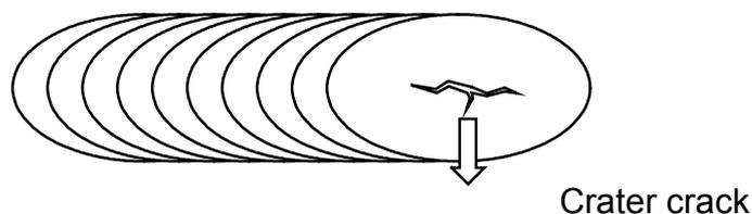
*FIG. 12. Crater crack.*
