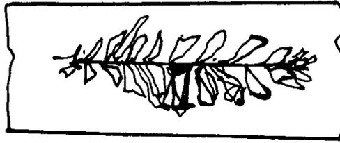
*FIG. 9. Piping in weld.*
