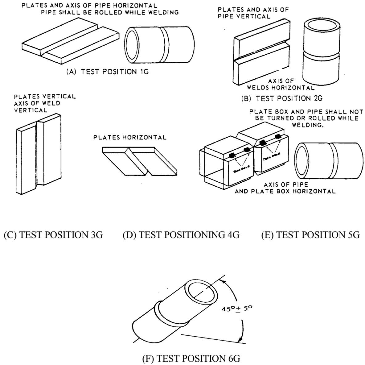
FIG. 2. Positions of plates and pipes for groove weld.
