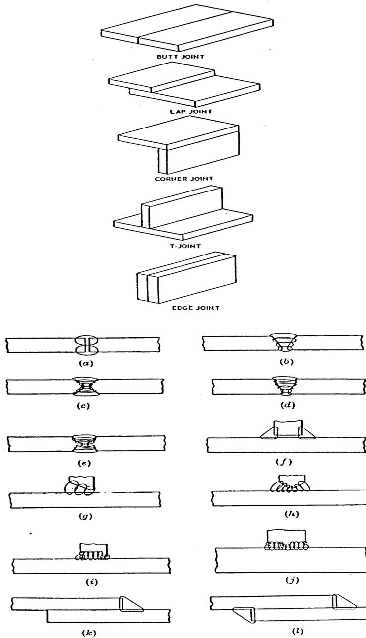
FIG. 1. Types of welding joints.
