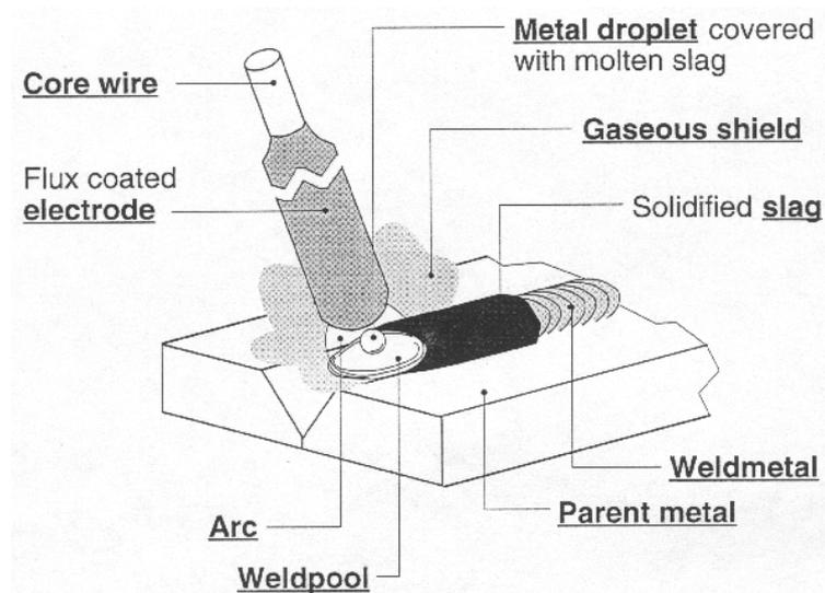
FIG. 3. Schematic diagram of MMAW.
