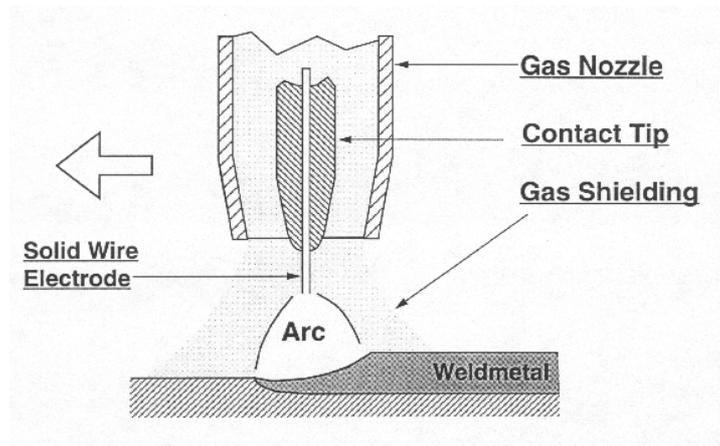
FIG. 4. Schematic diagram of GMAW.
