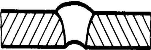
FIG. 14. Root concavity.
