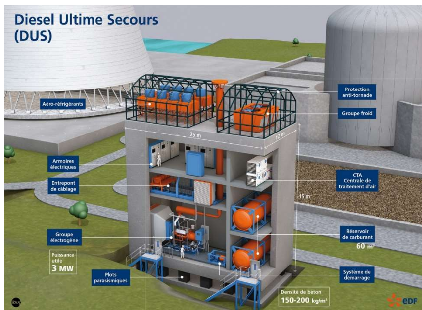
Fig. 4. Installation of a diesel of ultimate relief (reproduced with permission courtesy of EDF)
