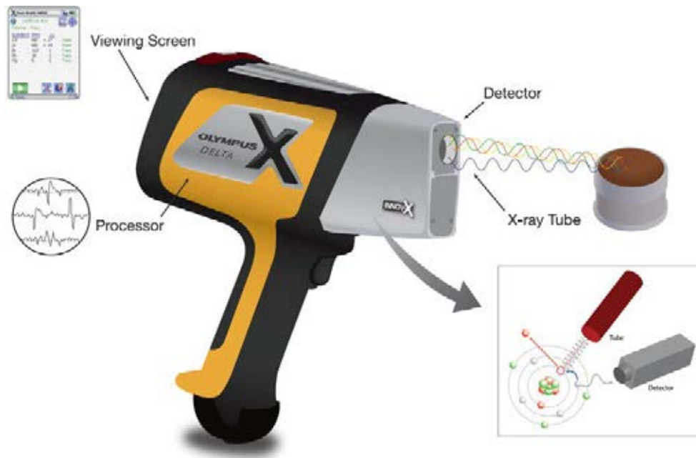
FIG. 16. X ray fluorescence tool for positive material identification (reproduced courtesy of Olympus-NDT with permission).
