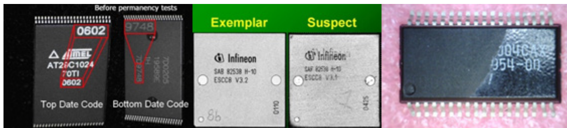
FIG. 37. Electronic counterfeit examples (left: date code changes; centre: tampering detected via acoustic microscope; right: blacktopping detected by heated solvent test) (reproduced courtesy of SMT Corp.).
