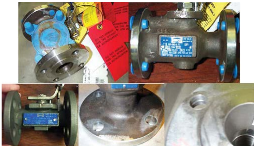
Note: Clamp marks and different rivet sizes are evident in the figure.
