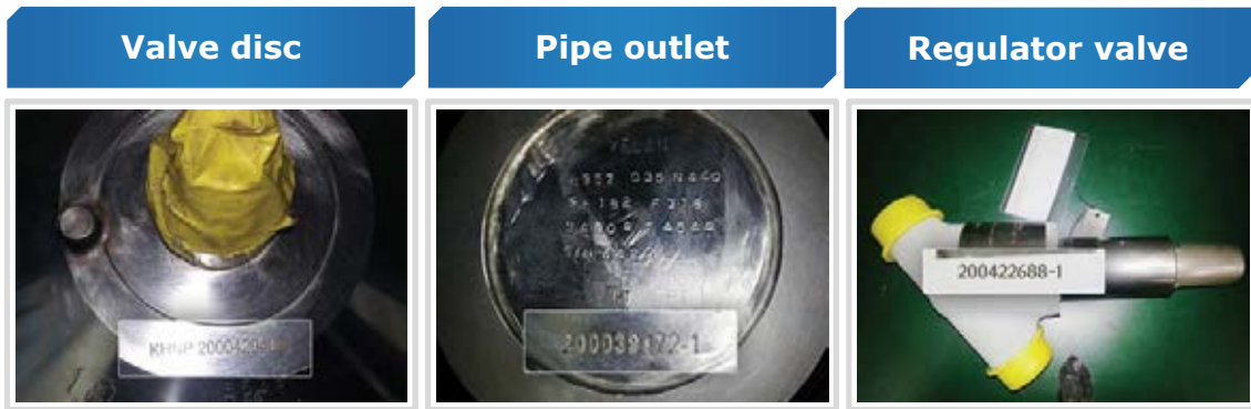
FIG. 20. Laser engraving (courtesy of Korea Hydro & Nuclear Power).
