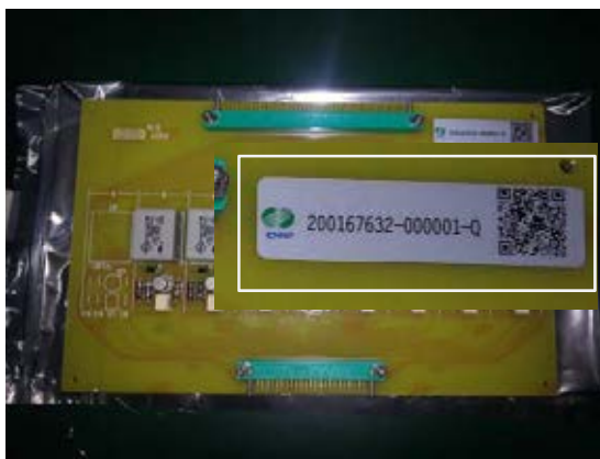
FIG. 21. Polyester film radiofrequency identification label with a quick read two dimensional barcode (courtesy of Korea Hydro & Nuclear Power).
