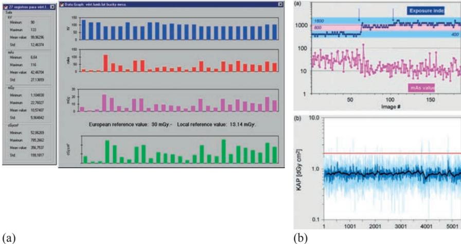
FIG. 3. (a) An on-line patient dose monitoring system developed for computed radiography auditing [13]. (b) Top: anteroposterior lumbar spine radiograph exposure. Small alterations of the automated exposure control are indicated (arrows). Bottom: automated assessment of the kerma area product in posteroanterior chest radiographs. The majority of exposures are below the diagnostic reference level (red line) [3].
