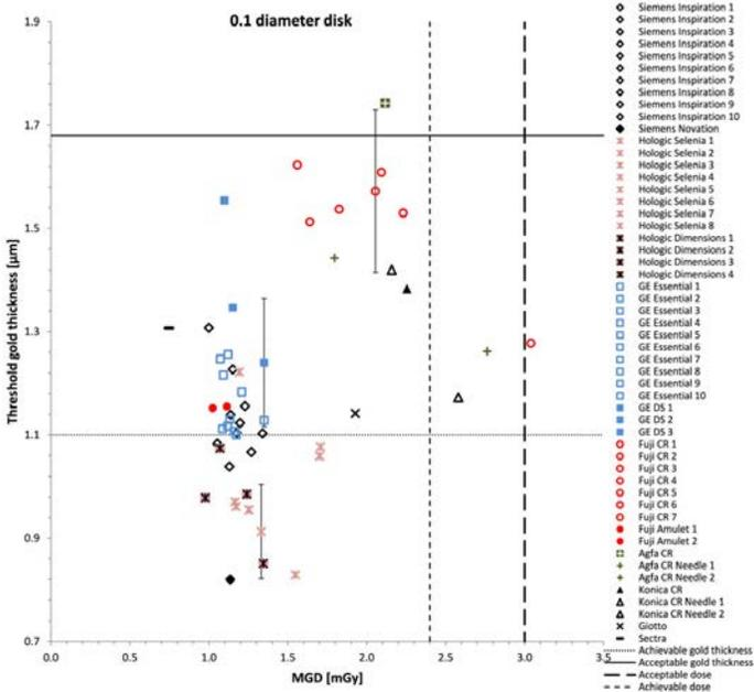
FIG. 4. Combined visualization of mean glandular dose (MGD) and threshold gold thickness to detect the 0.1 mm disc for a large set of systems [11].
