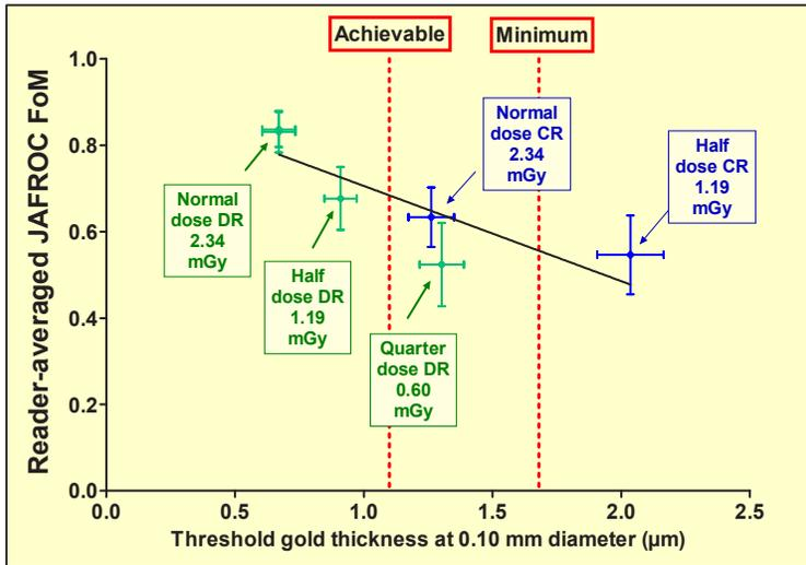
FIG. 5. Link between the threshold gold thickness retrieved from analysis of CDMAM images for different system simulations and a performance parameter retrieved from human reading of images of a virtual clinical trial of corresponding X ray systems (courtesy of K. Young, OPTIMAM project).
