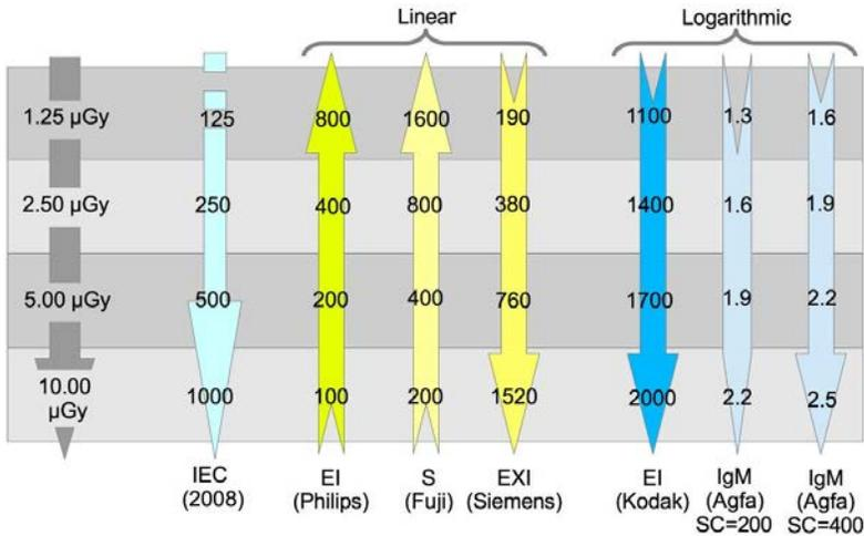
FIG. 1. A list of exposure indices terminology used by various digital systems and their relationship to traditional dose measure (in micrograys). In the second column, the proposal for an international standardization (International Electrotechnical Commission) is detailed [3].
