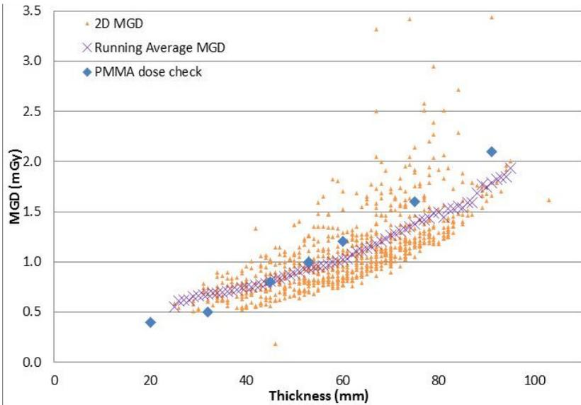
FIG. 1. Distribution of mean glandular doses (MGDs) for a large dose data survey using automated tools for data collection and MGD calculation assuming a thickness dependent glandularity distribution as in Ref. [5] for the age group 50–69 years. MGD estimates from acquisitions on polymethyl methacrylate (PMMA) are also indicated.
