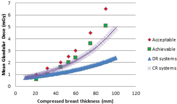
FIG. 3. Mean glandular dose (MGD) as a function of compressed breast thickness for a large patient dose sample examined with direct radiography (DR) and computed radiography (CR) technology, respectively. The achievable and acceptable dose levels for polymethyl methacrylate (PMMA) acquisitions (all of them corresponding to a specific compressed breast thickness) are plotted on top of this graph.
