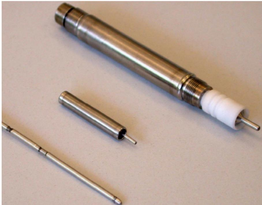
FIG. 12.1. Examples of fission chambers with different diameters for the measurement of neutron flux (courtesy of the French Alternative Energies and Atomic Energy Commission).
