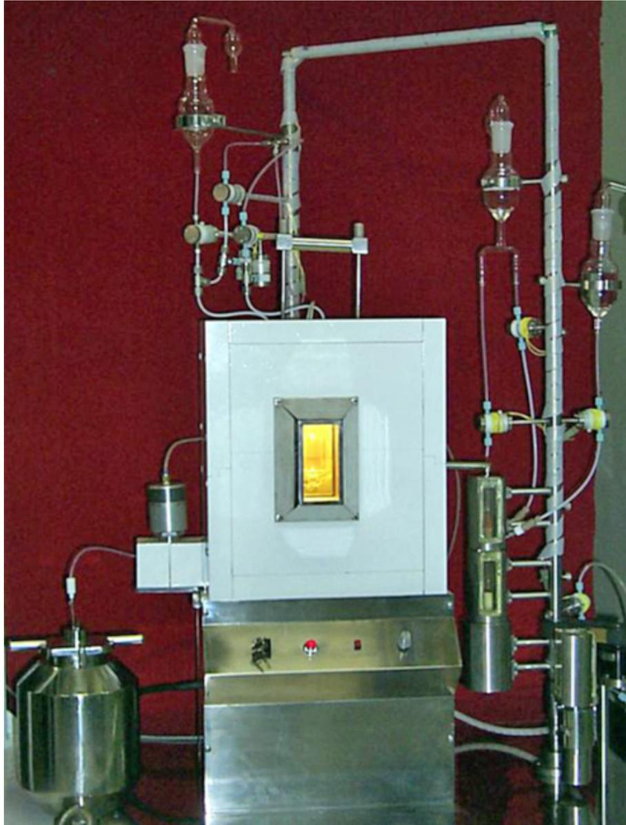
FIG. 5.5. Technetium-99m solvent extraction unit (courtesy of the Korea Atomic Energy Research Institute).
