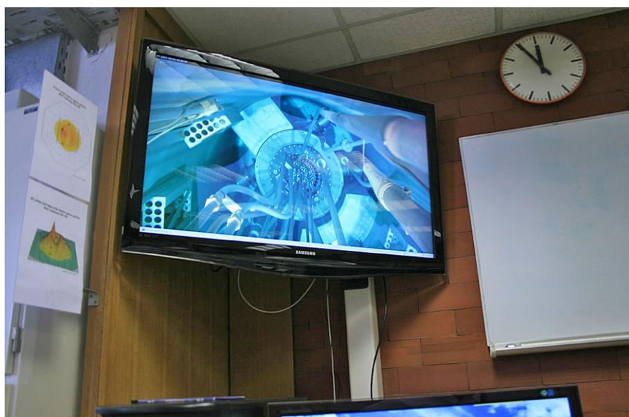
FIG. 2.4. Remote view of the TRIGA reactor core displayed on a high definition camera system used for reactor operator training (courtesy of the Jožef Stefan Institute).
