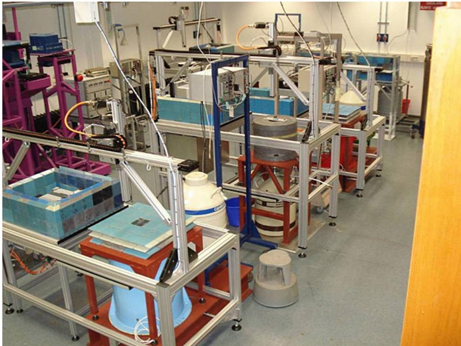
FIG. 3.5. Automatic sample changers in the laboratory for instrumental neutron activation analysis (courtesy of Delft University of Technology).
