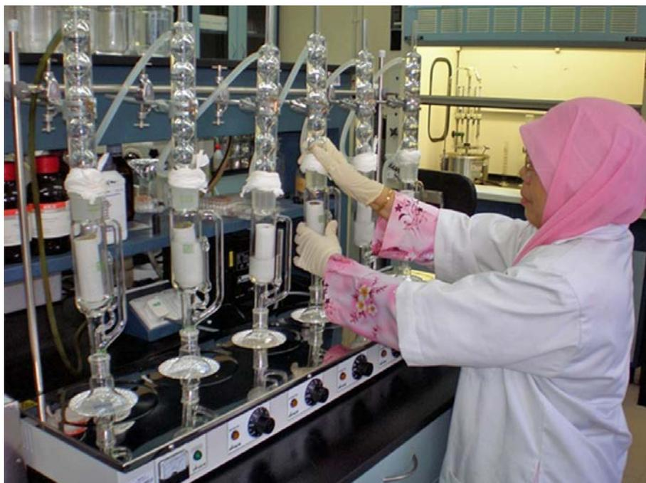
FIG. 3.1. Sample preparation for instrumental neutron activation analysis (courtesy of the Malaysian Nuclear Agency).
