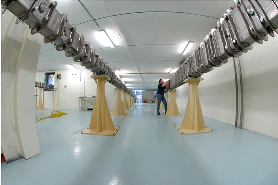
FIG. 9.5. Thermal neutron beam guide tubes at the 20 MW OPAL research reactor (courtesy of ANSTO).
