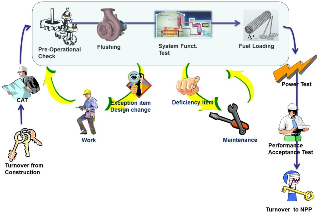
FIG. 25. Typical turnover process to commissioning and operation.
