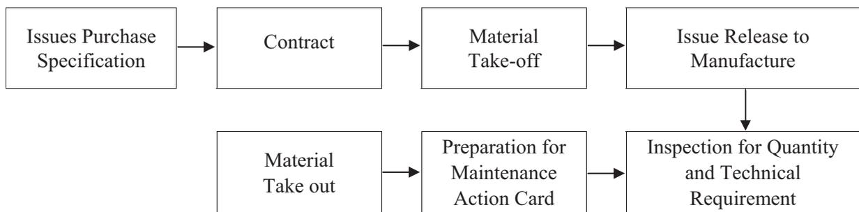
FIG. VI-4. General process for material control.
