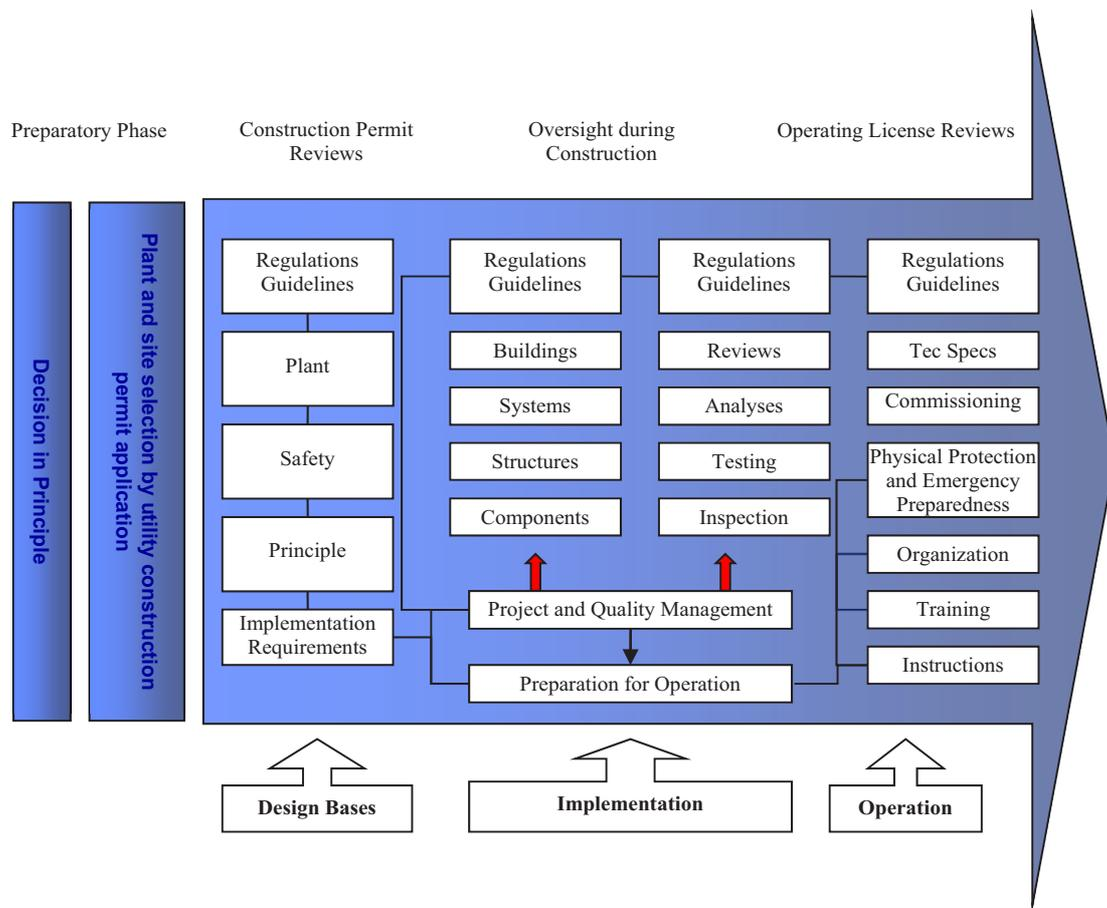
FIG. 21. Three steps of construction inspection programme [13].
