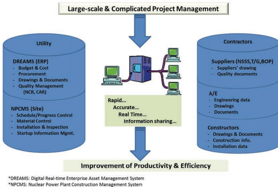
FIG. 6. Example of computerized information control system.
