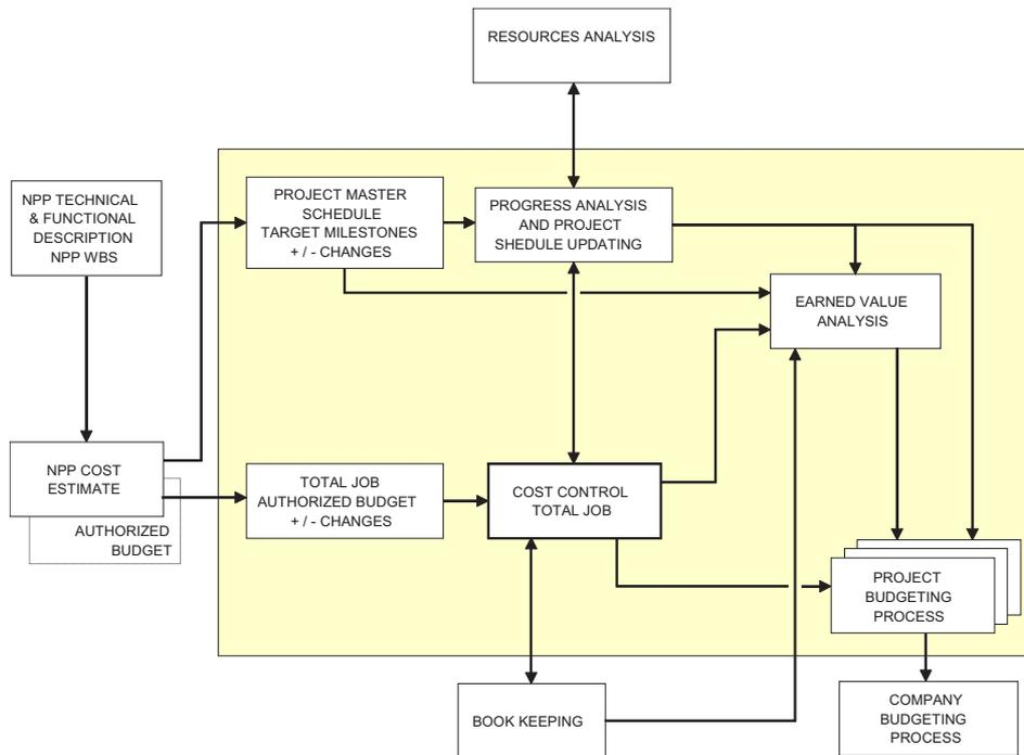
FIG. IX-3. The macro flowchart of the project planning and control.
