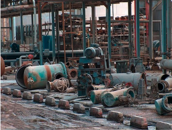
FIG. 2. NORM contaminated items in storage prior to cleaning or disposal.
