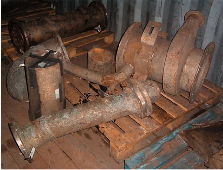
*FIG. 4. Objects contaminated with NORM.*
