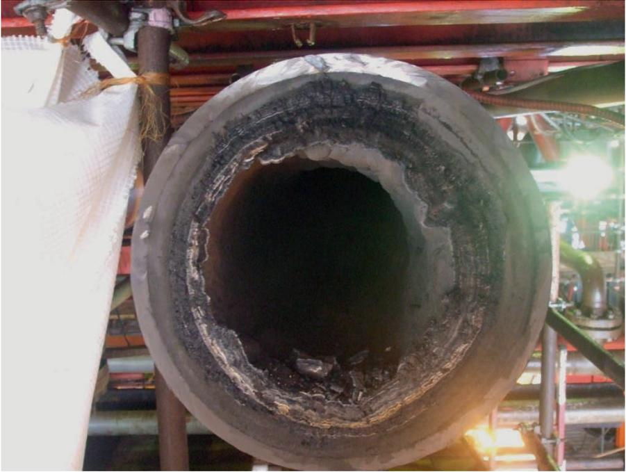
FIG.1. NORM contaminated pipe.
