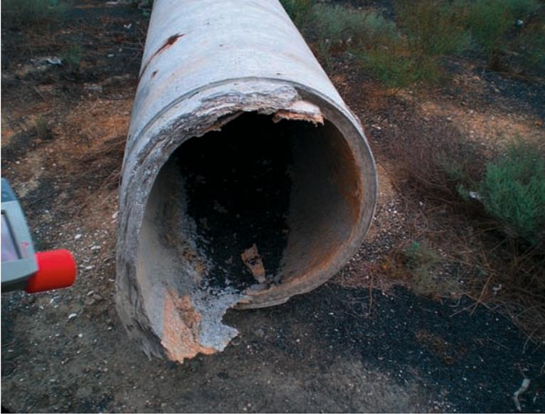
*FIG. 5. Asbestos cement water pipe with radium scale and radioactive coal dust residues.*
