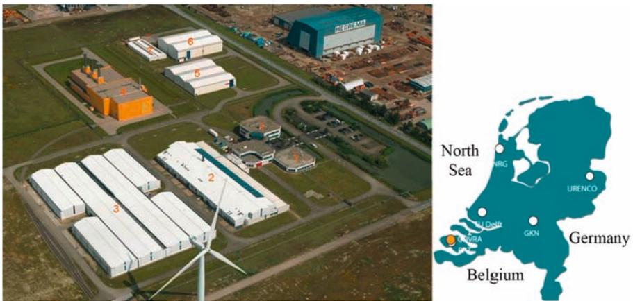
*FIG. 1. The COVRA site. (1) Office building and exhibition centre; (2) Building for the treatment of low and medium level waste (AVG); (3) Storage building for conditioned low and medium level waste (LOG); (4) Storage building for high level waste (HABOG); (5) Storage building for low level material from the enrichment industry (VOG); (6) Storage building for low level NORM waste from the ore processing industry (COG); (7) Storage building for scrap material (SOG).*
