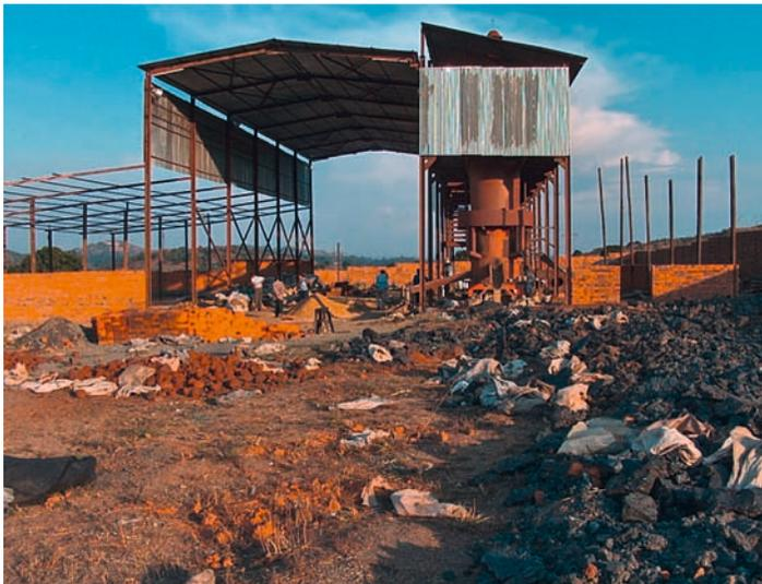
*FIG. 4. Artisanal copper smelter; at right, slag spread as fill for future building foundations.*
