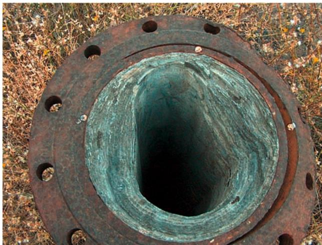
*FIG. 3. Uranium process residues in scrap pipework.*
