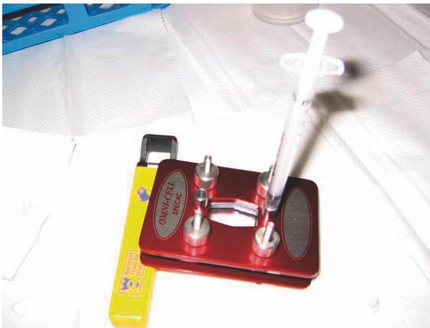
FIG. 21. FTIR cell with a 1 mL syringe in the filling port. The cell is raised at one end by propping on any suitable object, such as a pencil.
