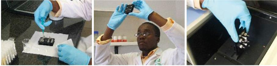
FIG. 22. Procedure for filling the cell. The cell should be filled using a 1 mL syringe, checked for bubbles by holding the cell up to a light, and placed in the sample chamber of the FTIR.
