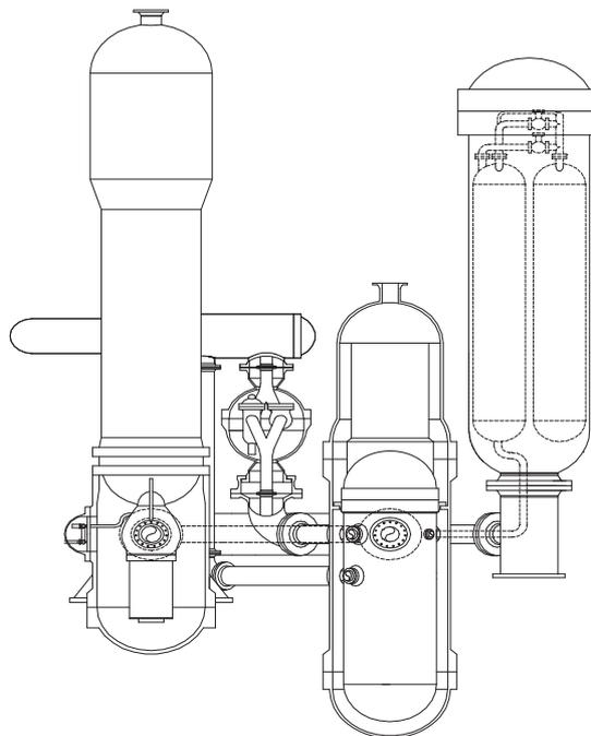
FIG. 5. Layout of the MARS reactor with pressurized containment for primary loop protection.
