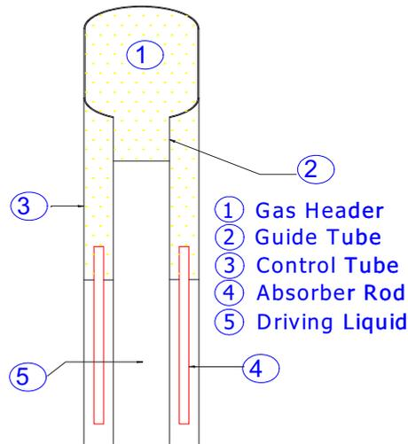
FIG. X-4. Schematic view of PPRS.
