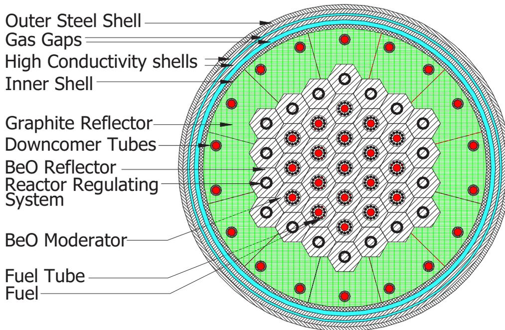
FIG. X-1. Cross-sectional layout of CHTR core.
