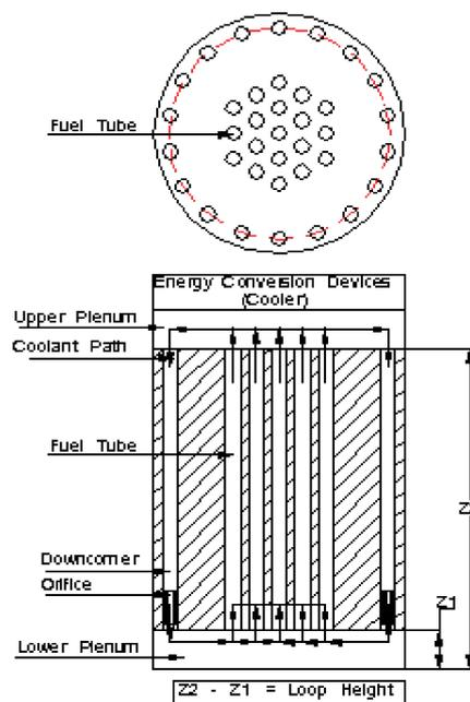
FIG. 11. Schematic view of CHTR primary circuit loop.
