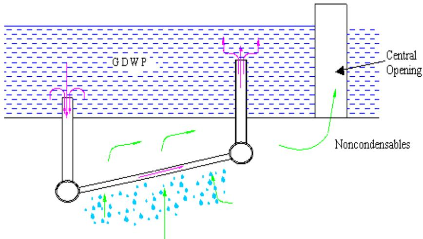
FIG. VI-5. Passive containment cooling system.
