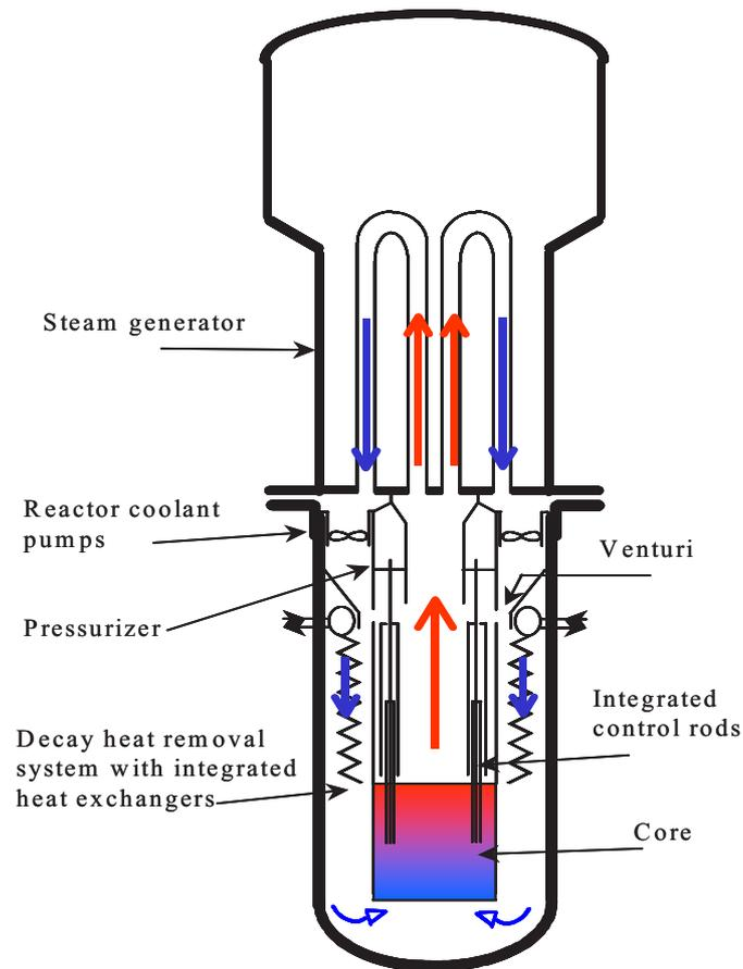
FIG. IV-2. Primary coolant system [IV-1].
