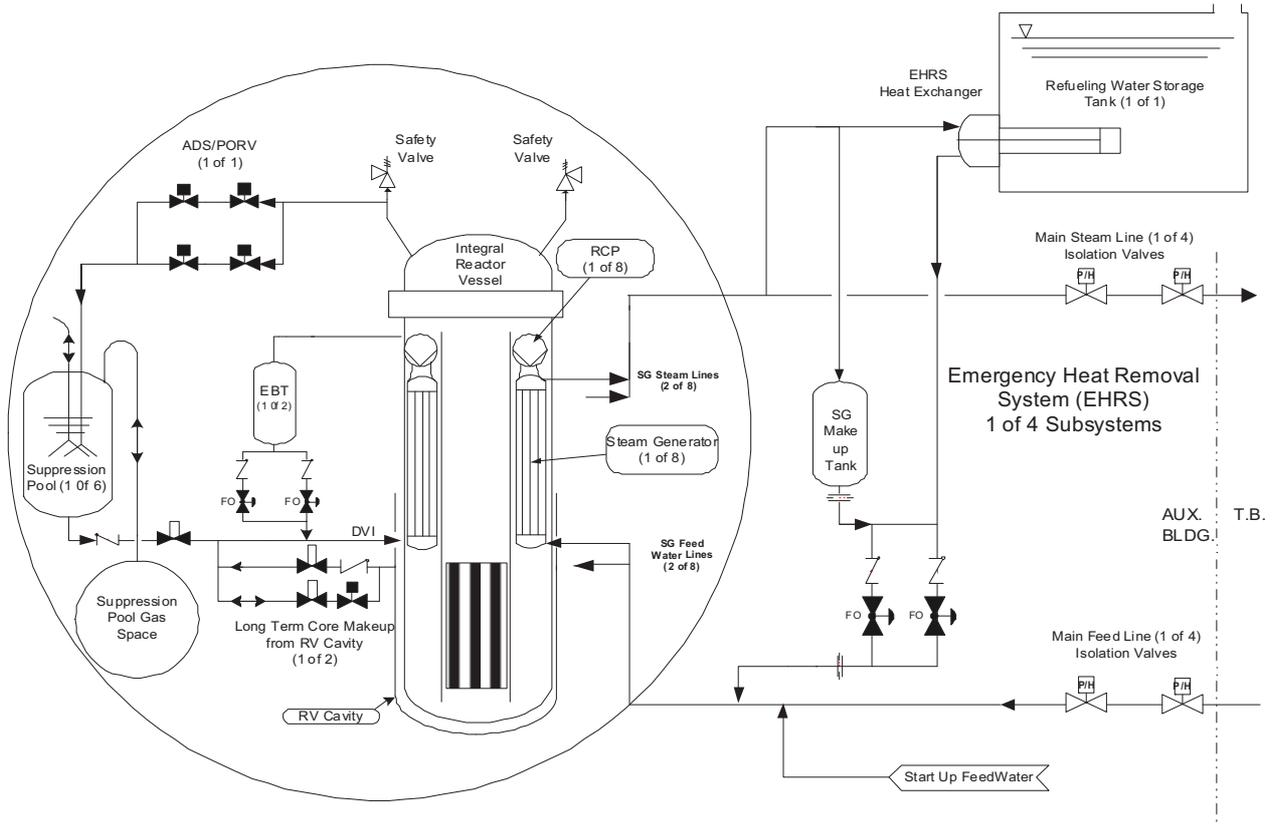
FIG. II-3. Schematic view of the IRIS's passive safety systems.
