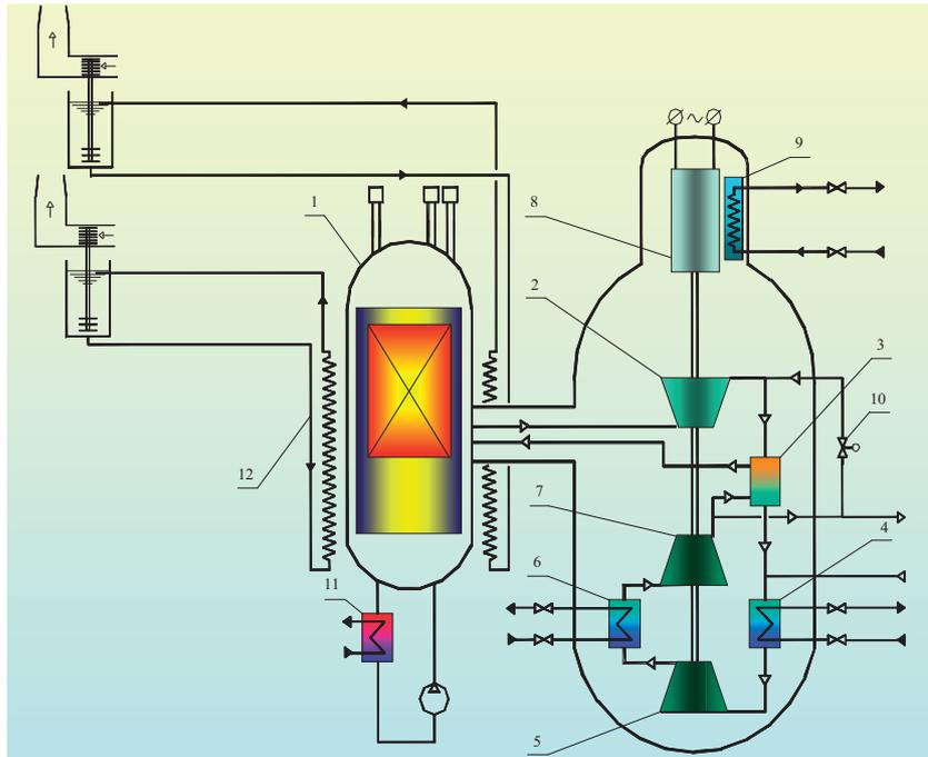
1–Reactor; 2–Turbine; 3–Recuperator; 4, 6–Pre-cooler and intercoolers;
