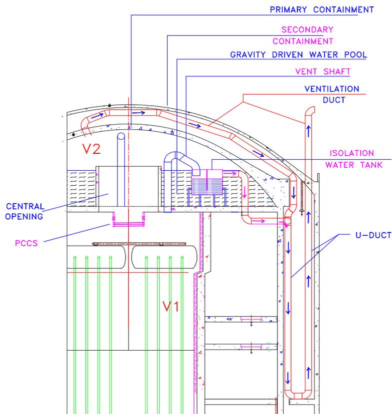
FIG. VI-6. Passive containment isolation system.
