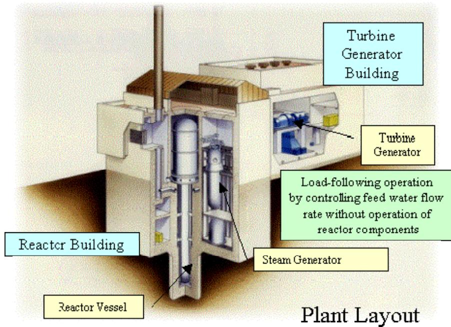
FIG. VIII-3. Reactor building of the 4S-LMR (1991 design) [VIII-1].
