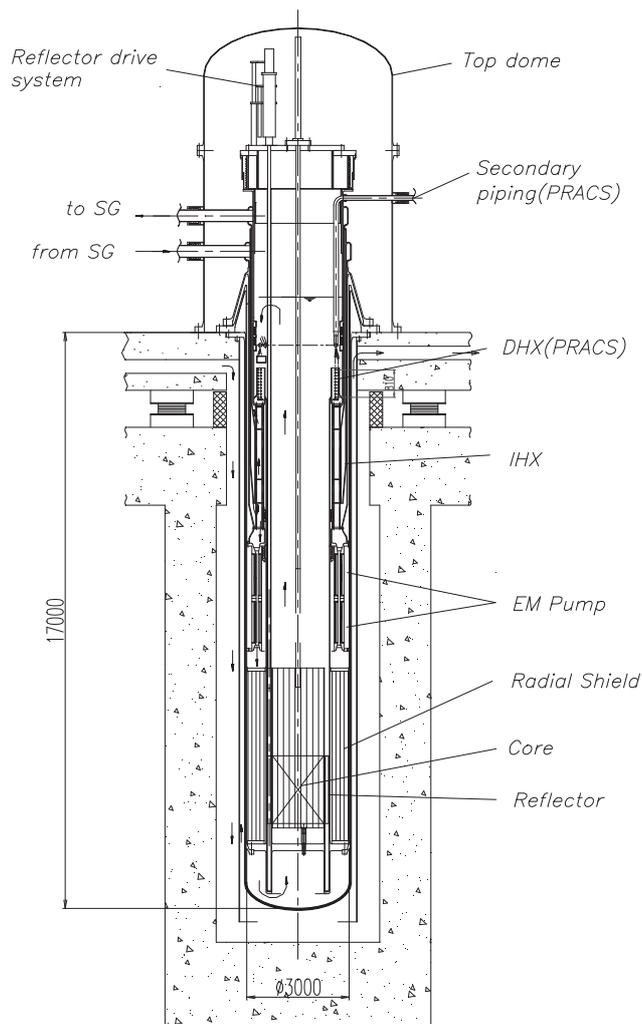
FIG. VIII-1. Vertical view of 4S-LMR layout.
