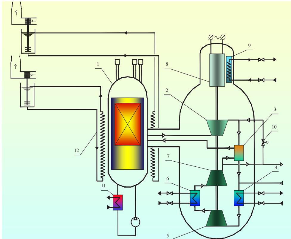
1–Reactor; 2–Turbine; 3–Recuperator; 4, 6–Pre-cooler and inter-cooler;
