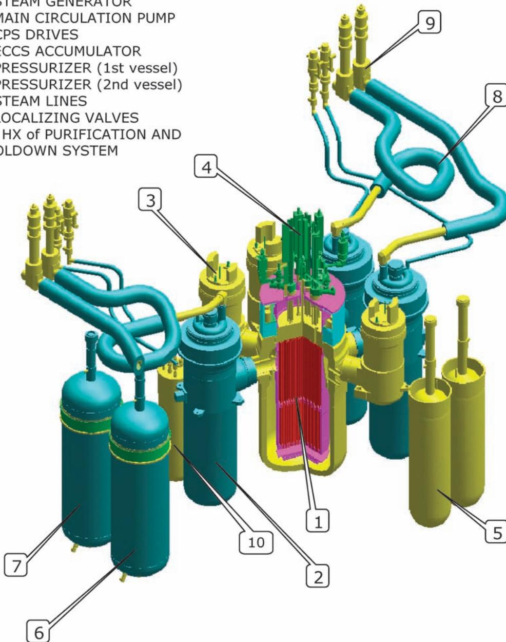
CPS - control and protection system    ECCS – emergency core cooling system    HX – heat exchanger
