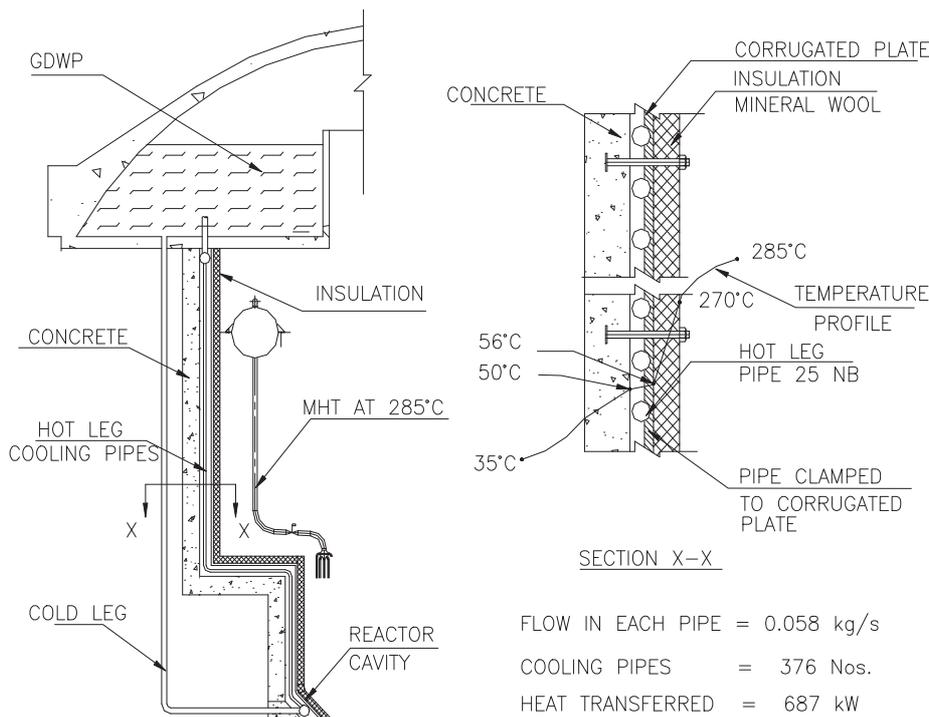
FIG. VI-8. Schematic view of passive concrete cooling system.
