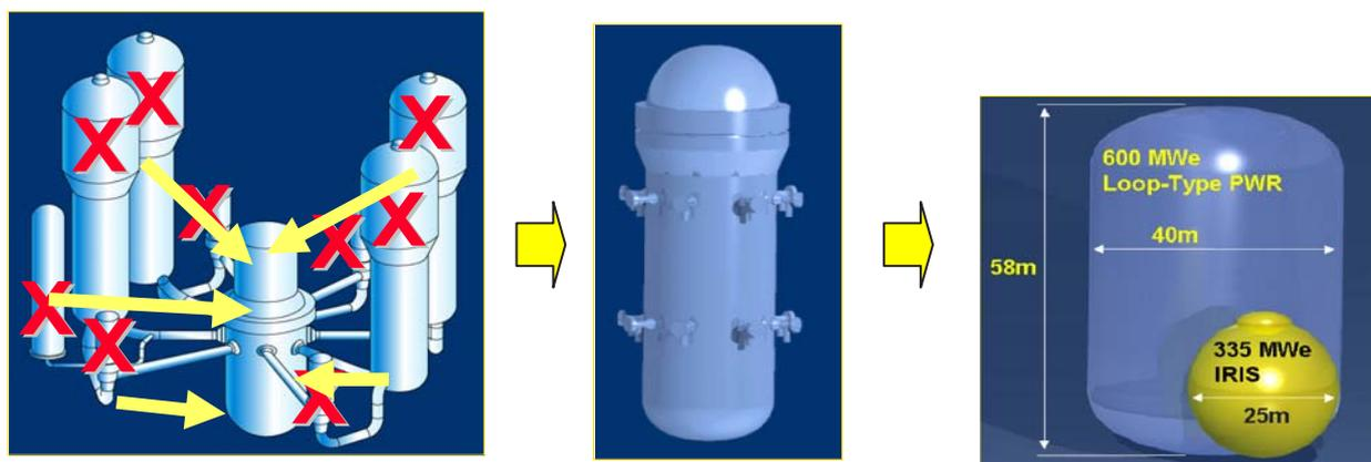
FIG. II-2. Compact integral layout of IRIS.
