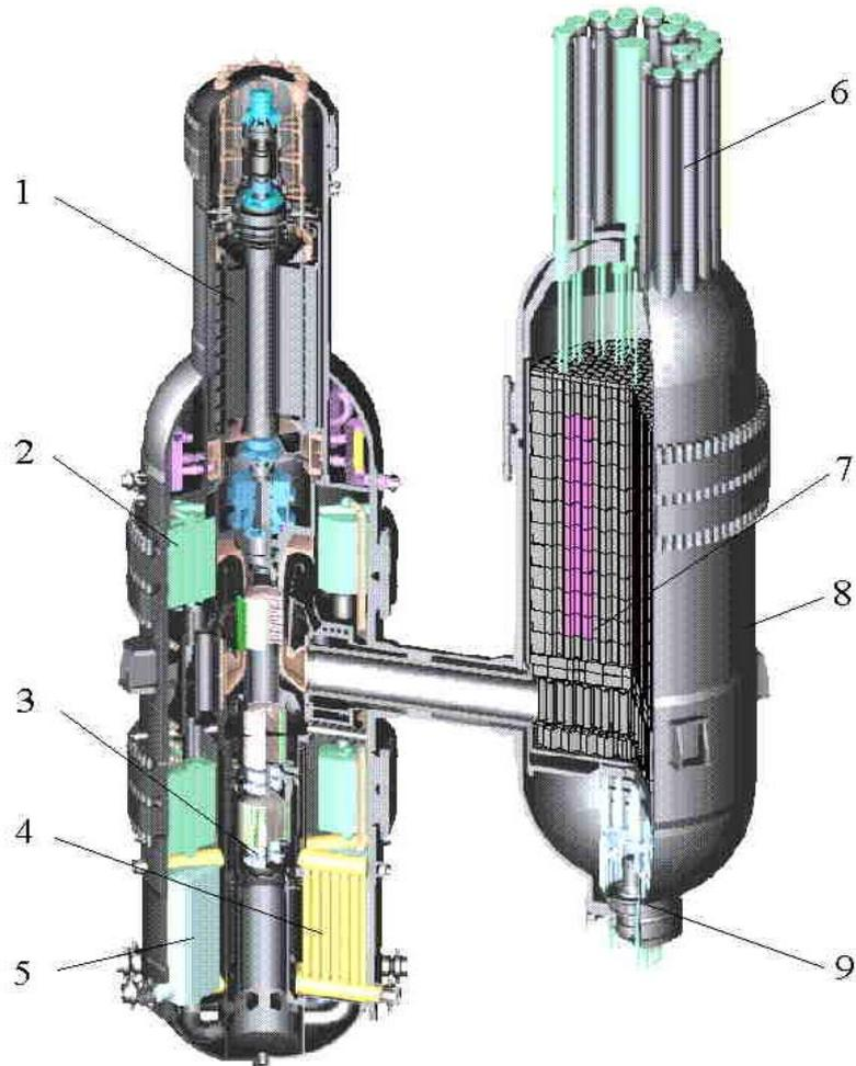
1 – Generator; 2 –Recuperator; 3 – Turbocompressor; 4 – Intercooler;
