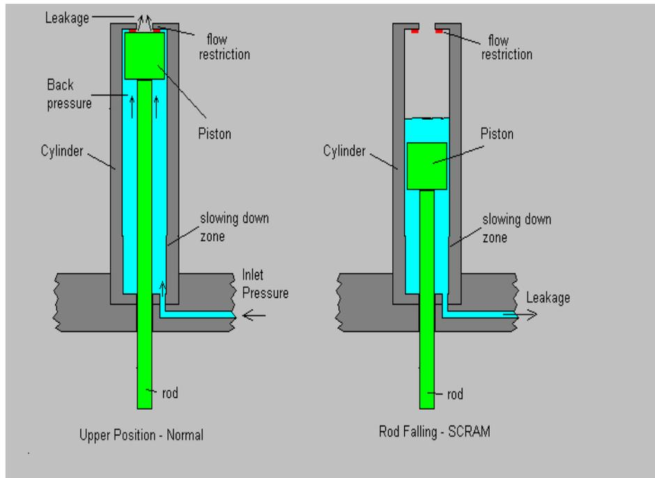
FIG. III-3. Simplified operating diagram of a hydraulic control rod drive (fast shutdown system).
