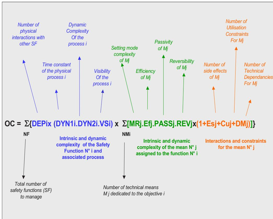
FIG. IV-4. Quantification of complexity — Operational complexity index (OC).
