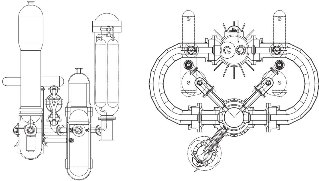
FIG. V-2. Pressurized containment for primary loop protection (CPP) [V-1].
