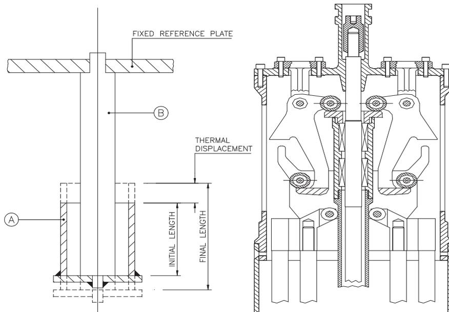
FIG. V-4. Operating scheme (left) and self-releasing head (right) of the ATSS [V-1].
