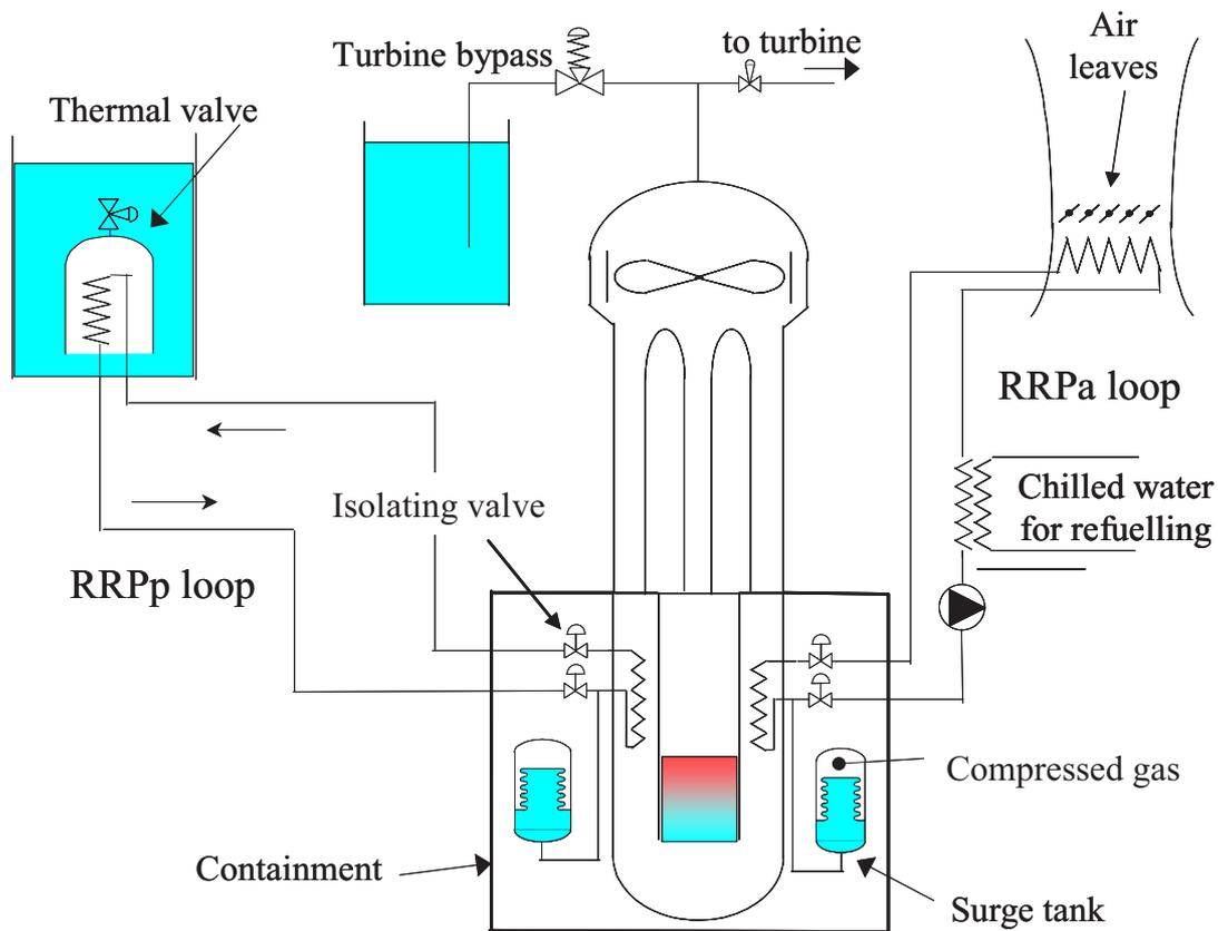
FIG. IV-6. Residual heat removal system on the primary circuit [IV-1].
