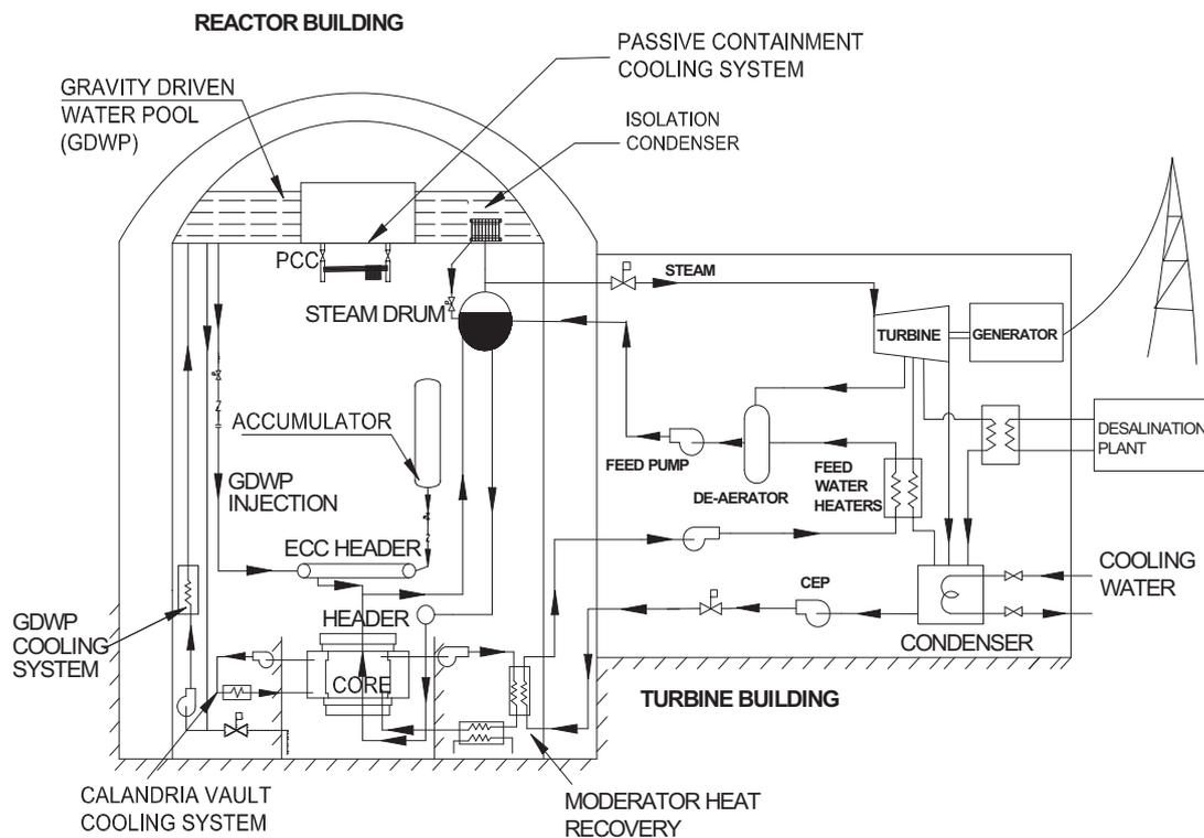
FIG. VI-1. General arrangement of AHWR [VI-1].
