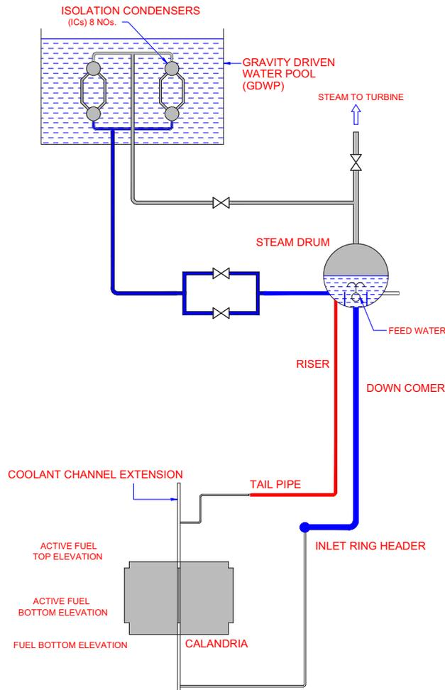
FIG. 7. Heat transport systems of AHWR.
