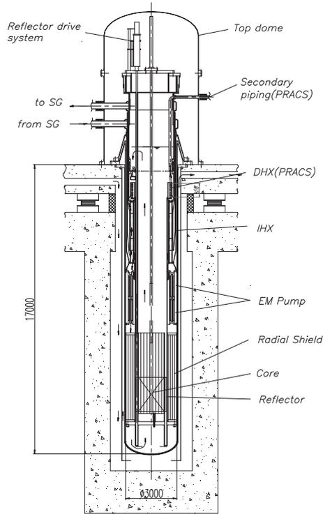
FIG. 9. Vertical view of the 4S-LMR layout.
