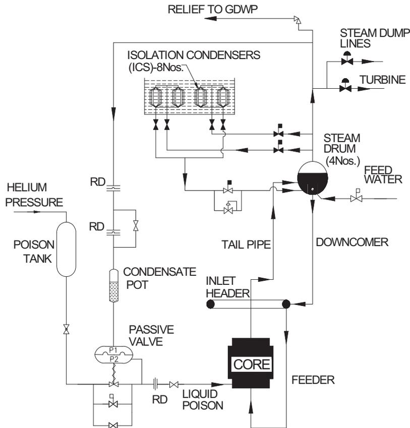
FIG. VI-7. Passive shutdown by MHT high pressure (RD is for rupture disc).
