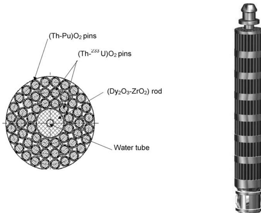
FIG. VI-2. AHWR fuel cluster arrangement.
