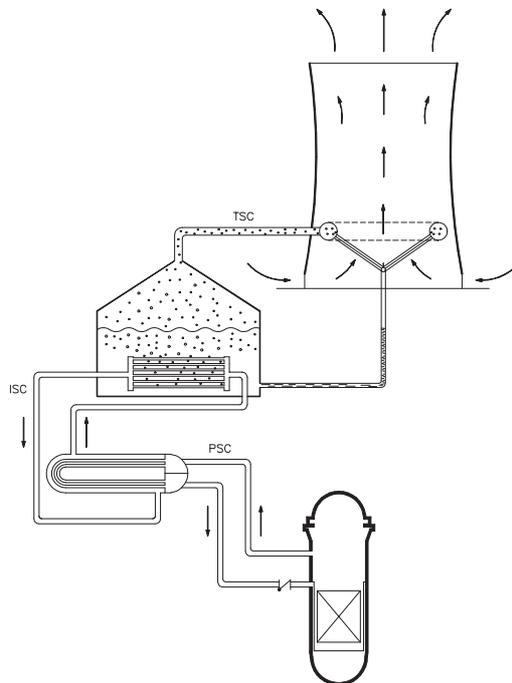
FIG. V-3. Scheme of the safety core cooling system (SCCS) [V-1].
