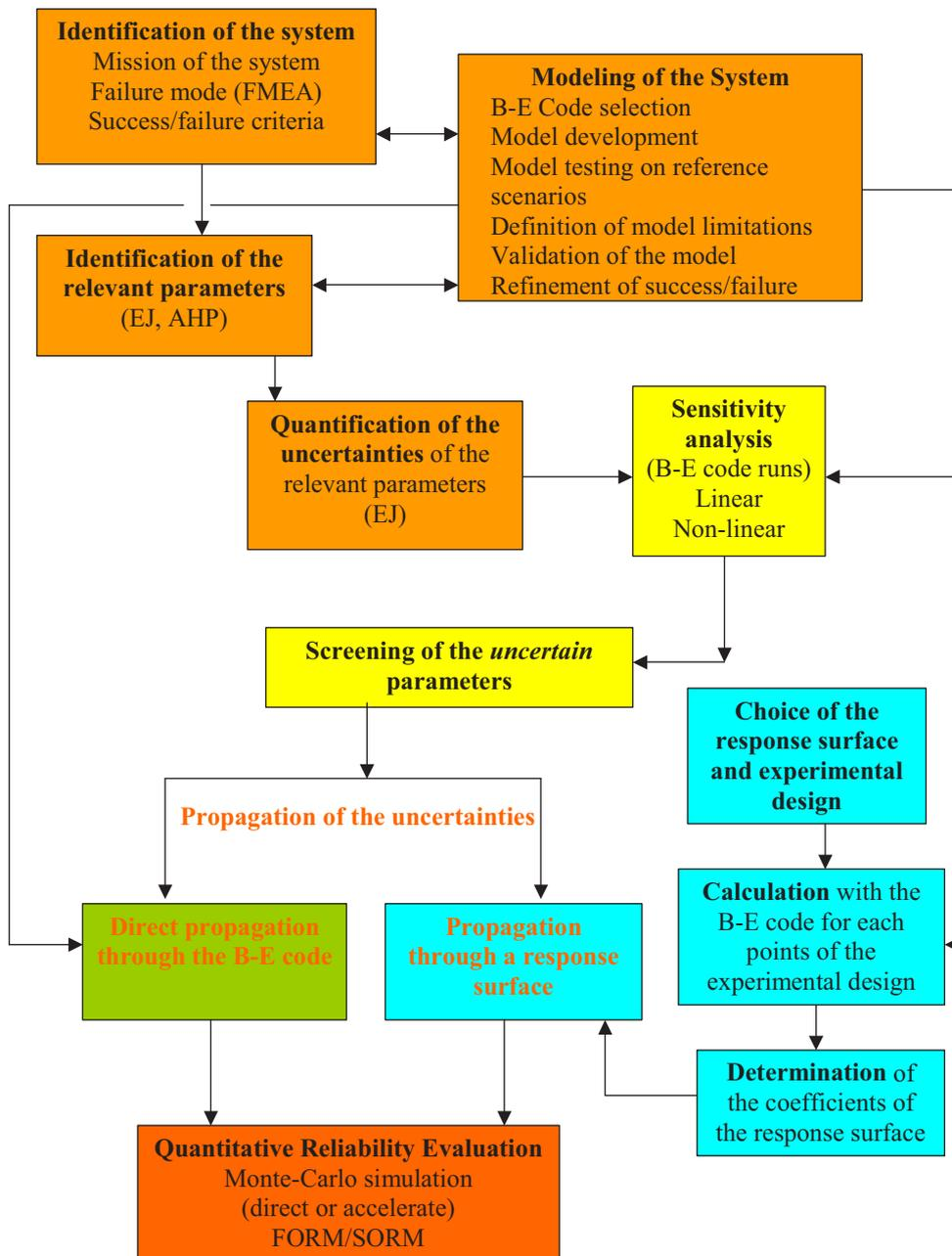
FIG. 1. Schematics of the RMPS methodology.
