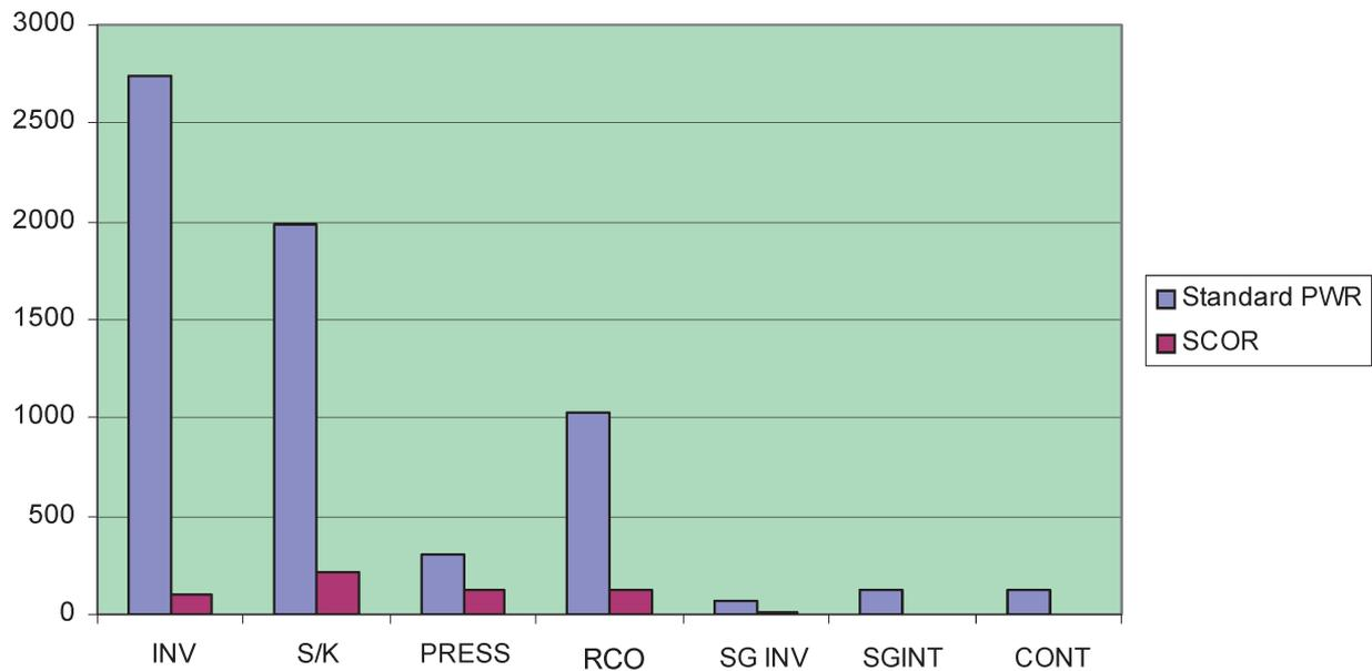
FIG. IV-5. Operational complexity vs. safety functions for the SCOR and a standard PWR [IV-1].
