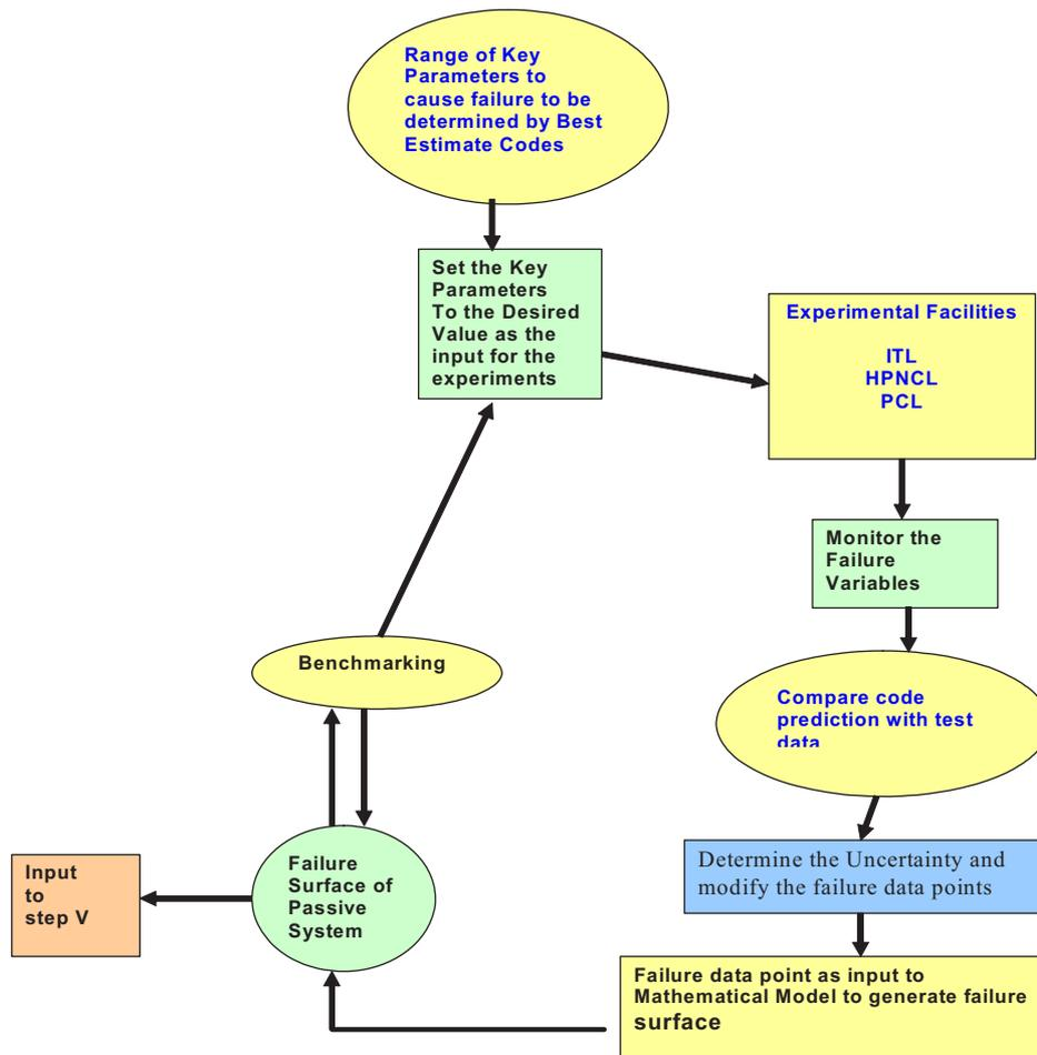
FIG. 3. APSRA methodology: programme flowchart for benchmarking of the failure surface based on experimental data.
