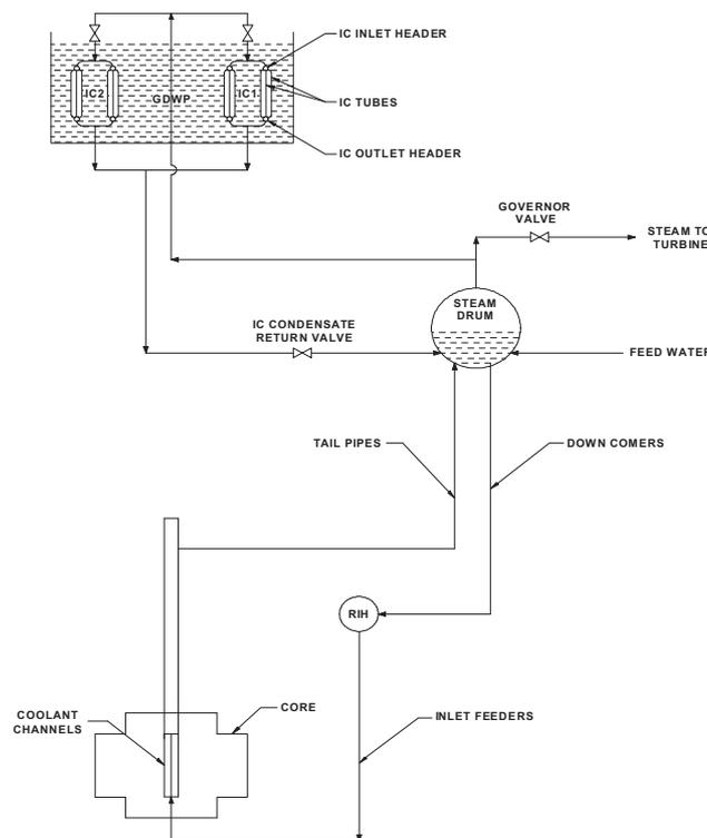
FIG. VI-3. MHT and decay heat removal system.
