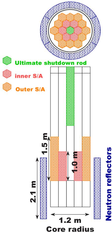
FIG. VIII-2. Core configuration of the 4S-LMR (Annex XV [VIII-1]).
