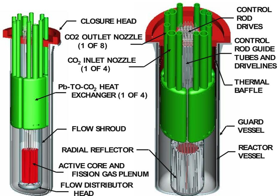
FIG. 10. General view of the SSTAR layout.
