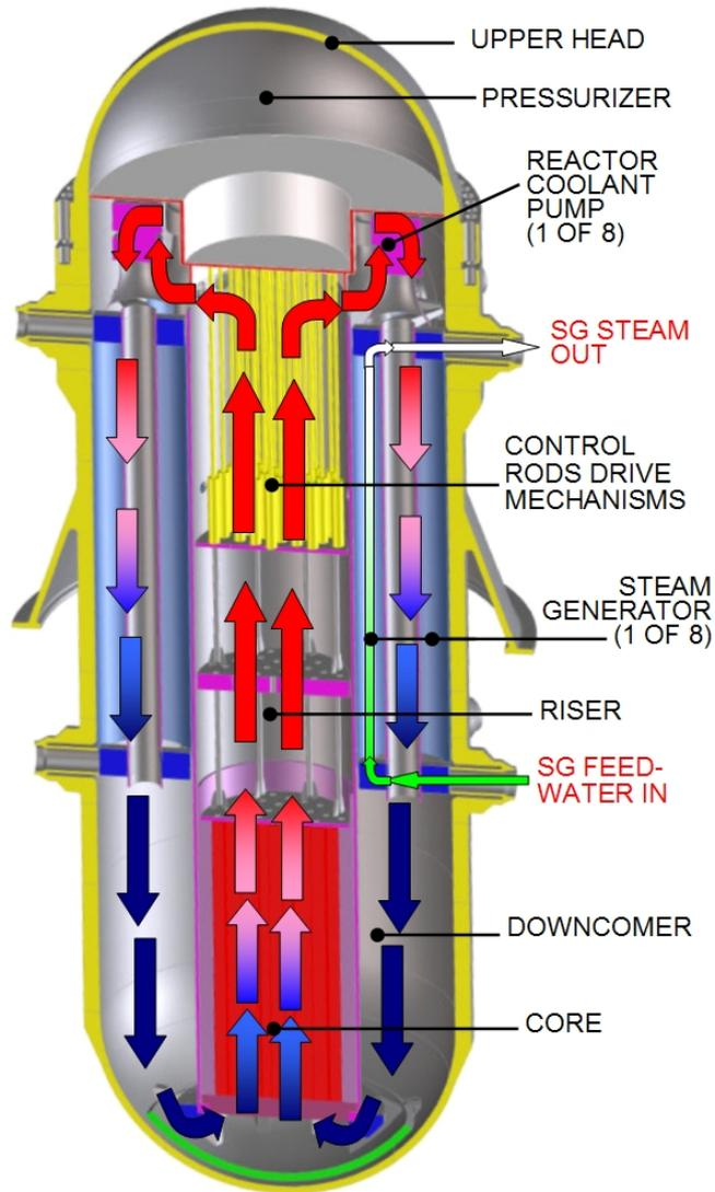
FIG. II-1. Integral primary system of IRIS.
