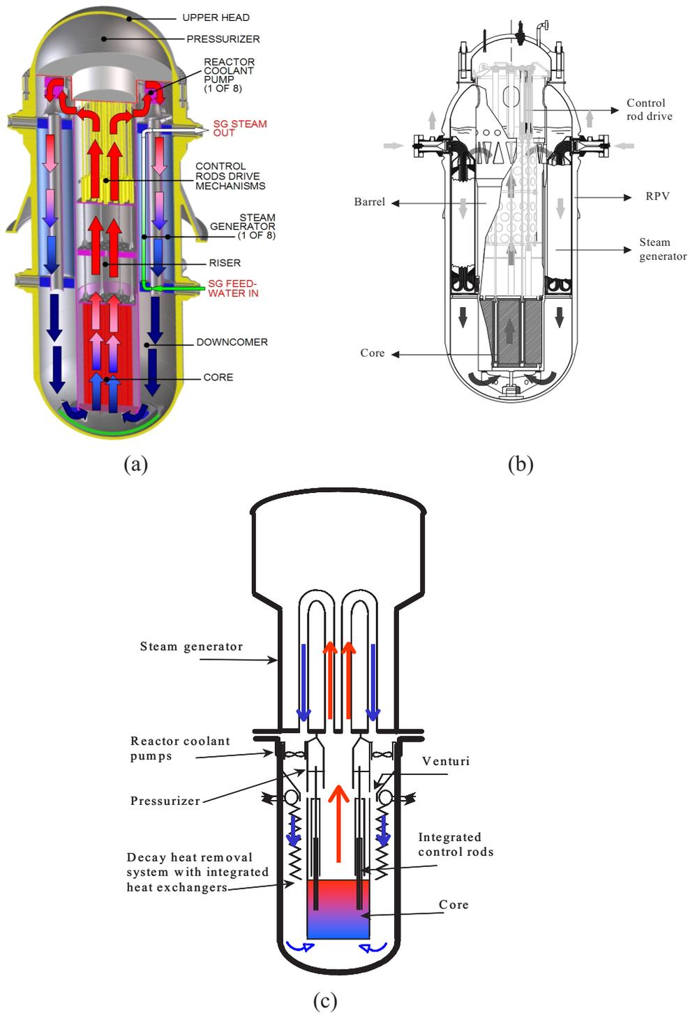
FIG. 3. Schematics of the primary coolant system for (a) IRIS; (b) CAREM-25; and (c) SCOR.
