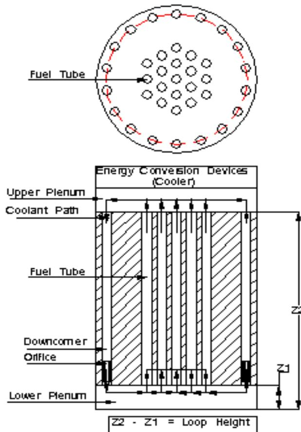
FIG. X-5. Schematic view of CHTR primary circuit loop.
