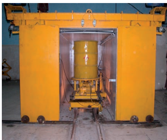
FIG. A-17. Waste assaying system operational at SWMF, Trombay.
