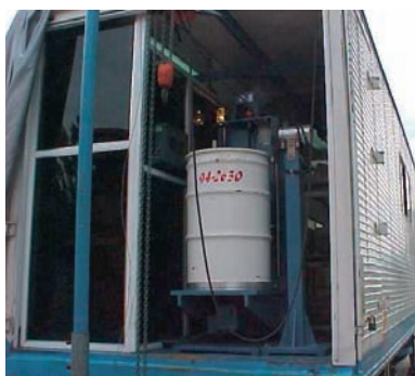
FIG. A-21. Portable automated waste assay system.
