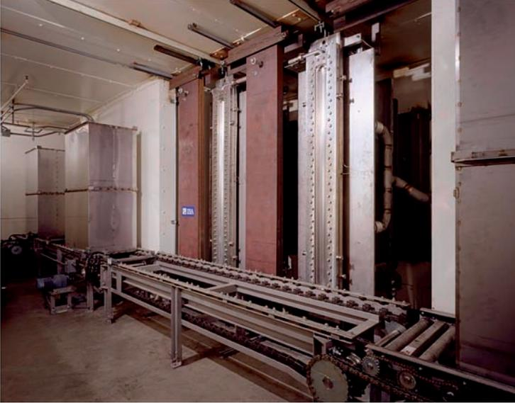
*FIG. 3.8. Product transport system in front of an electron beam scanner equipped with an X ray conversion target (courtesy of IBA, Belgium).*
