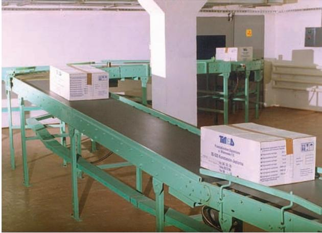
*FIG. 5.6. Belt conveyor in the Elektronika 10/10 accelerator facility.*
