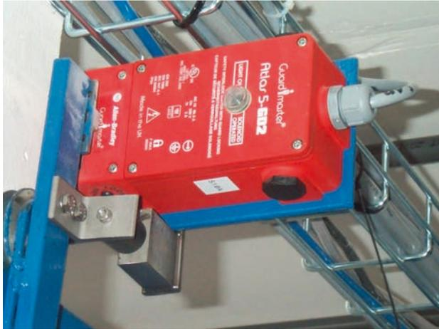
FIG. 10.2. Example of an EN 954-1 category 4 approved door switch with holding mechanism.
