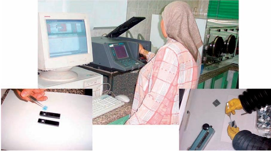
FIG. 7.6. A staff member at the NCRRT dosimetry laboratory measuring the optical absorbance of an irradiated film dosimeter in the spectrophotometer.
