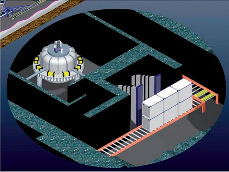
FIG. 3.7. An electron beam irradiator equipped with an X ray converter (courtesy of IBA, Belgium).
