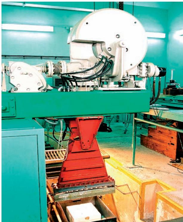
*FIG. 5.2. An LAE 13/9 electron accelerator has two output windows: (1) a horizontal beam output for R&D study; and (2) a vertical scanned beam output for radiation processing.*
