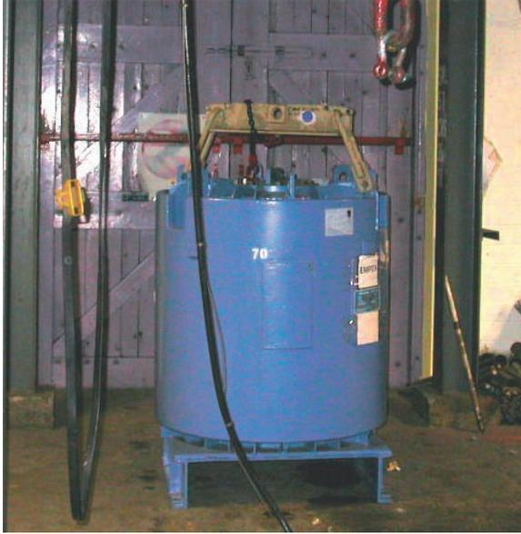
FIG. 10.1. Type B(U) packaging container for a  $^{60}\text{Co}$  source.
