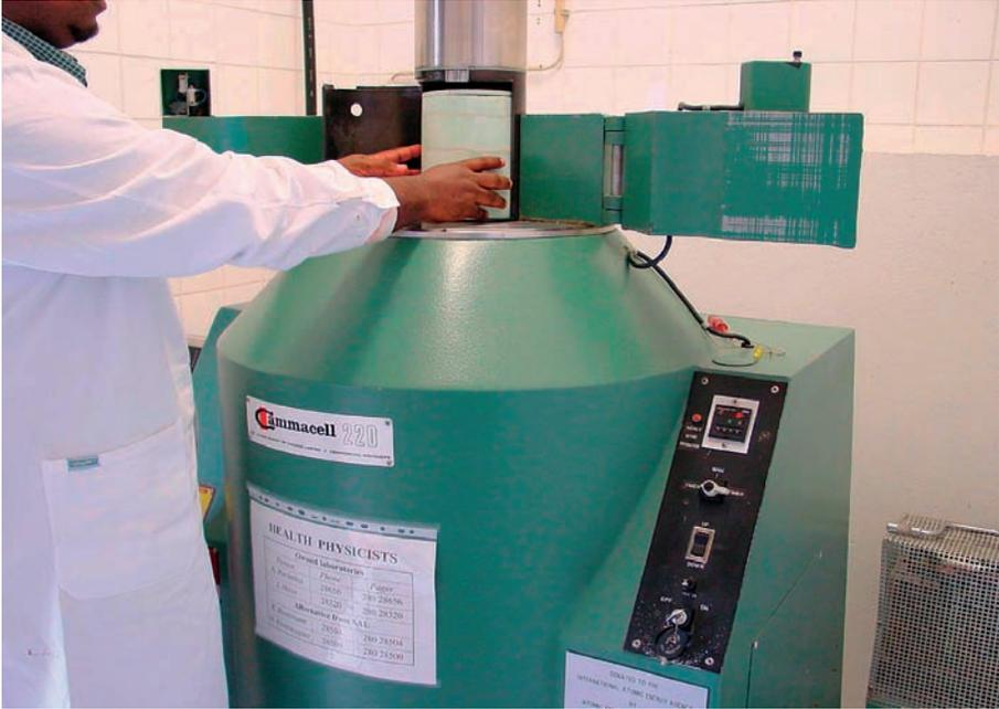
*FIG. 2.8. Self-contained dry storage gamma irradiator suitable for research and small scale irradiations. In preparation for irradiation, a sample holder is being placed in the irradiation chamber when it is in the loading position. Depending on the dose rate of the day, the timer on the control panel (bottom right) is set to give the desired dose.*
