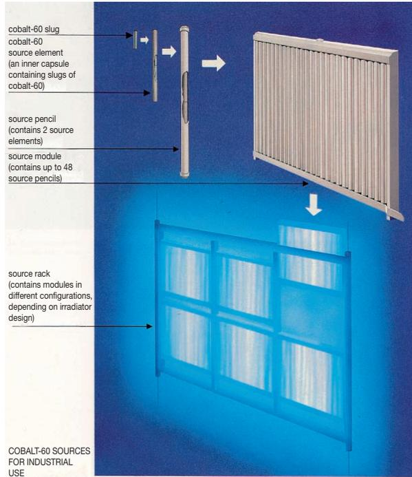
FIG. 2.3. Buildup of a typical cobalt source rack from slugs, pencils and module (courtesy of MDS Nordion, Canada).
