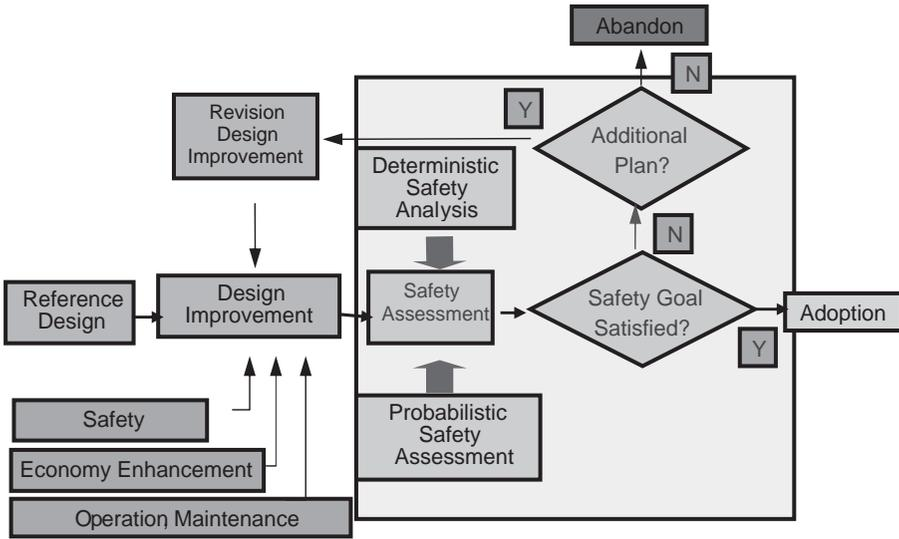
FIG. 6. Process for design improvement for enhancing safety.
