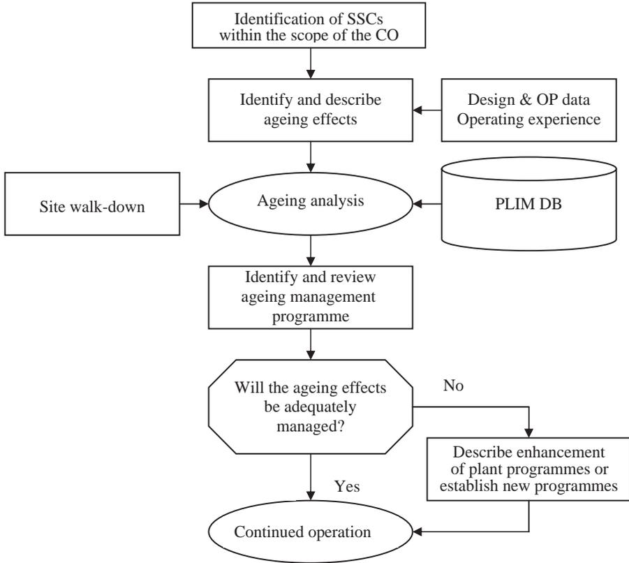
FIG. 5. Ageing evaluation process in a PSR.
