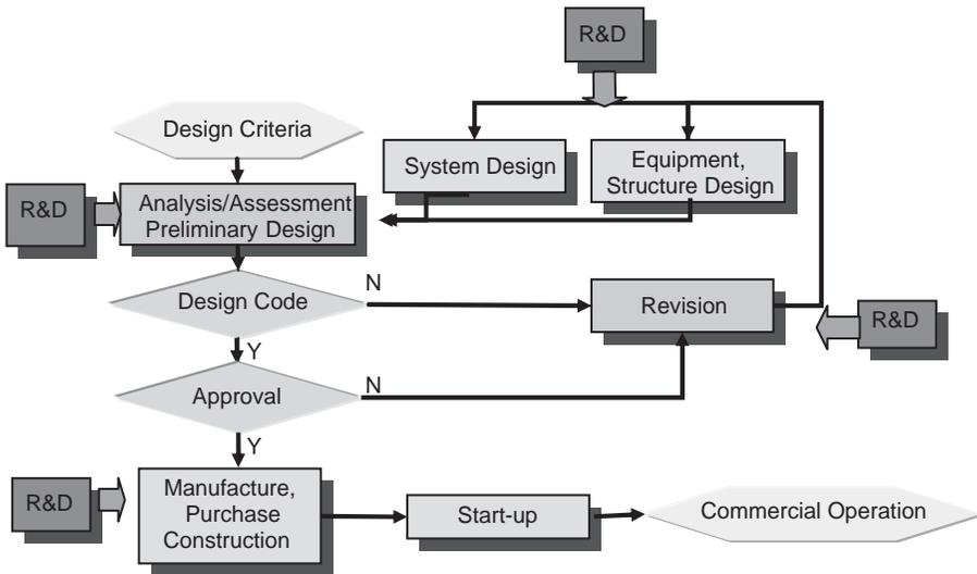
FIG. 8. Process of using the results of R&D for enhancing safety.
