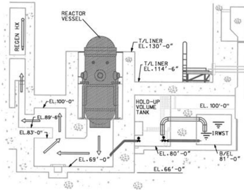
FIG. 4. APRI400 reactor cavity.
