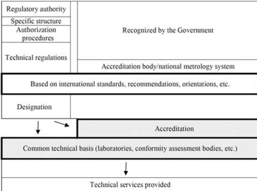
FIG. 3. Regulatory regime using a common technical basis provided by national systems (adapted from [2]).
