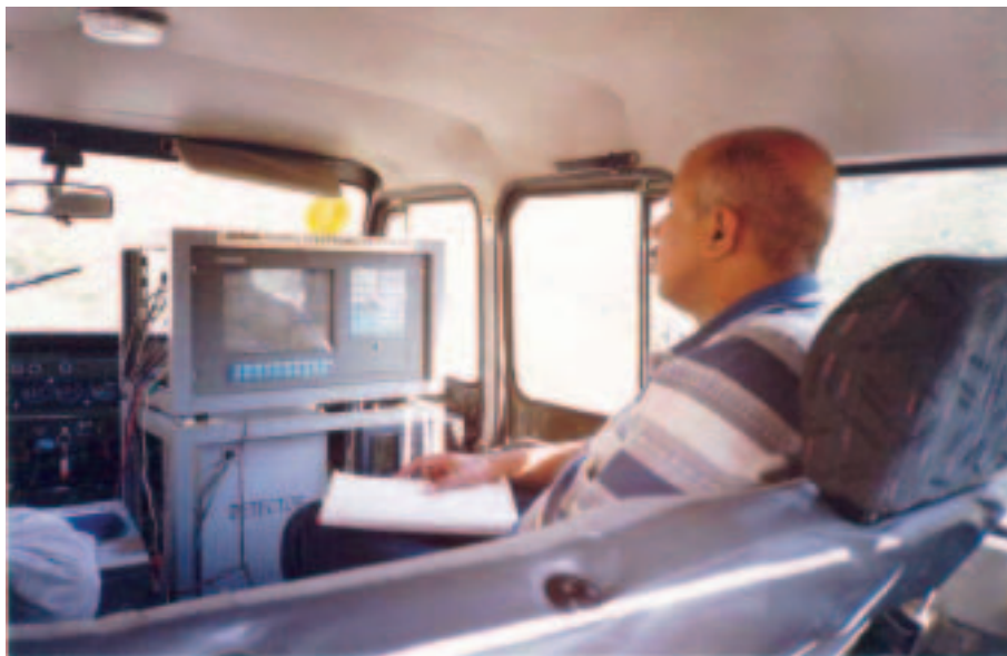
FIG. 4. AGSS installed in the NRSS jeep during the source search operation.
