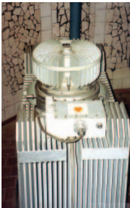
FIG. 2(a). A strontium-90 thermogenerator from the former Soviet Union.
