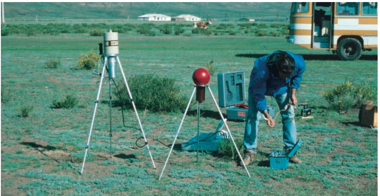
FIG. 10. In situ gamma spectrometric and exposure dose rate measurements during the IAEA mission in July 1994.
