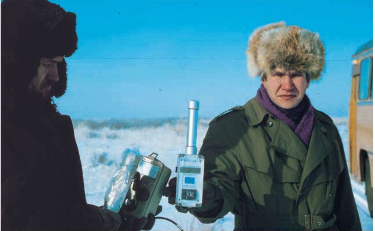
FIG. 9. Gamma dose rate measurements at Lake Balapan during the IAEA mission in November 1993.
