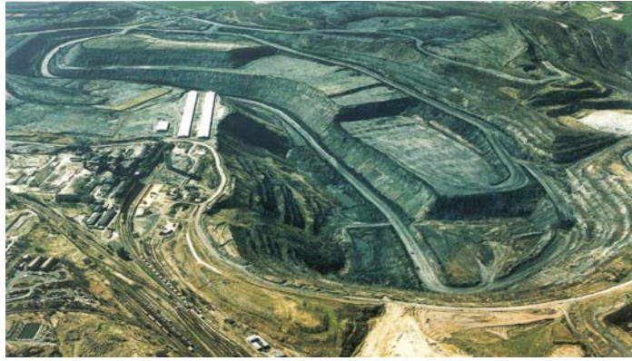
FIG.6. Lichtenberg open pit partially backfilled, with disposal areas for material A (foreground, bottom of the pit), B, and C (background), and ongoing relocation of the Nordhalde (background right). Situation in 1999.
