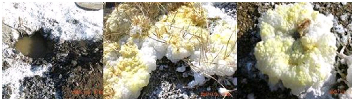
FIG.3. Uranium salt precipitates on the bottom of the creek that receives the seepage from the low grade ore pile, the Taboshar “Hill”.
