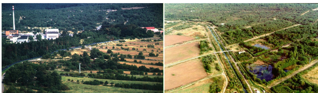
FIG.3. Wellfields with pattern 20x50 m (left) and well lines at spacing of 100 m (right).
