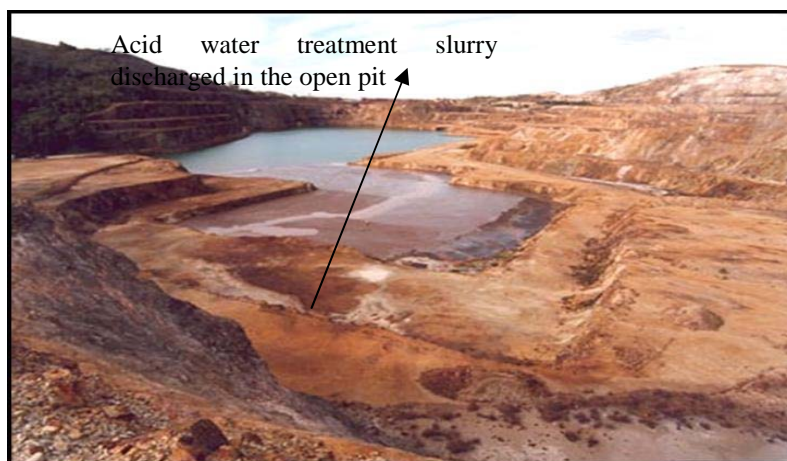
FIG. 2. Open pit with the deposition of the slurry from the acid water treatment in detail.
