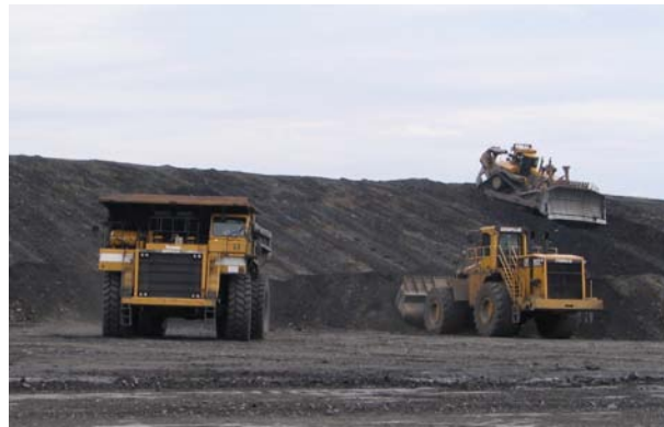
FIG.5. Waste rock excavation. Technological sequence with Dozer D11R, Front-end loader CAT 992H and haul truck CAT 785. Relocation of Halde Paitzdorf, June 2006.
