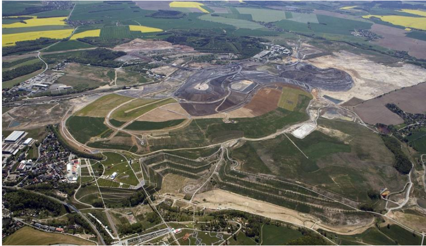
FIG.10. Reclaimed Ronneburg mine site, with the almost completely backfilled former Lichtenberg open pit, partially covered and re-vegetated (May 2007). Footprint areas of the Nordhalde (foreground, re-vegetated), Absetzerhalde (right), and Halde Reust (background).
