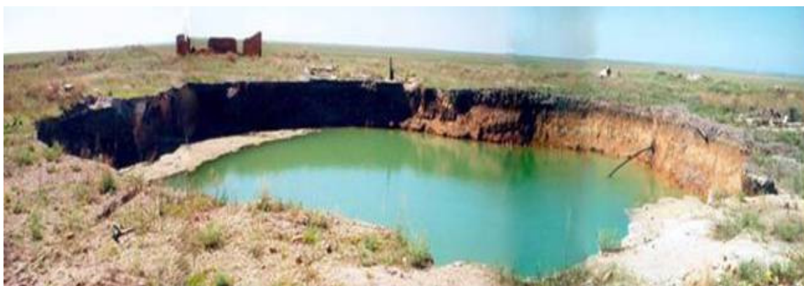
FIG. 9. Kamyshovoye deposit in n. Kazakhstan. Mine cave-in in the vicinity of the shaft No. 5 of the mine No. 3, mine administration No. 4.
