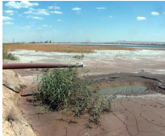
FIG.1. Discharging the tailings from gold processing over the “old” uranium tailings into the tailings impoundment at Navoi, Uzbekistan.
