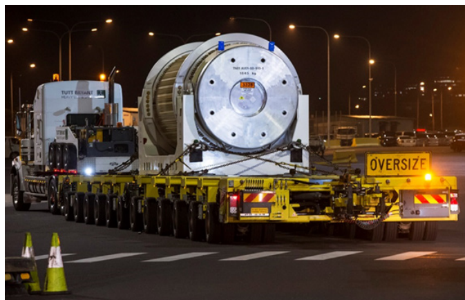
FIG. I-5. TN 81 cask loaded and ready for transport (courtesy of ANSTO).
