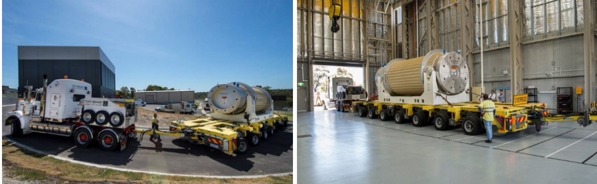
FIG. I-7. TN 81 cask moved to interim waste store at ANSTO (courtesy of ANSTO).
