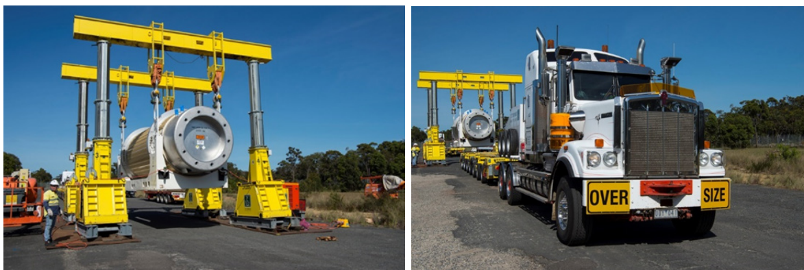
FIG. I-6. TN 81 cask transfer from external to internal transport for interim storage at the ANSTO site (courtesy of ANSTO).
