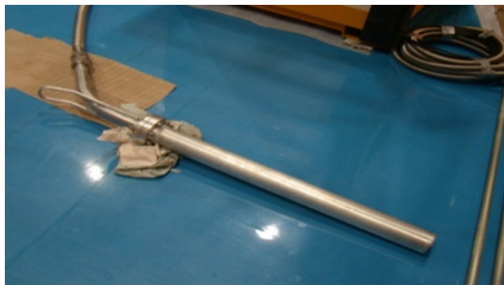
FIG. I-14. Watertight fuel handler used to remove fuel between storage rack and core (courtesy of Malaysian Nuclear Agency).
