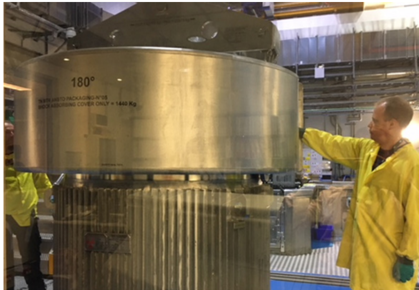
FIG. 8. TN MTR spent fuel transport cask (courtesy of ANSTO).
