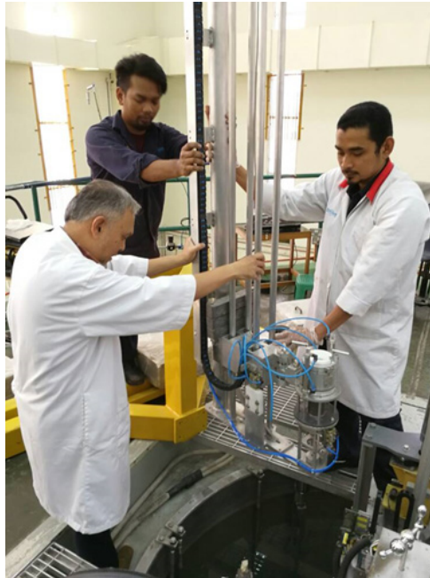
FIG. I–15. Researchers lowering the underwater test rig into the reactor pool (courtesy of Malaysian Nuclear Agency).
