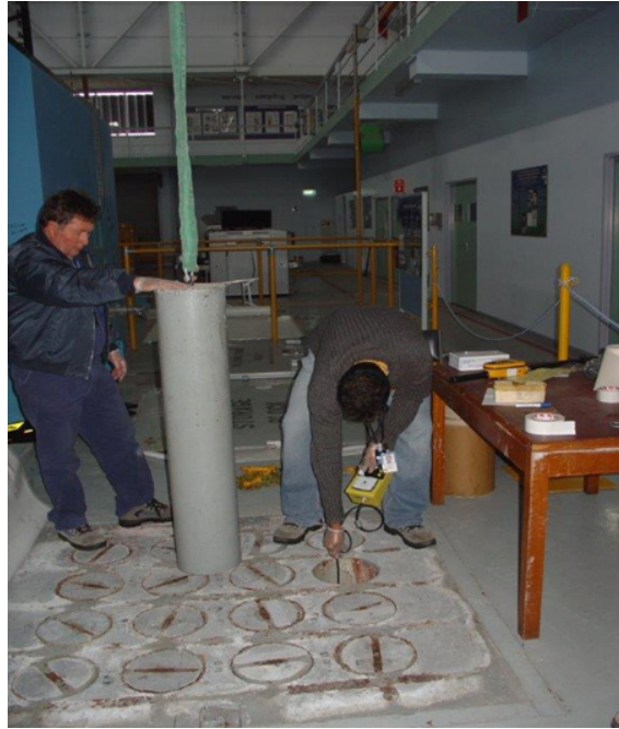
FIG. 10. Moata spent fuel holes inspection (courtesy of ANSTO).
