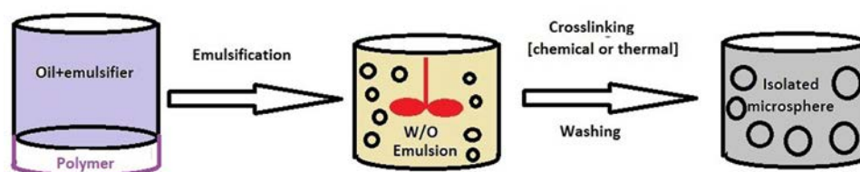
FIG. 21. Microparticle preparation using the emulsion technique. Courtesy of A. Dash and A. Jalilian.
