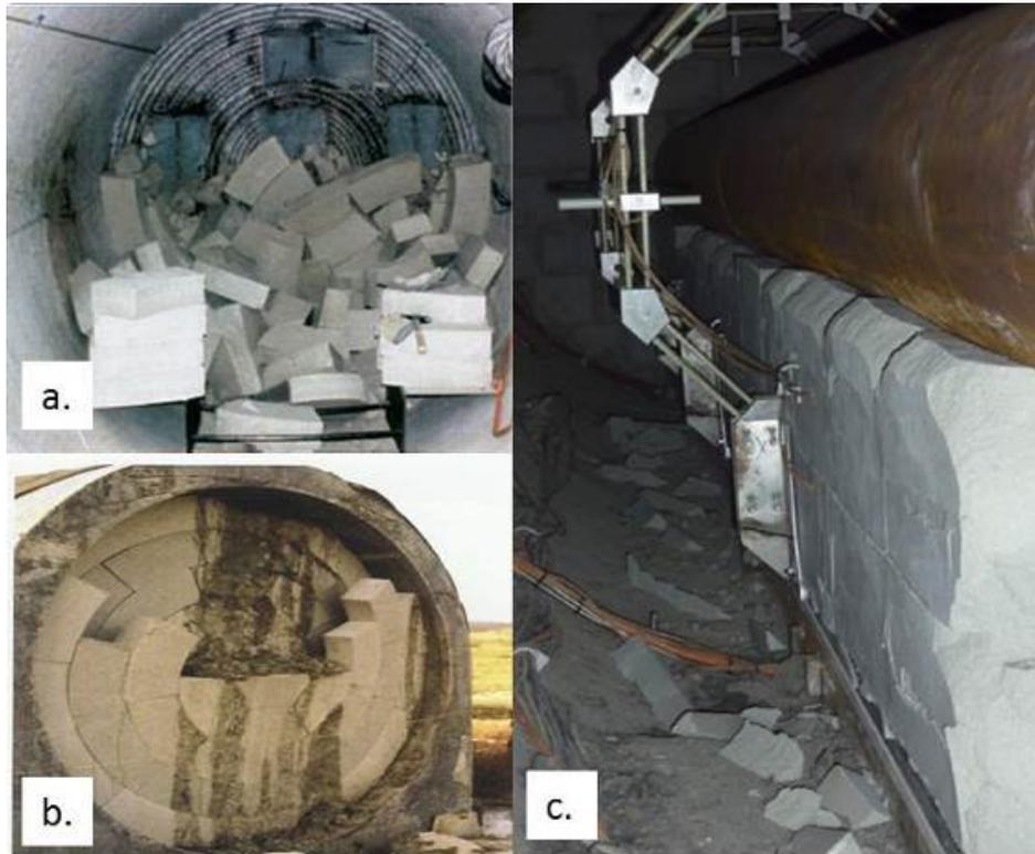
FIG. 9. Examples showing the difficulties in the handling and emplacement of highly compacted bentonite blocks underground.
