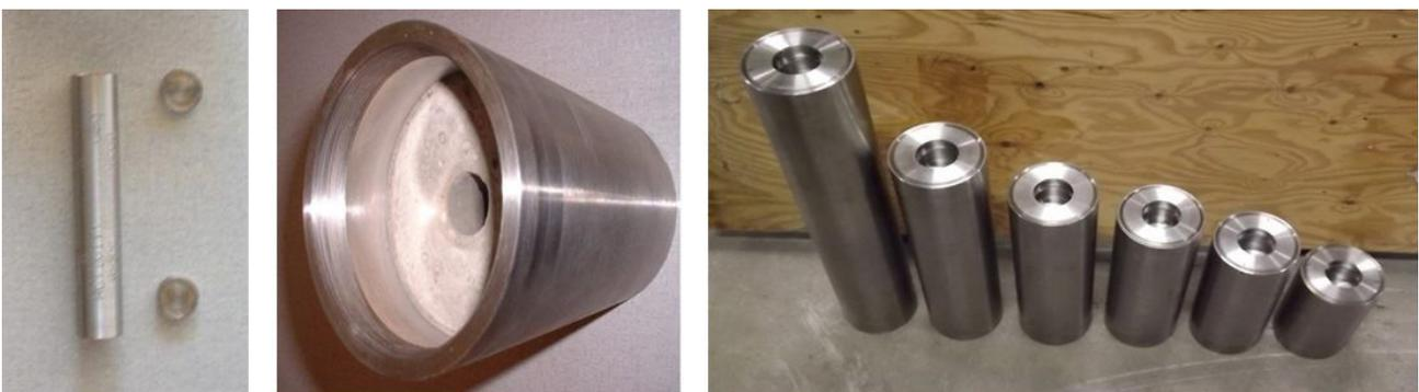
FIG. 51. DSRS standardized waste package design. Stainless steel capsule (left) with a 7 cm diameter; interior cement buffer (centre) in the various sizes available (right).
