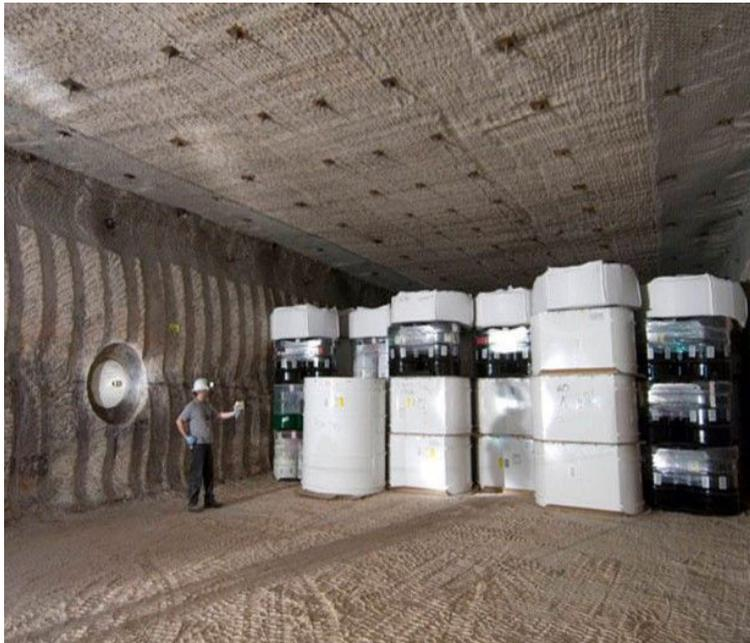
FIG. 43. Disposal operations at the WIPP, USA, showing both remote and contact handled waste packages (courtesy of the United States Department of Energy).
