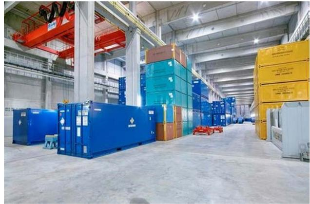
FIG. 50. Waste containers (cylindrical and cubic) meeting the WAC for disposal at Konrad, Germany (courtesy of Gesellschaft für Nuklear Service (left) and Bundesgesellschaft für Endlagerung mbH (right)).
