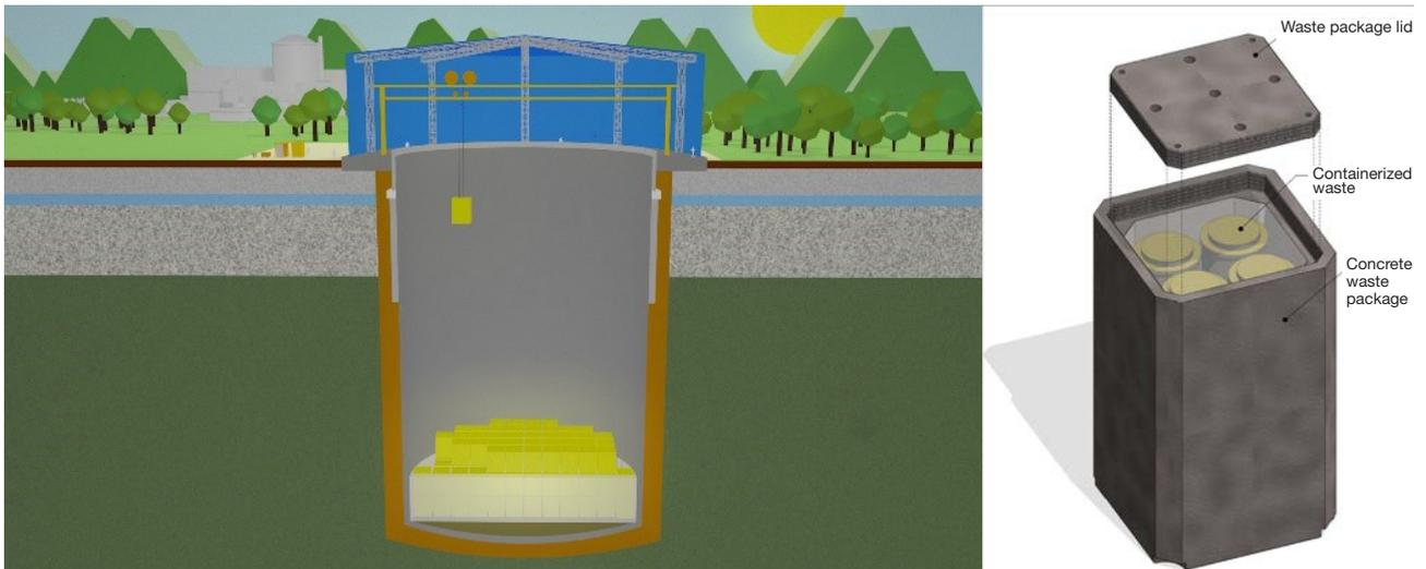
FIG. 28. Vrblina repository, Slovenia: vertical cross-section of the silo during the operational period and an illustration of a waste container (courtesy of the Agency for Radioactive Waste, Slovenia).
