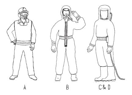
Industrial suits of different types provide varying degrees of protection.
