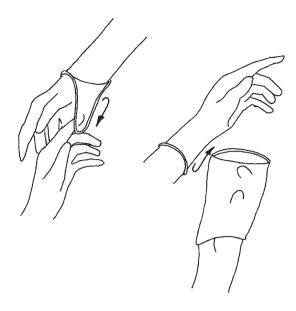
Procedure for removing contaminated lightweight gloves.
