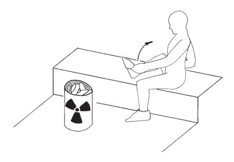
Procedure for removing contaminated footwear.
