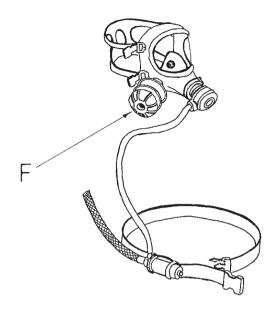
Full face mask with compressed air line and auxiliary filter.
