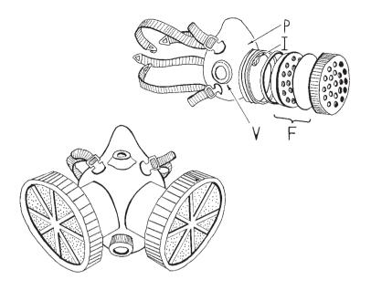
Half mask respirators with single and multiple cartridges.
